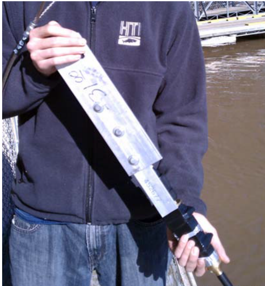
Figure 2-8 Representative Photograph of a “Dock” Mount
