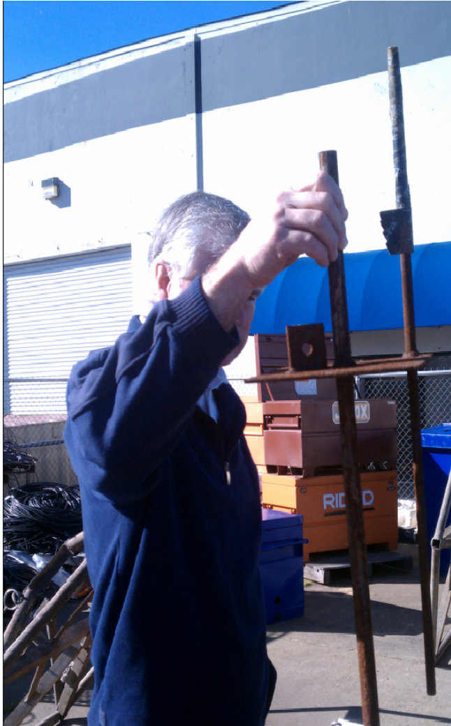
Figure 12. Example of the “Pound In” mount used for deployment of hydrophones H2, H4, H11, H13, H14, H15, and H19 at the GSNPB, 2011.
