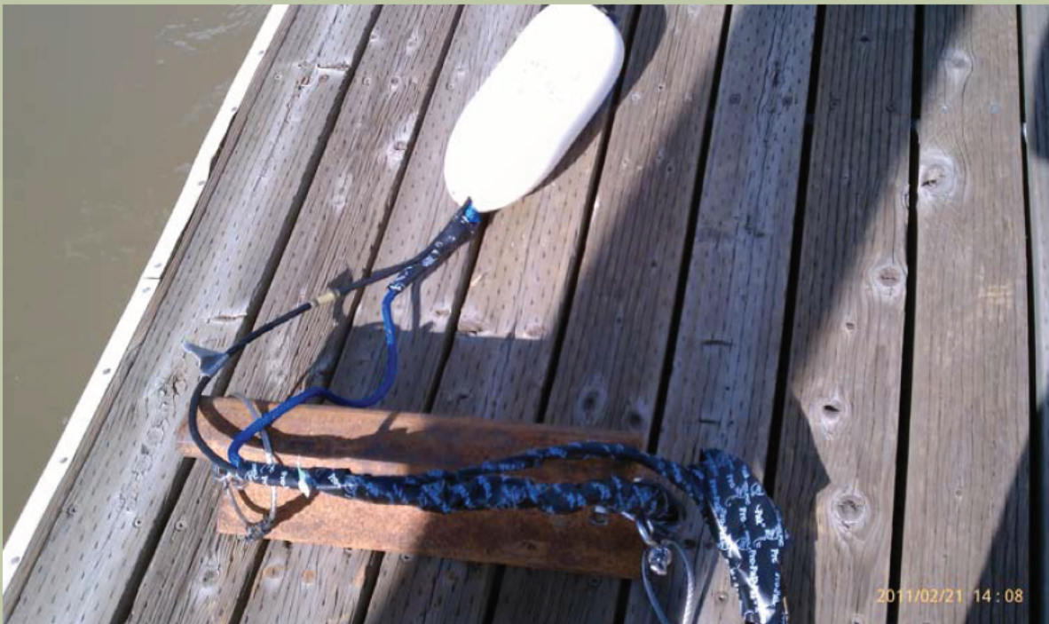
Figure 6-28 Example Hydrophone Mount used for Head of Old River (HOR) Deployments during the 2011 VAMP
