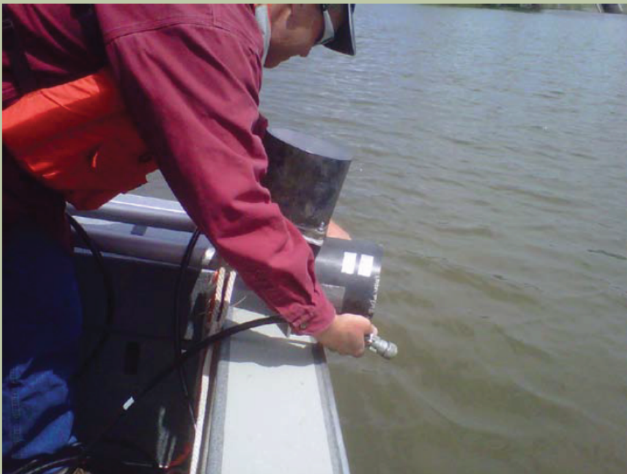
Figure 6-30 Picture of 200khz Transducers as they are being Lowered over the Side of the Boat for a Mobile Survey
