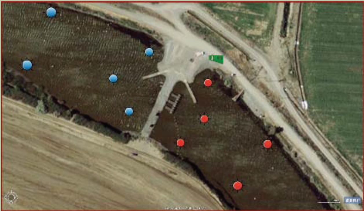
Figure 8-3 2D Acoustic Biotelemetry System Deployed at the Old River at Tracy Barrier in 2010. (The Red Circles Indicate the Location of the Hydrophones Located Upstream of the Old River at Tracy Barrier and the Blue Circles Indicate the Locations of the Hydrophones Located Downstream of the Barrier)
