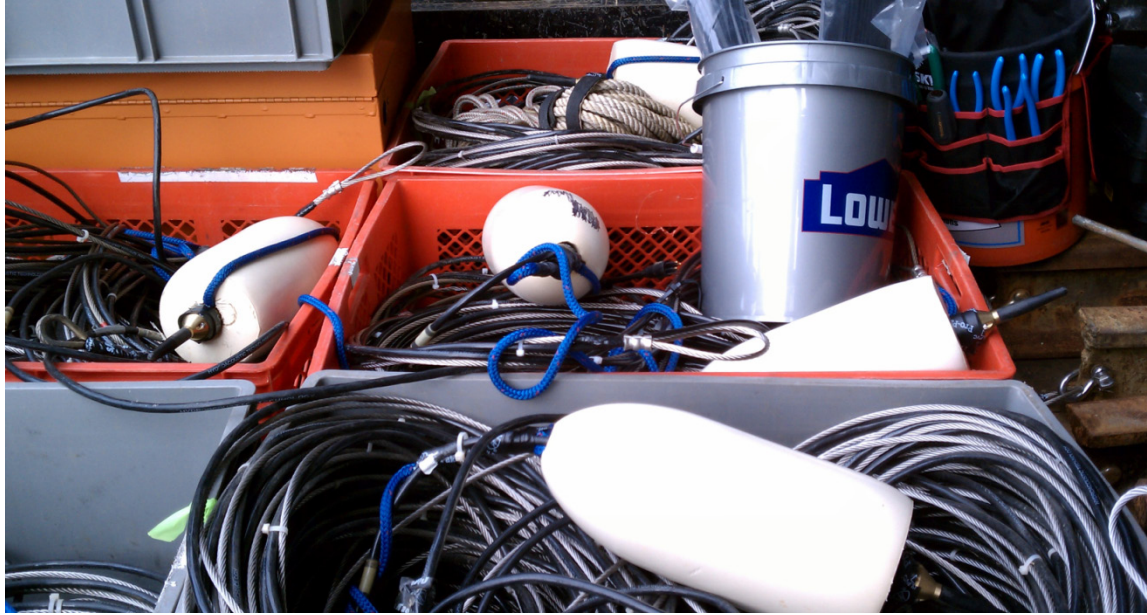
Figure 11. Hydrophone cables ready for deployment.
