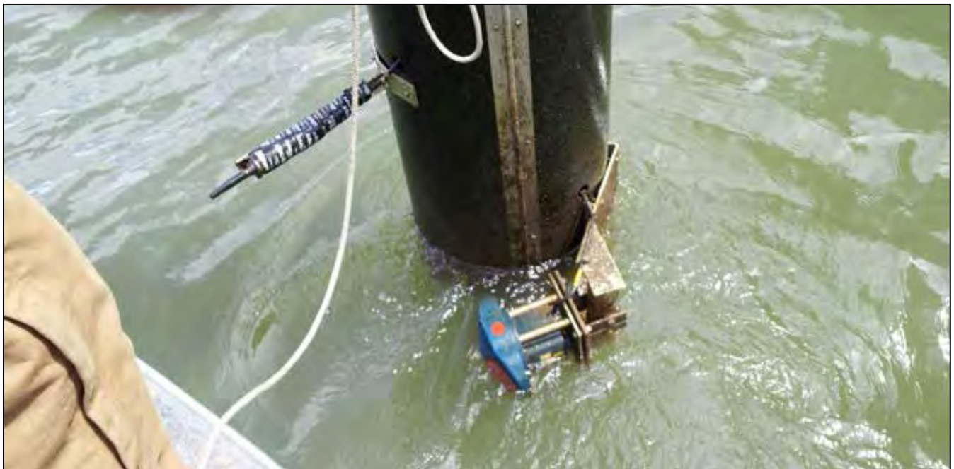
Figure 2-11 Typical Floating Pile Mount
