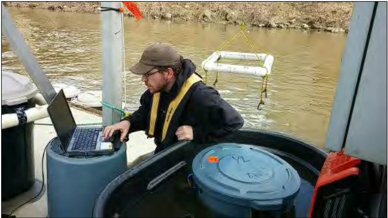
Figure 2-15 Confirming Operation of Acoustic Transmitters before Release
