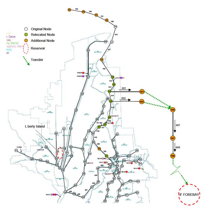
DSM2 Grid Modifications for North Delta Intakes in Alternatives 4, 7 and 8
