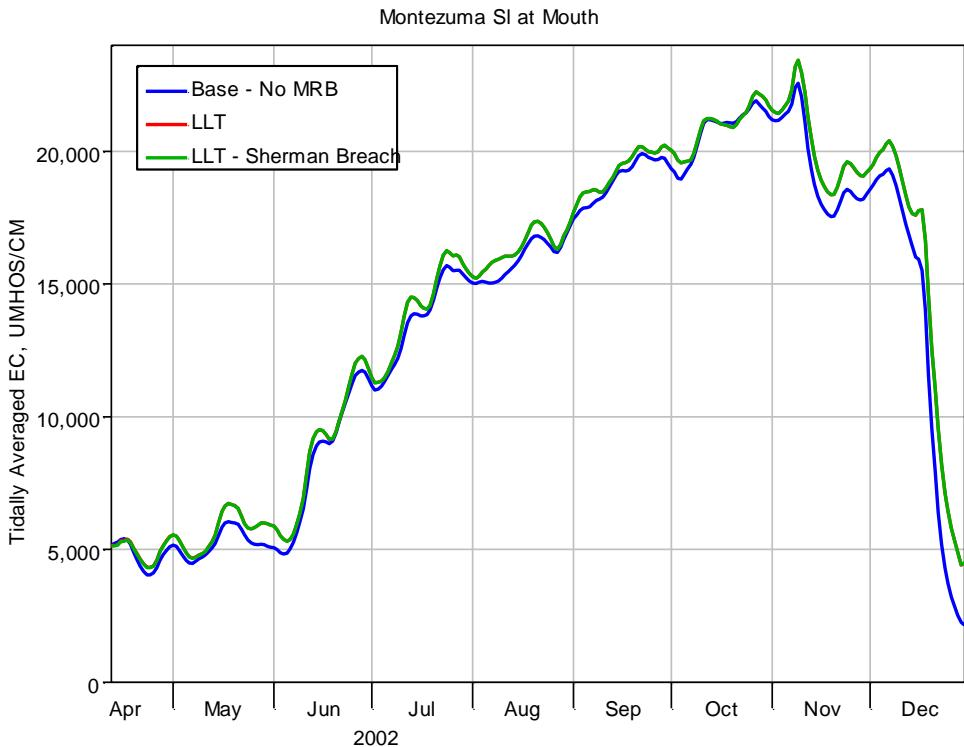
**Figure 5-166** Tidally averaged EC at Montezuma Sl at Mouth for Base-No MRB, LLT and LLT-Sherman Breach.
