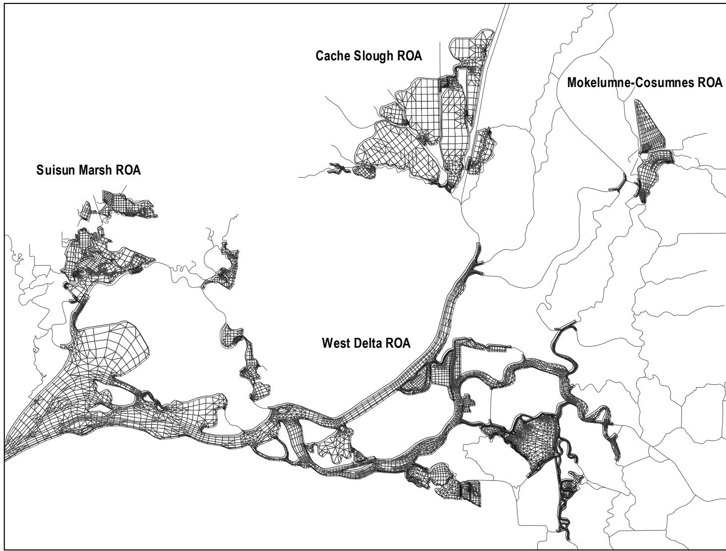
Figure 2-2 RMA Early Long-Term model finite element mesh.
