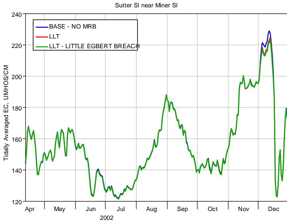
**Figure 5-128** Tidally averaged EC in Sutter Slough for Base-No MRB, LLT and LLT-Little Egbert Breach.
