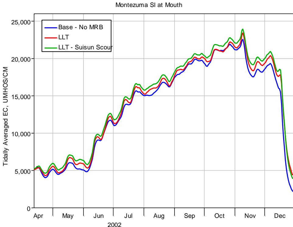
**Figure 5-97** Tidally averaged EC at Montezuma Slough at Mouth for Base-No MRB, LLT and LLT-Suisun Scour.
