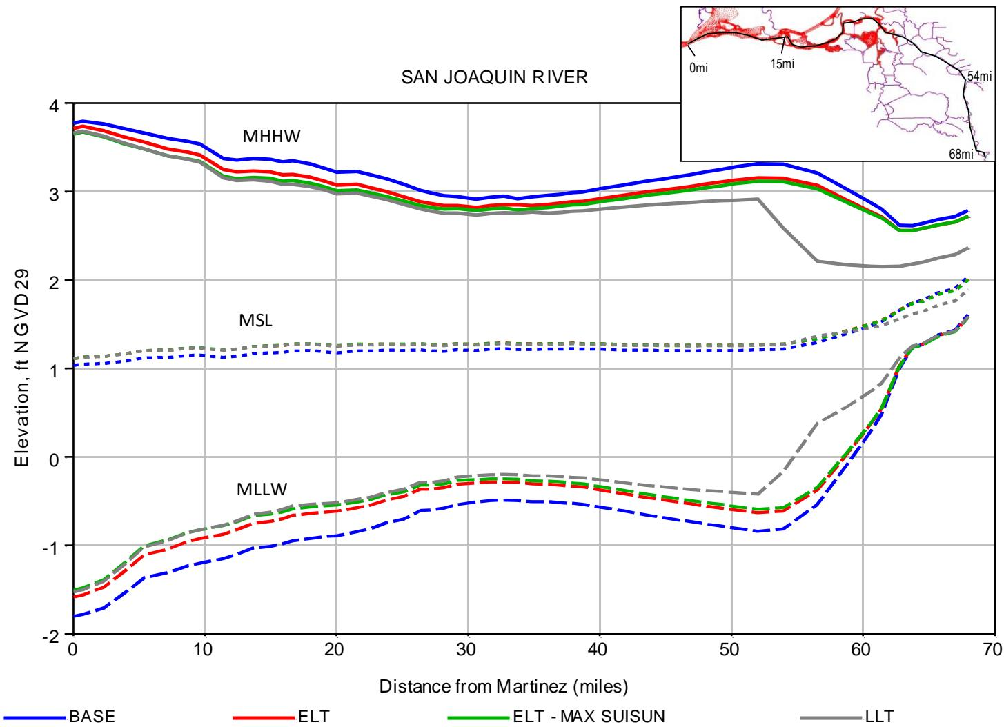
Figure 4-8 Profiles of July 2002 MHHW, MSL and MLLW along the San Joaquin River for the Base – No SMSCG (Base), ELT and ELT - Max Suisun simulations.
