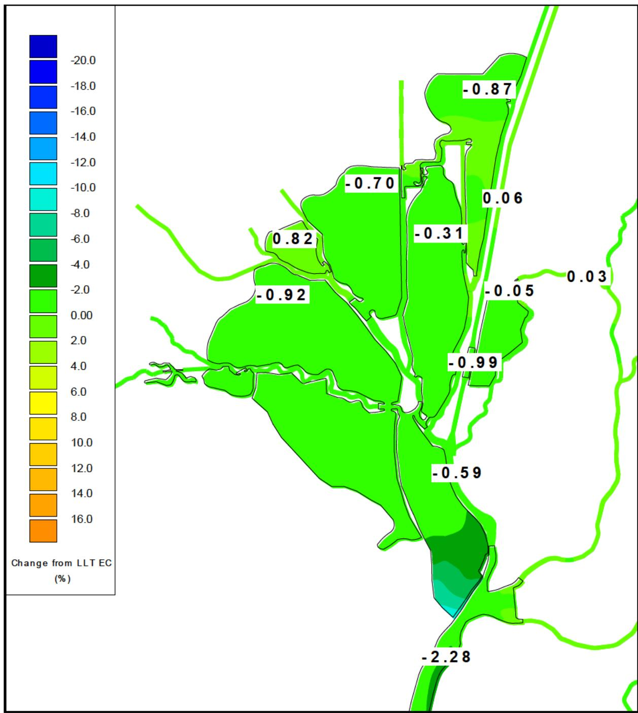
Figure 5-149 Contour plots of LLT – Little Egbert change from LLT tidally averaged EC in the Cache Slough ROA on September 24, 2002.
