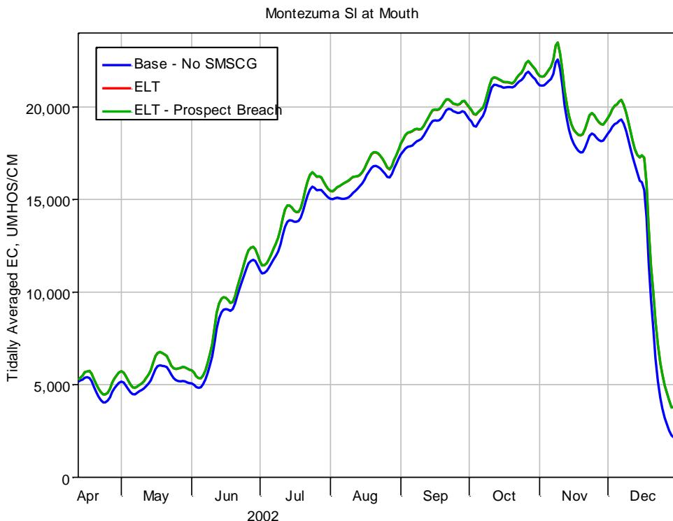
**Figure 5-121** Tidally averaged EC at Montezuma Slough at Mouth for Base-No SMSCG, ELT and ELT-Prospect Breach.
