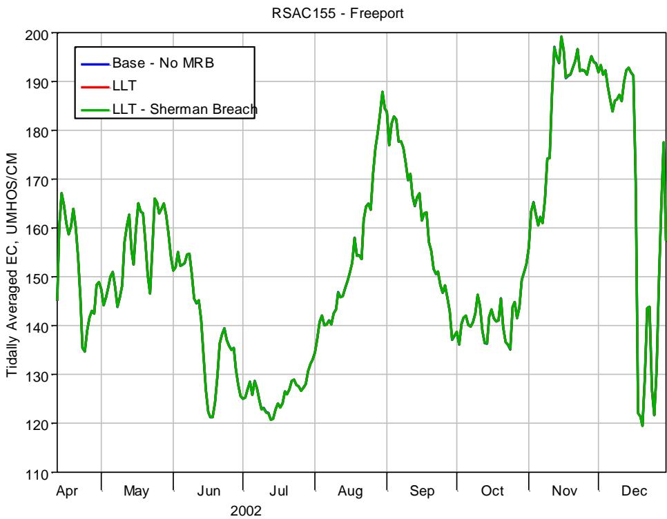
**Figure 5-151** Tidally averaged EC at RSAC155 for Base-No MRB, LLT and LLT-Sherman Breach.
