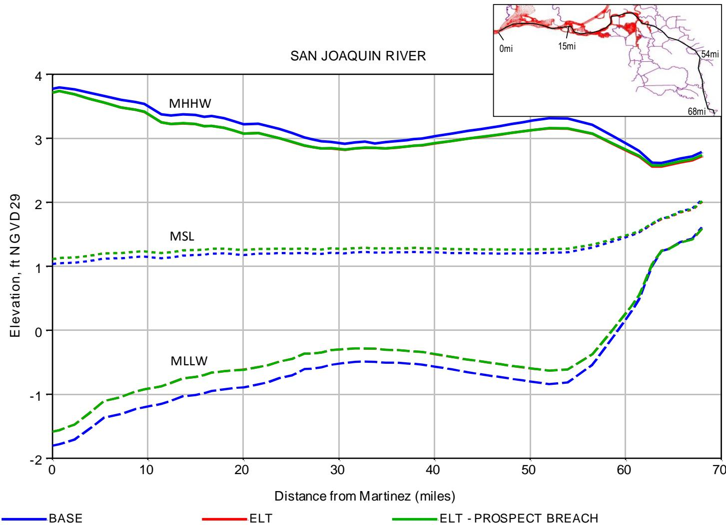
Figure 4-99 Profiles of July 2002 MHHW, MSL and MLLW along the San Joaquin River for the Base - No SMSCG (Base), ELT and ELT - Prospect Breach simulations.
