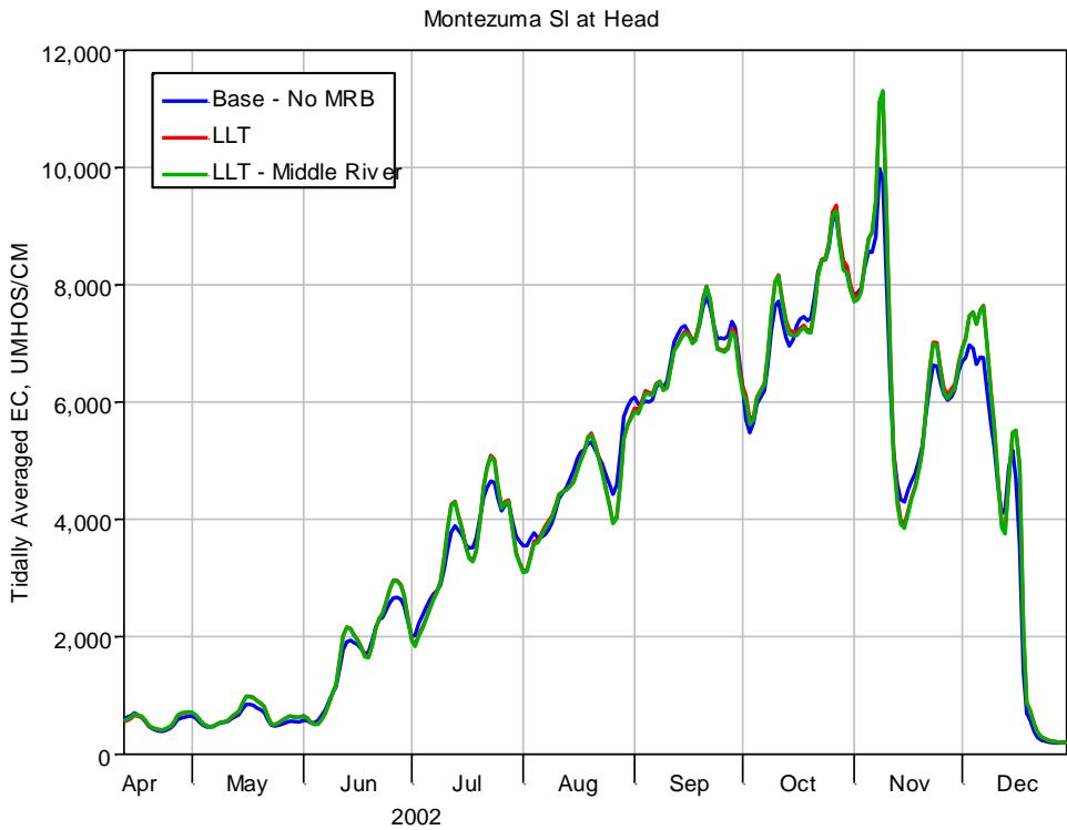
**Figure 5-71** Tidally averaged EC at Montezuma Slough at Head for Base-No MRB, LLT and LLT-Middle River.
