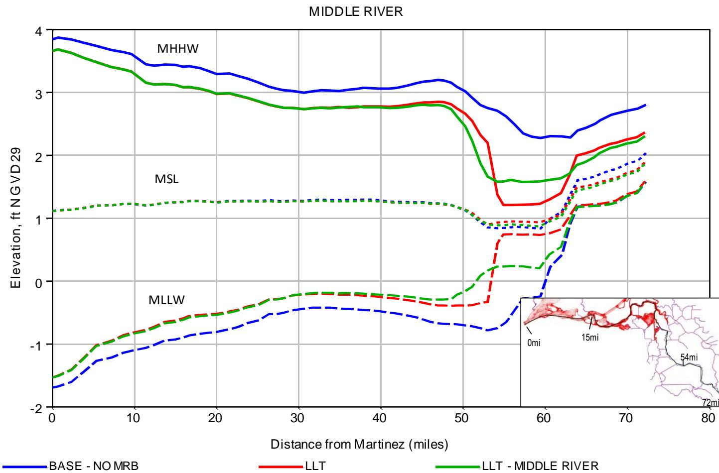
Figure 4-56 Profiles of July 2002 MHHW, MSL and MLLW along the Middle River for the Base - No MRB, LLT and LLT - Middle River simulations.
