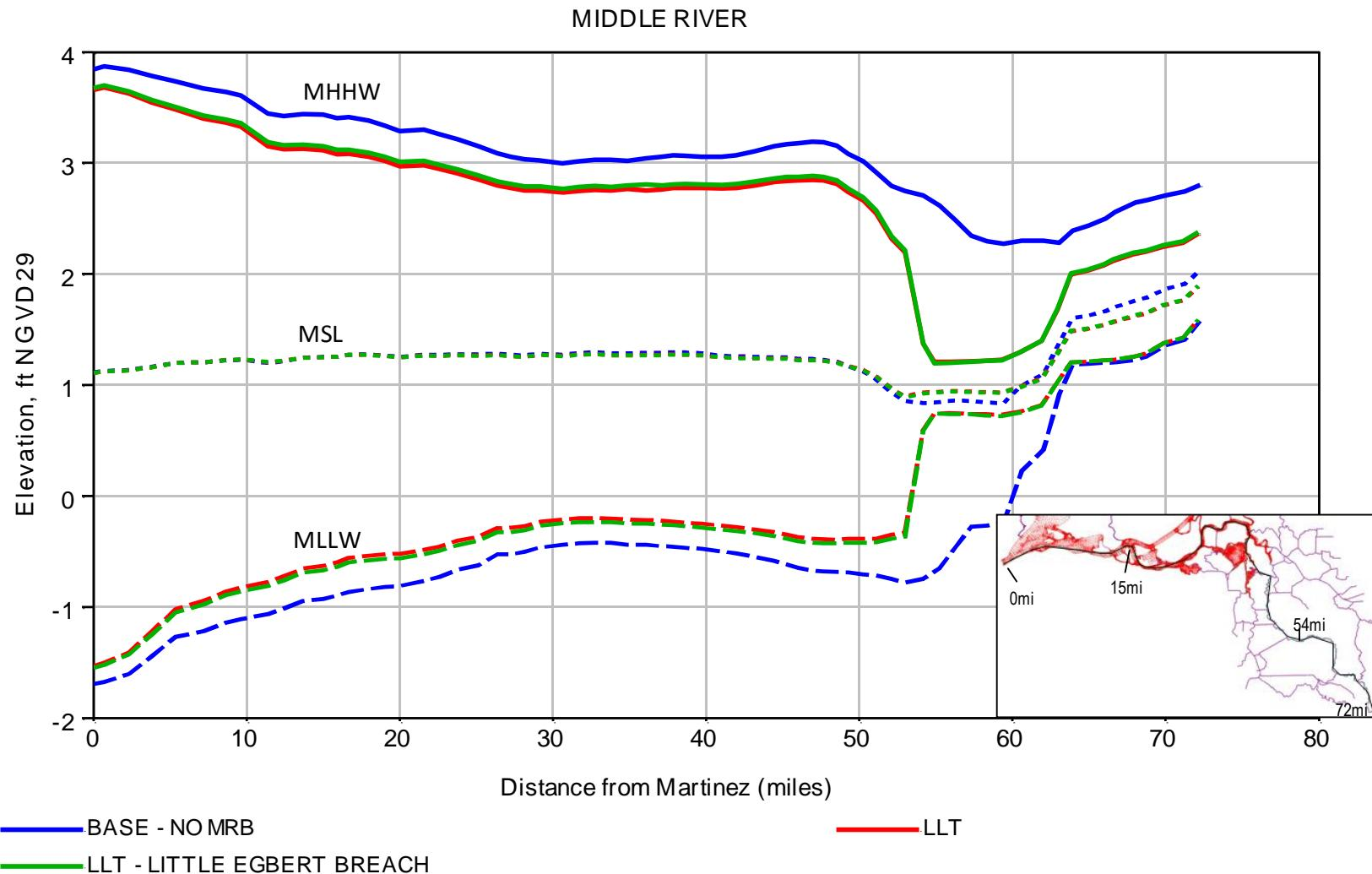
Figure 4-120 Profiles of July 2002 MHHW, MSL and MLLW along the Middle River for the Base - No MRB, LLT and LLT - Little Egbert Breach simulations.
