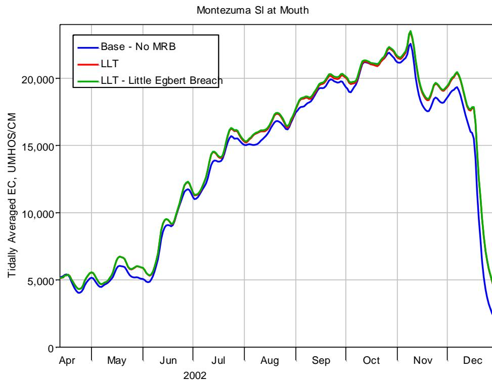
**Figure 5-145** Tidally averaged EC at Montezuma Sl at Mouth for Base-No MRB, LLT and LLT-Little Egbert Breach.
