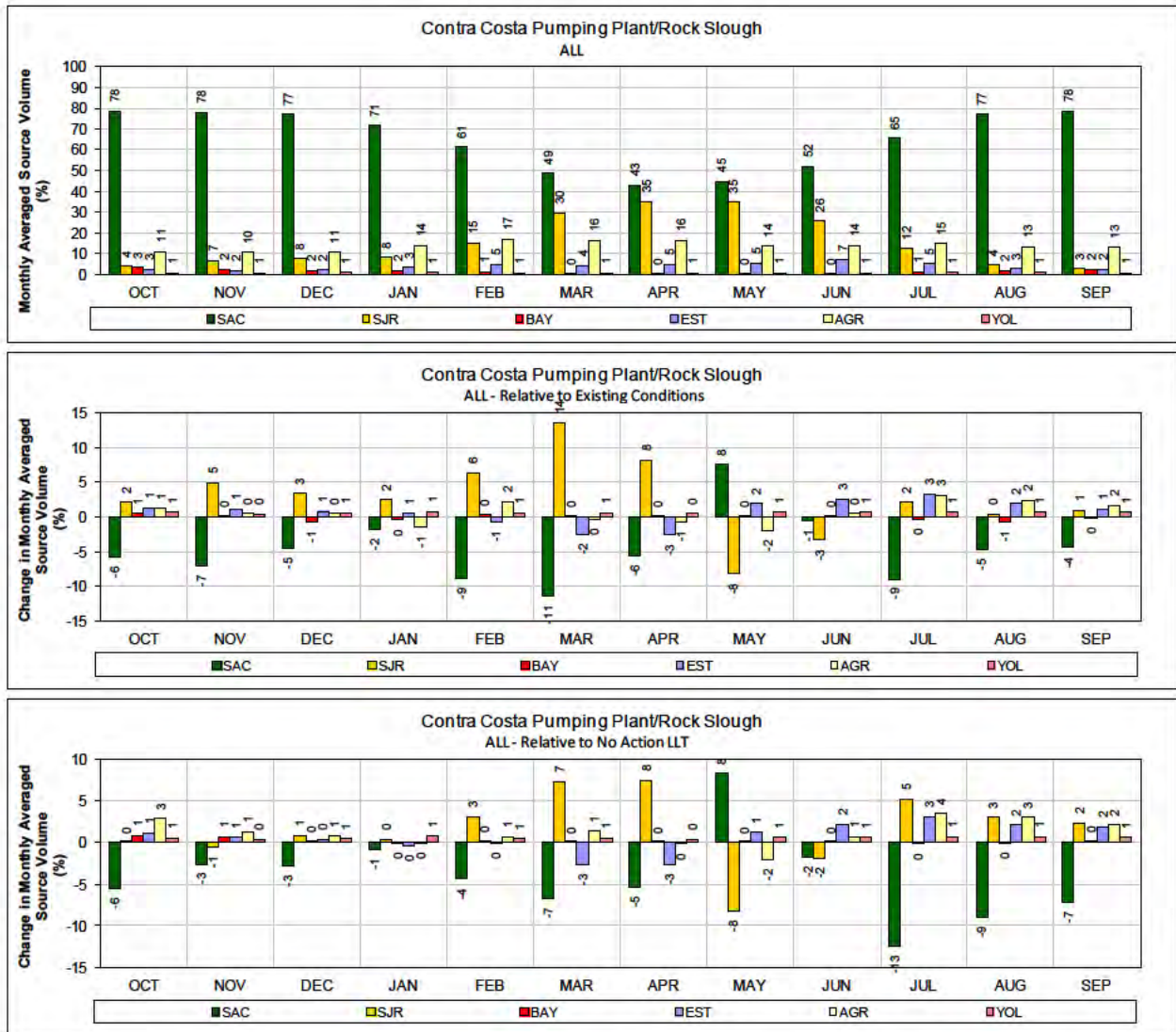
1 Figure 83. ALT 3 – Contra Costa Pumping Plant #1 for ALL years (1976-1991) 2 Monthly average source volume (top figure) and change in monthly average source volume relative to 3 Existing Conditions and No Action Alternative Late Long Term (bottom two figures).
