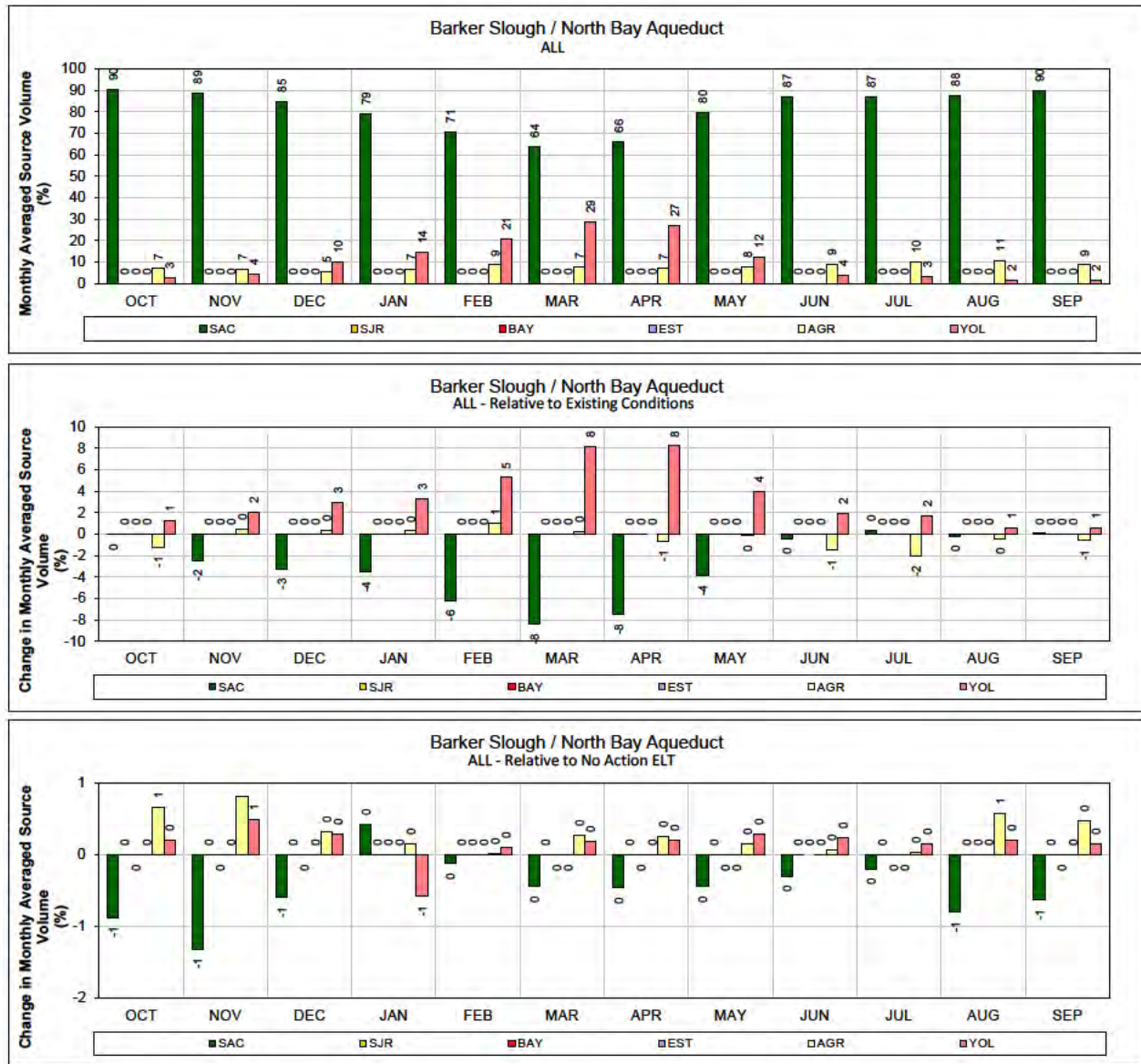
1 Figure 323. ALT 4A – North Bay Aqueduct at Barker Slough Pumping Plant for ALL years (1976-1991) 2 Monthly average source volume (top figure) and change in monthly average source volume relative to 3 Existing Conditions and No Action Alternative Early Long Term (bottom two figures).
