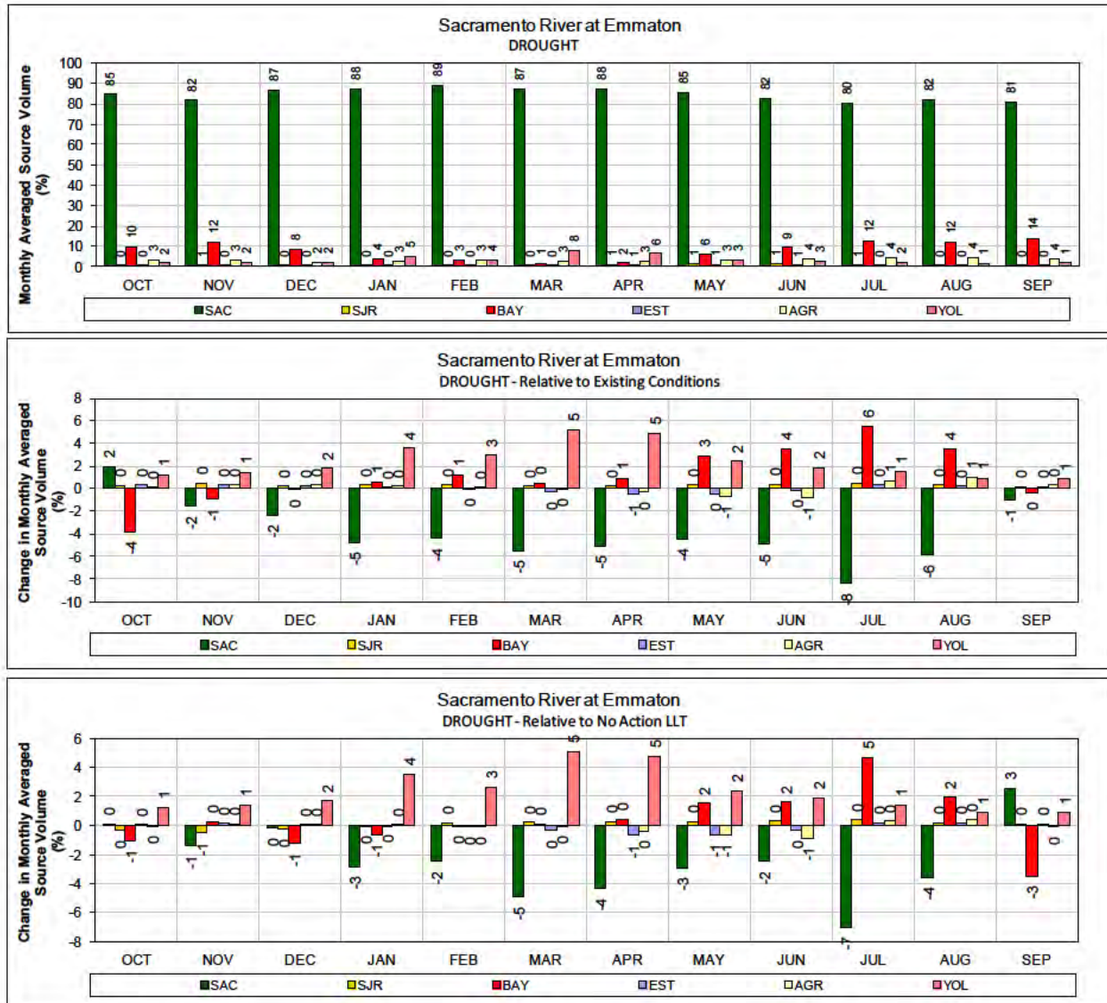
1 Figure 98. ALT 4 Scenario H1 – Sacramento River at Emmaton for DROUGHT years (1987-1991) 2 Monthly average source volume (top figure) and change in monthly average source volume relative to 3 Existing Conditions and No Action Alternative Late Long Term (bottom two figures).
