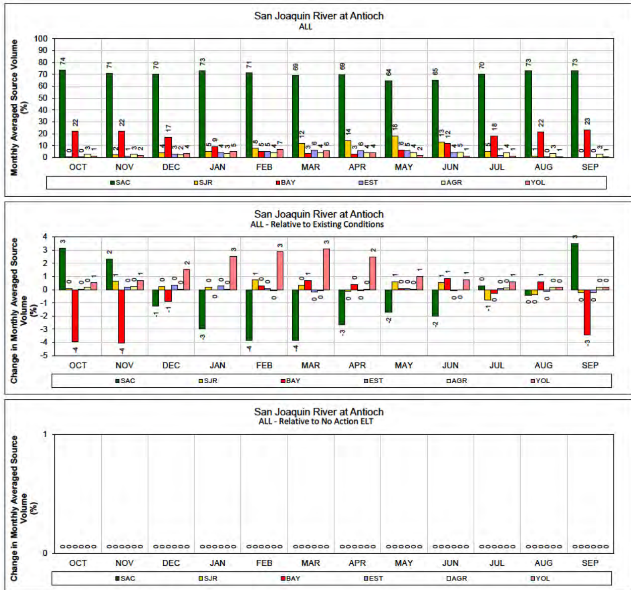
1 Figure 297. No Action ELT – San Joaquin River at Antioch for ALL years (1976-1991) 2 Monthly average source volume (top figure) and change in monthly average source volume relative to 3 Existing Conditions and No Action Alternative Early Long Term (bottom two figures).
