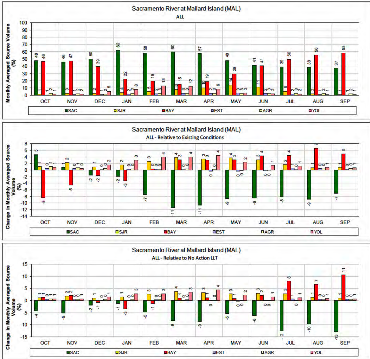
1 Figure 123. ALT 4 Scenario H2 – Sacramento River at Mallard Island for ALL years (1976-1991) 2 Monthly average source volume (top figure) and change in monthly average source volume relative to 3 Existing Conditions and No Action Alternative Late Long Term (bottom two figures).
