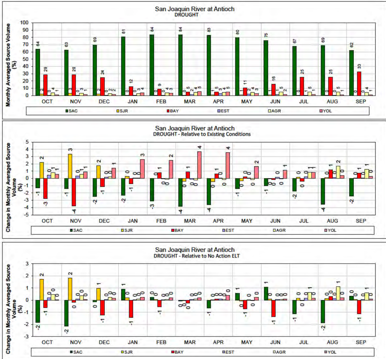
1 Figure 364. ALT 5A – San Joaquin River at Antioch for DROUGHT years (1987-1991) 2 Monthly average source volume (top figure) and change in monthly average source volume relative to Existing Conditions and No Action Alternative Early Long Term (bottom two figures). 3
