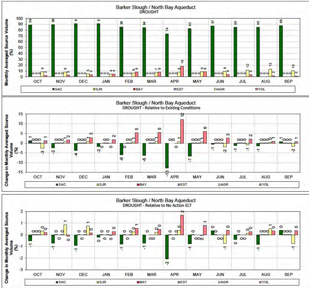
1 Figure 346. ALT 2D – North Bay Aqueduct at Barker Slough Pumping Plant for DROUGHT years 2 (1987-1991) 3 Monthly average source volume (top figure) and change in monthly average source volume relative to 4 Existing Conditions and No Action Alternative Early Long Term (bottom two figures).
