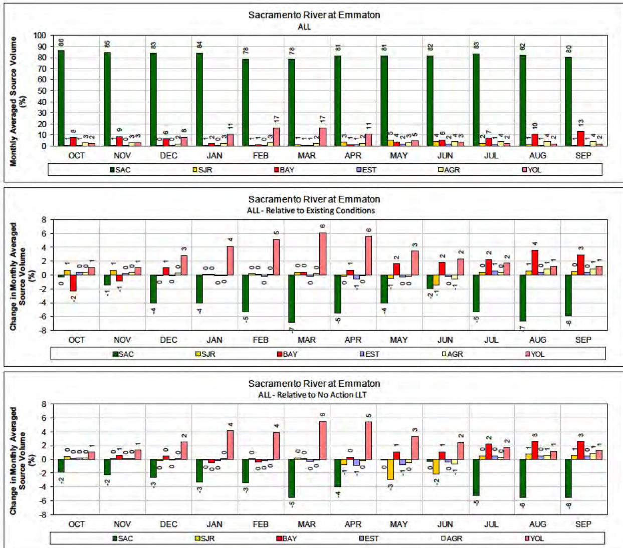
1 Figure 75. ALT 3 – Sacramento River at Emmaton for ALL years (1976-1991) 2 Monthly average source volume (top figure) and change in monthly average source volume relative to 3 Existing Conditions and No Action Alternative Late Long Term (bottom two figures).
