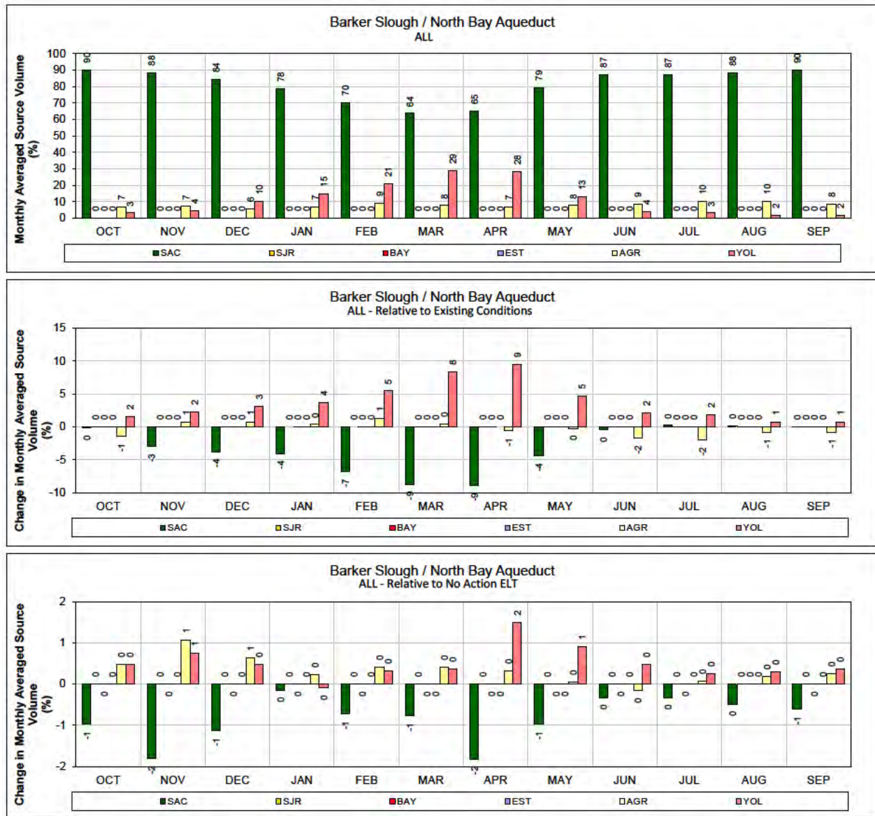
1 Figure 345. ALT 2D – North Bay Aqueduct at Barker Slough Pumping Plant for ALL years (1976-1991) 2 Monthly average source volume (top figure) and change in monthly average source volume relative to 3 Existing Conditions and No Action Alternative Early Long Term (bottom two figures).
