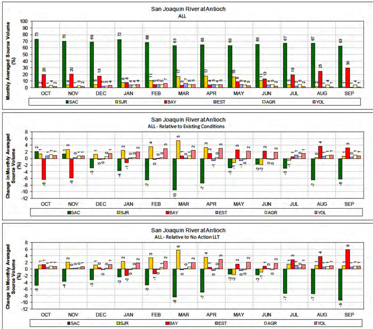
1 Figure 77. ALT 3 – San Joaquin River at Antioch for ALL years (1976-1991) 2 Monthly average source volume (top figure) and change in monthly average source volume relative to 3 Existing Conditions and No Action Alternative Late Long Term (bottom two figures).
