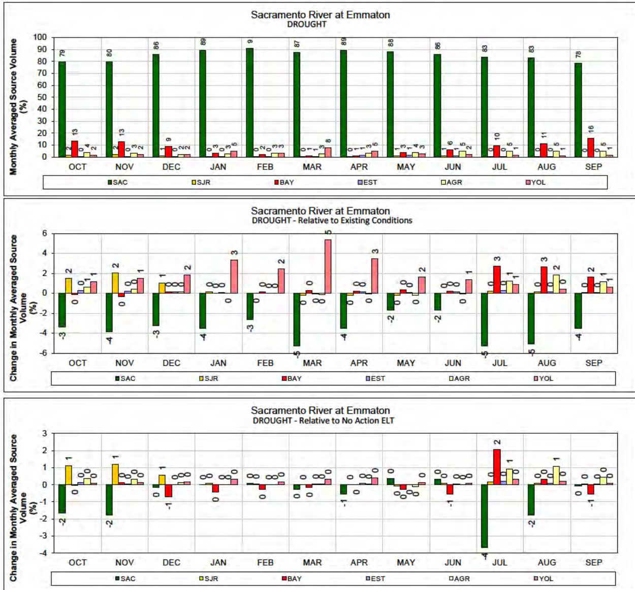
1 Figure 362. ALT 5A – Sacramento River at Emmaton for DROUGHT years (1987-1991) 2 Monthly average source volume (top figure) and change in monthly average source volume relative to 3 Existing Conditions and No Action Alternative Early Long Term (bottom two figures).
