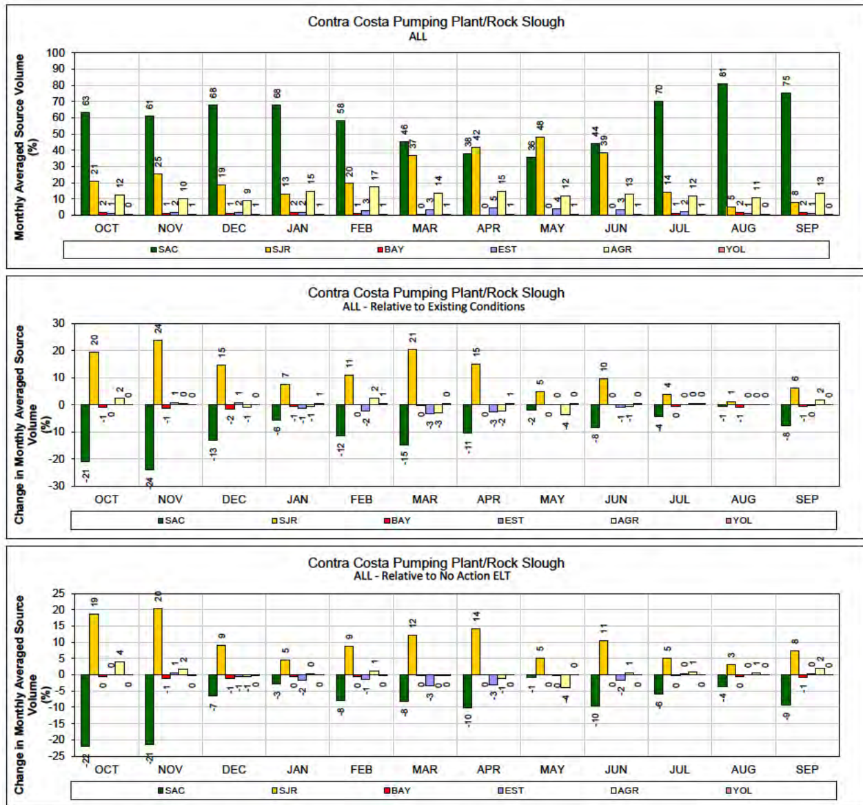
1 Figure 347. ALT 2D – Contra Costa Pumping Plant #1 for ALL years (1976-1991) 2 Monthly average source volume (top figure) and change in monthly average source volume relative to 3 Existing Conditions and No Action Alternative Early Long Term (bottom two figures).
