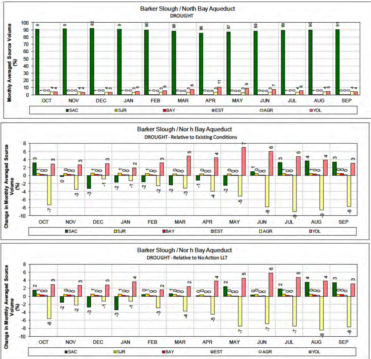
1 Figure 214. ALT 6 – North Bay Aqueduct at Barker Slough Pumping Plant for DROUGHT years 2 (1987-1991) 3 Monthly average source volume (top figure) and change in monthly average source volume relative to 4 Existing Conditions and No Action Alternative Late Long Term (bottom two figures).
