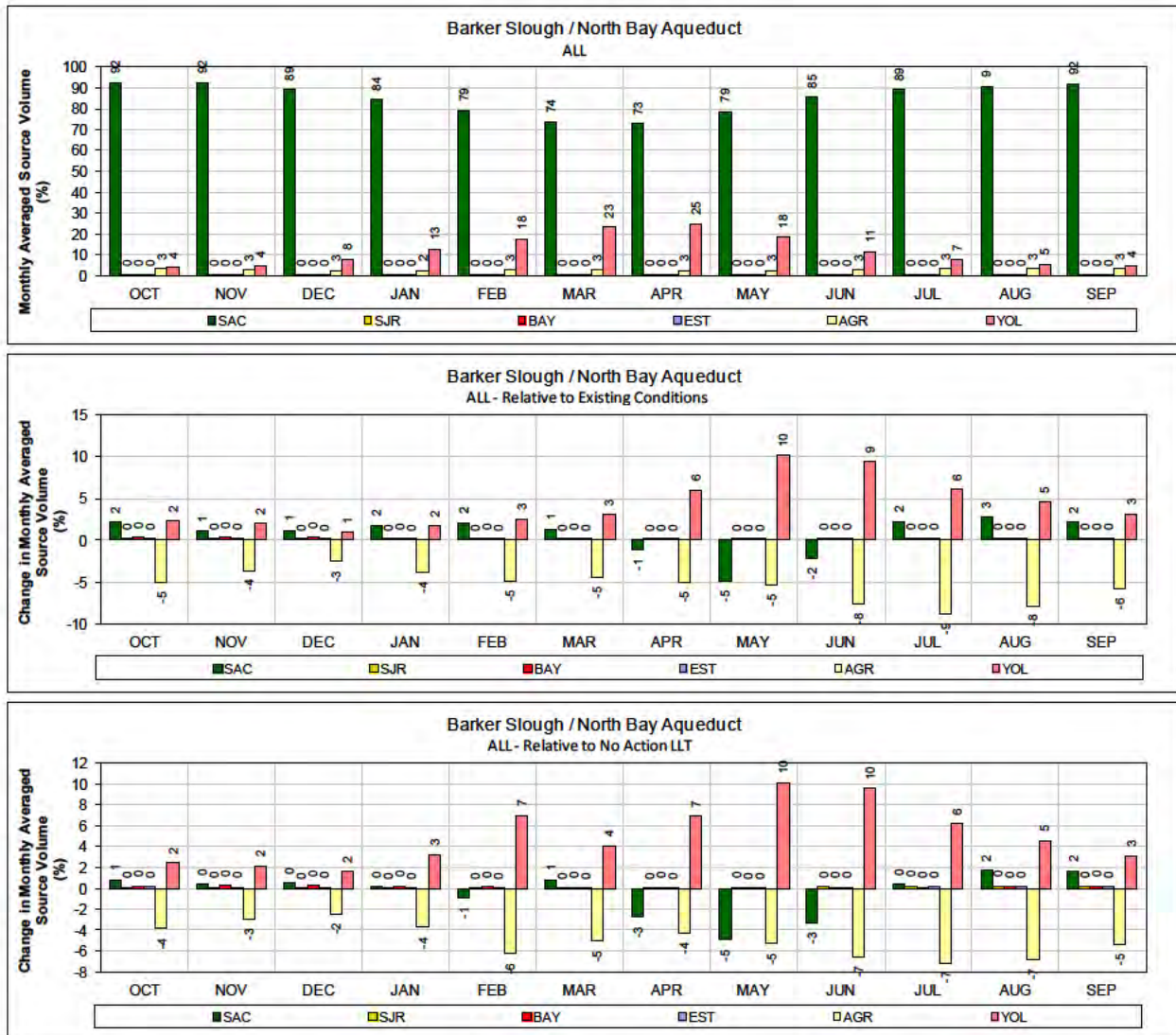
1 Figure 81. ALT 3 – North Bay Aqueduct at Barker Slough Pumping Plant for ALL years (1976-1991) 2 Monthly average source volume (top figure) and change in monthly average source volume relative to 3 Existing Conditions and No Action Alternative Late Long Term (bottom two figures).
