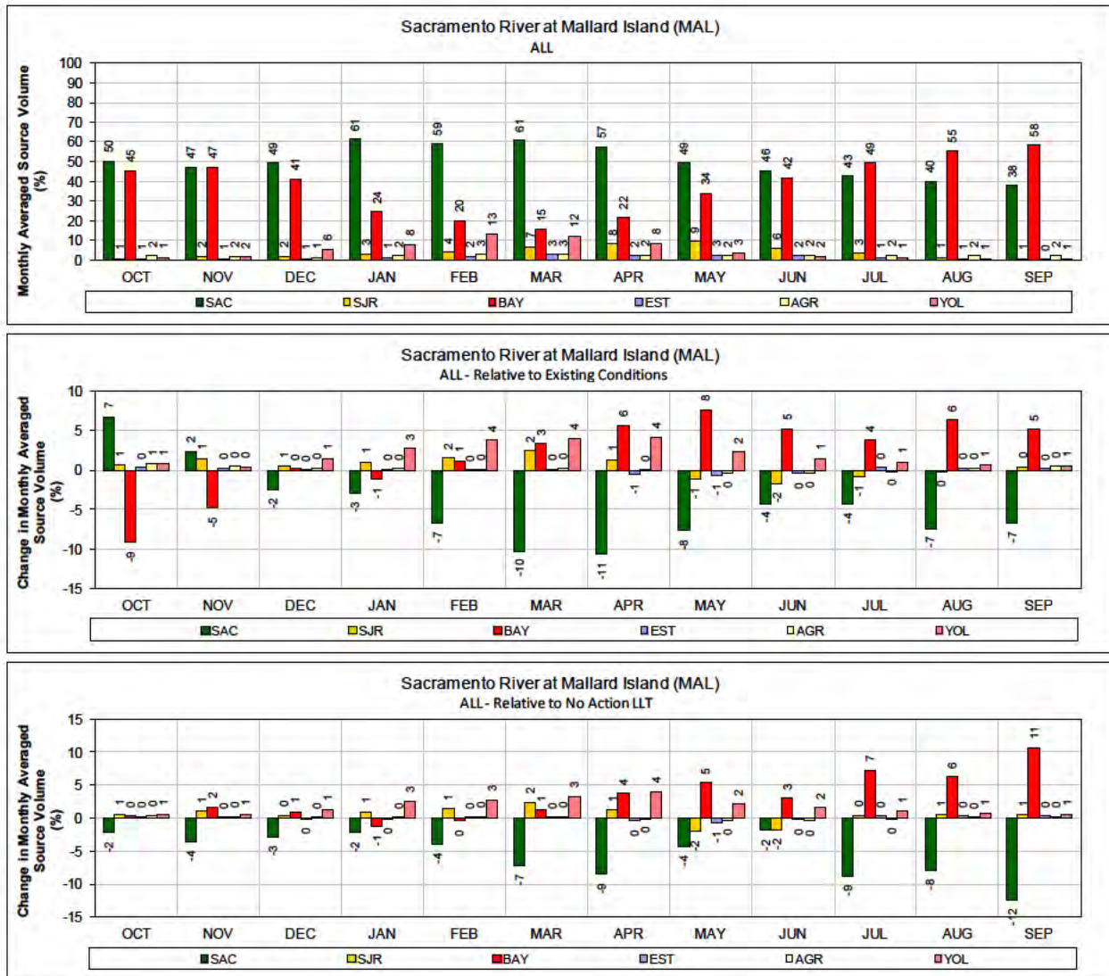
1 Figure 79. ALT 3 – Sacramento River at Mallard Island for ALL years (1976-1991) 2 Monthly average source volume (top figure) and change in monthly average source volume relative to 3 Existing Conditions and No Action Alternative Late Long Term (bottom two figures).
