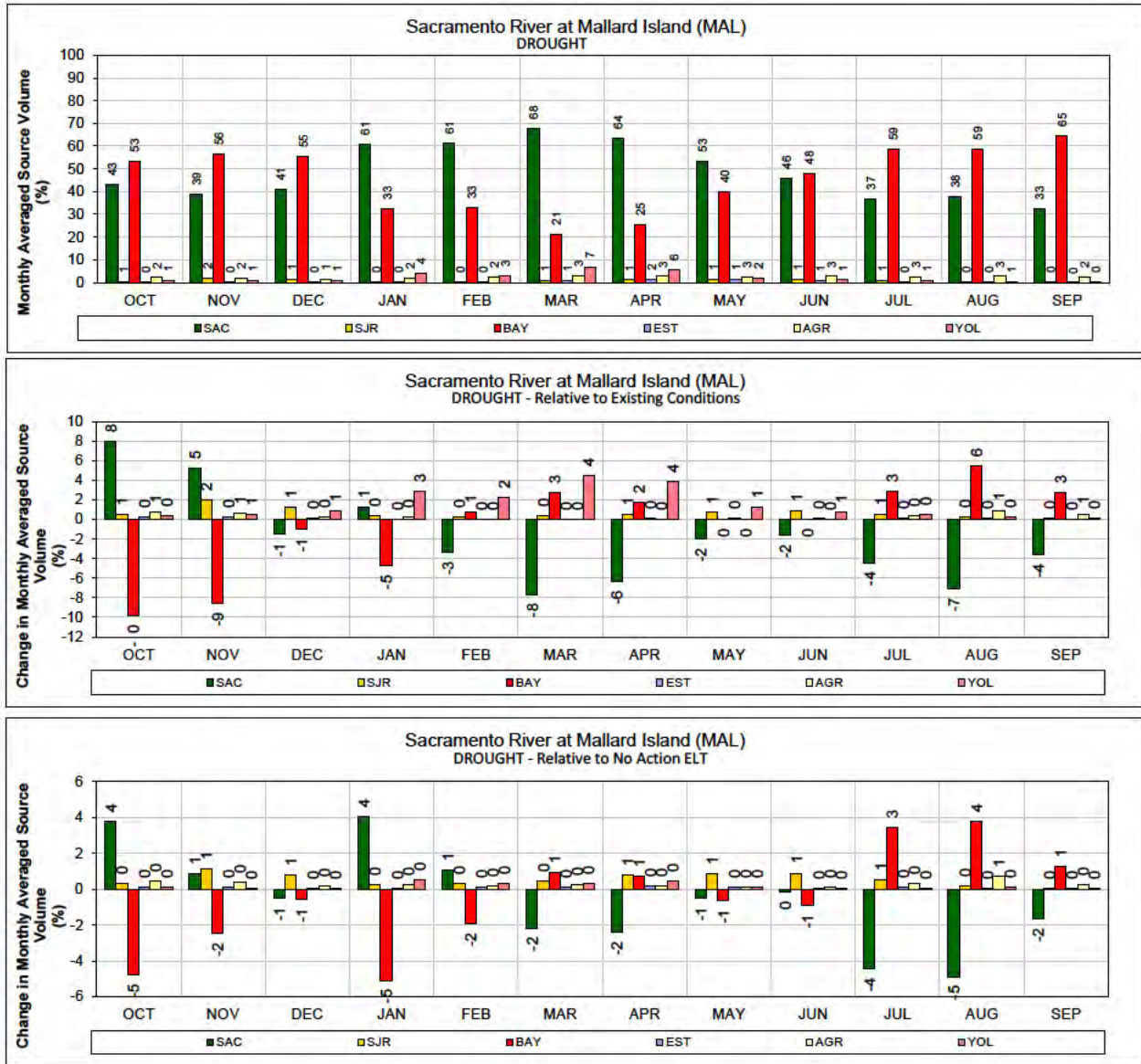
1 Figure 322. ALT 4A – Sacramento River at Mallard Island for DROUGHT years (1987-1991) 2 Monthly average source volume (top figure) and change in monthly average source volume relative to 3 Existing Conditions and No Action Alternative Early Long Term (bottom two figures).
