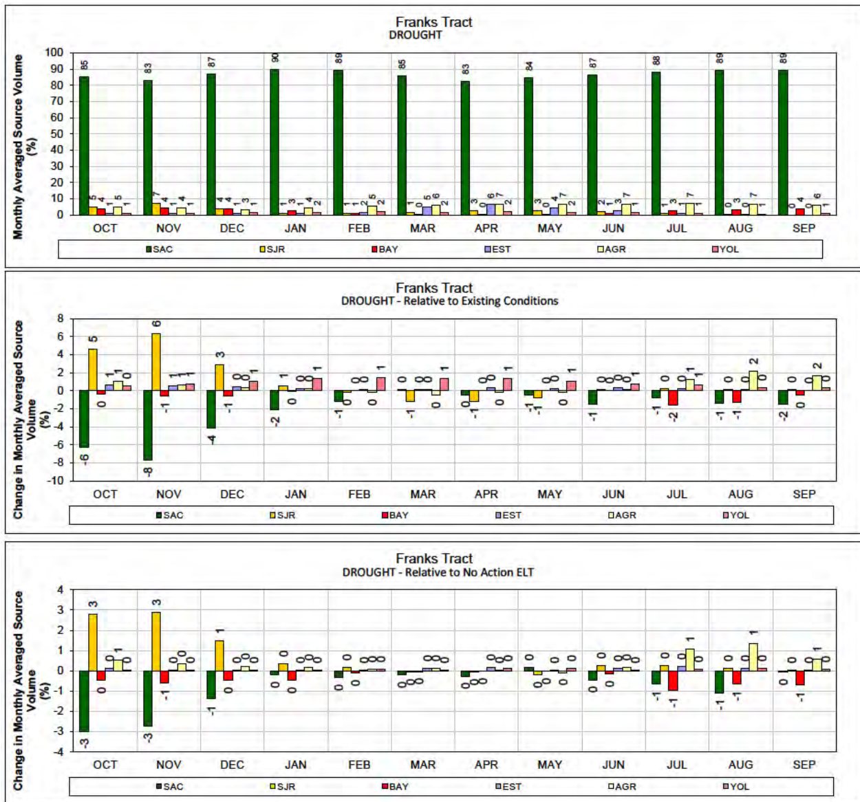
1 Figure 358. ALT 5A – Franks Tract for DROUGHT years (1987-1991) 2 Monthly average source volume (top figure) and change in monthly average source volume relative to 3 Existing Conditions and No Action Alternative Early Long Term (bottom two figures).
