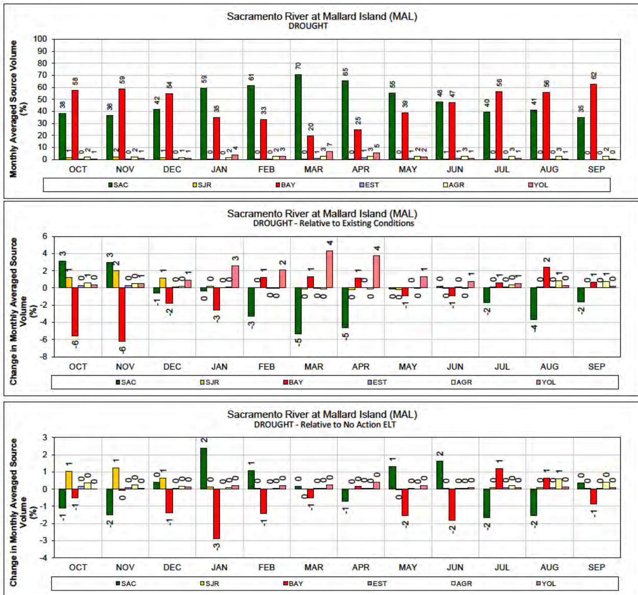
1 Figure 366. ALT 5A – Sacramento River at Mallard Island for DROUGHT years (1987-1991) 2 Monthly average source volume (top figure) and change in monthly average source volume relative to 3 Existing Conditions and No Action Alternative Early Long Term (bottom two figures).
