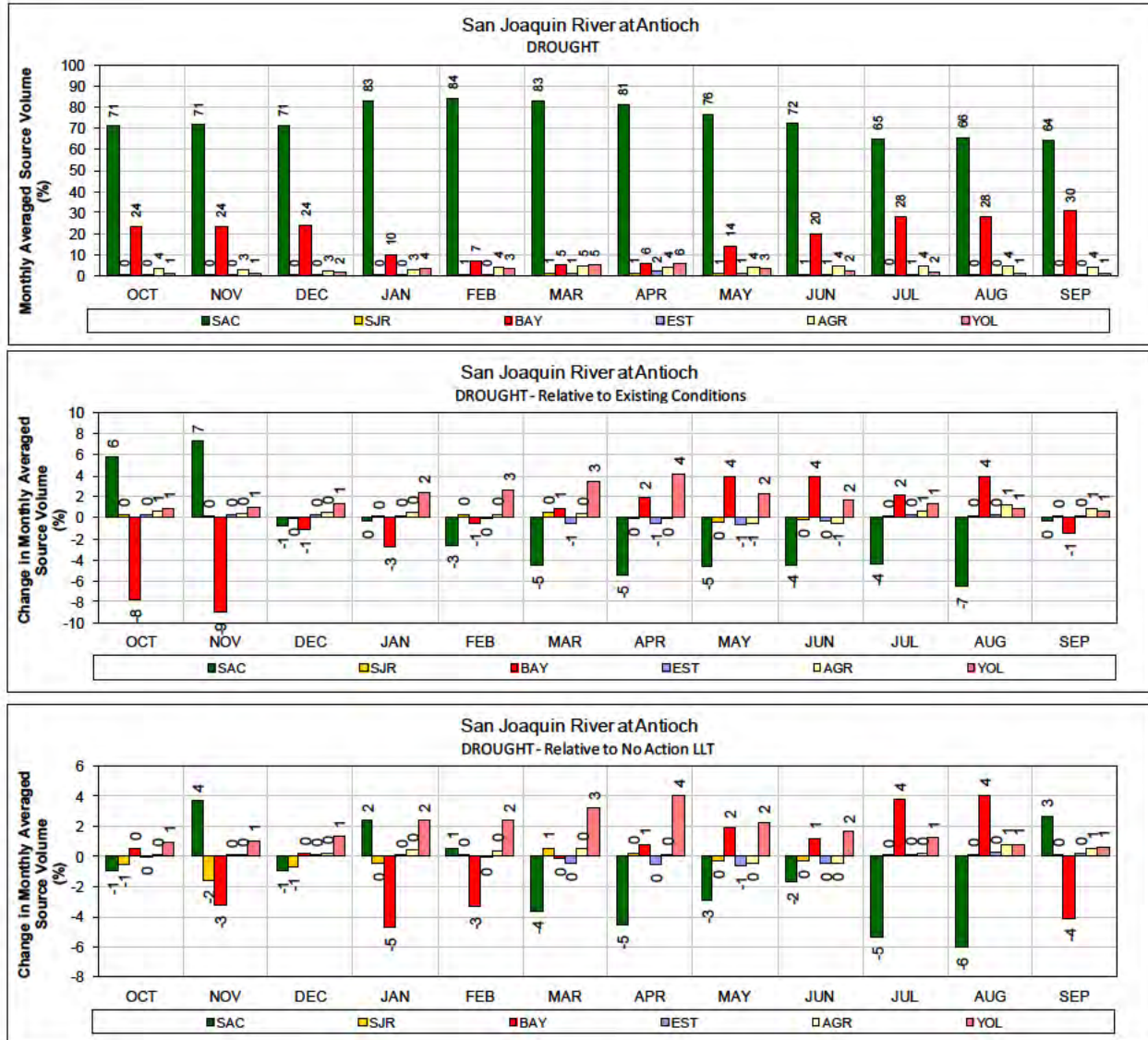
1 Figure 78. ALT 3 – San Joaquin River at Antioch for DROUGHT years (1987-1991) 2 Monthly average source volume (top figure) and change in monthly average source volume relative to 3 Existing Conditions and No Action Alternative Late Long Term (bottom two figures).
