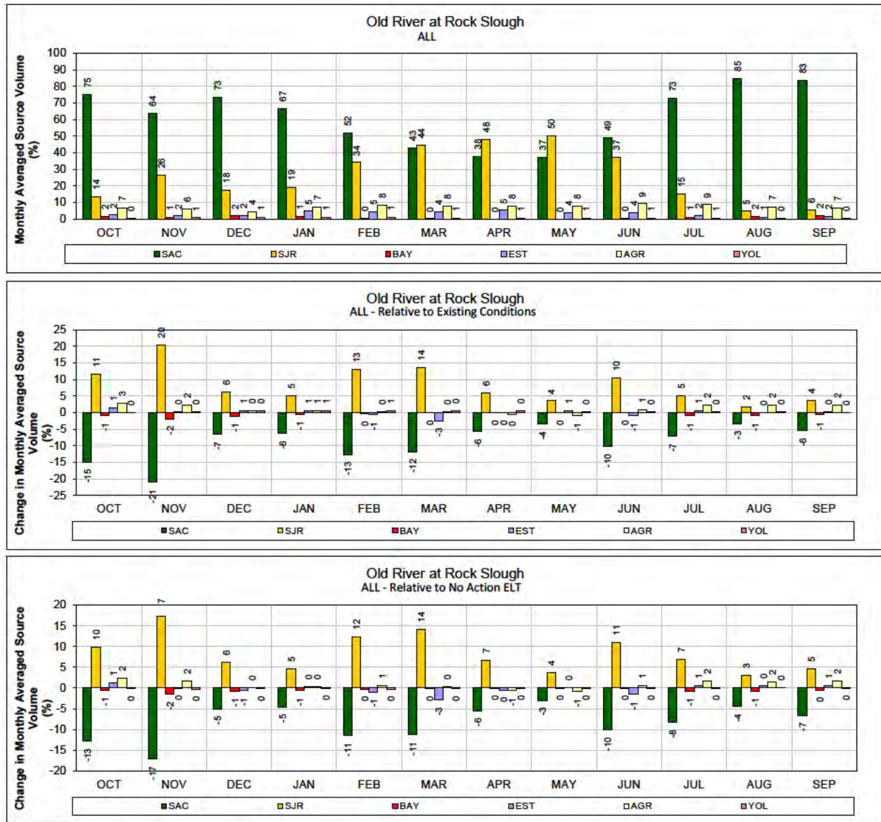
1 Figure 315. ALT 4A – Old River at Rock Slough for ALL years (1976-1991) 2 Monthly average source volume (top figure) and change in monthly average source volume relative to 3 Existing Conditions and No Action Alternative Early Long Term (bottom two figures).
