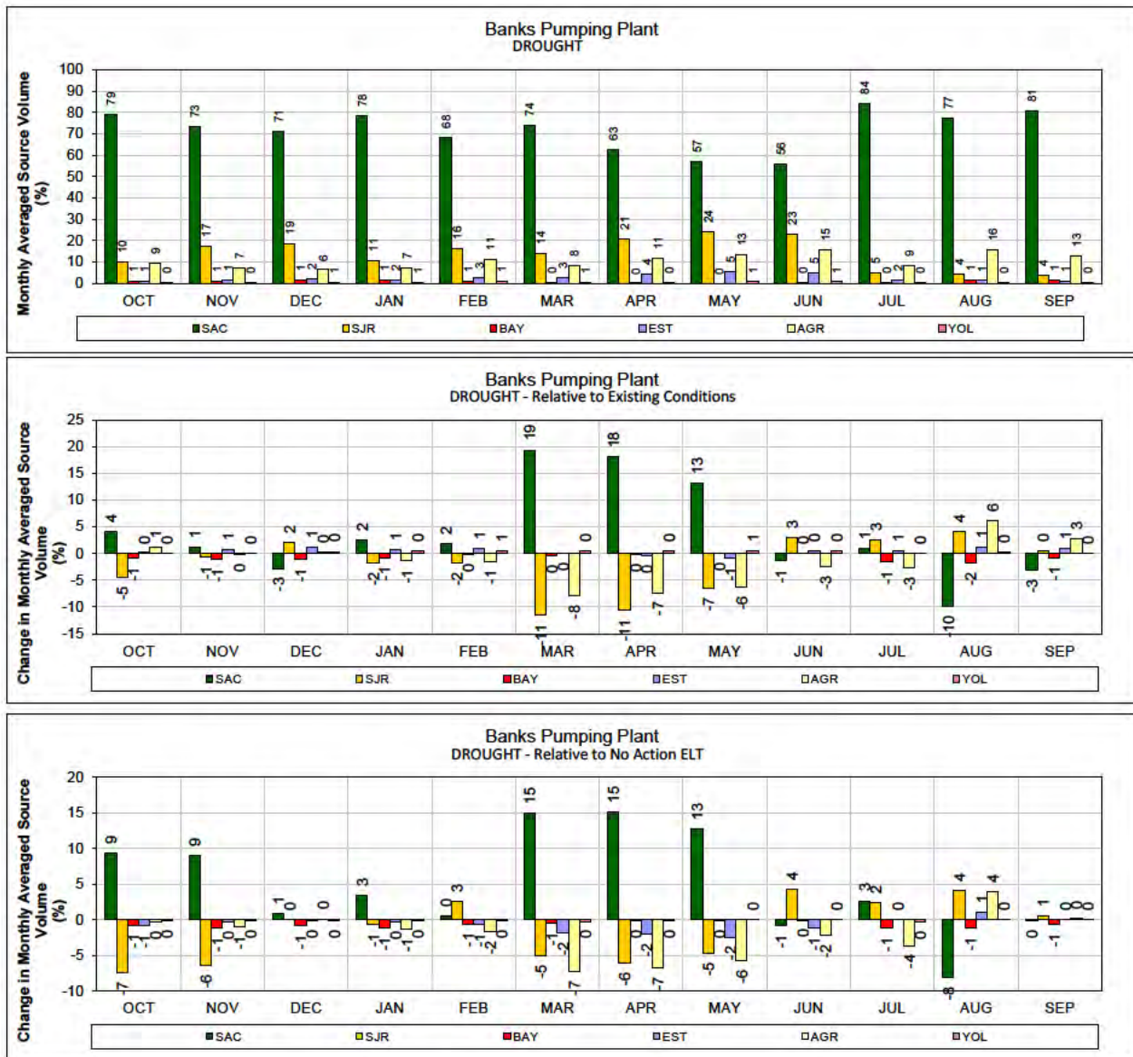
1 Figure 350. ALT 2D – Banks Pumping Plant for DROUGHT years (1987-1991) 2 Monthly average source volume (top figure) and change in monthly average source volume relative to 3 Existing Conditions and No Action Alternative Early Long Term (bottom two figures).
