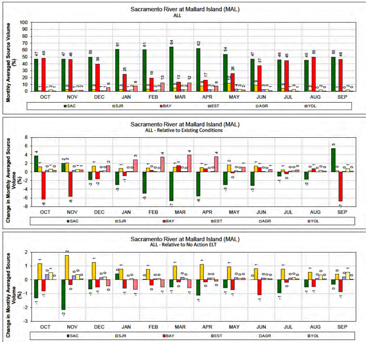
1 Figure 365. ALT 5A – Sacramento River at Mallard Island for ALL years (1976-1991) 2 Monthly average source volume (top figure) and change in monthly average source volume relative to 3 Existing Conditions and No Action Alternative Early Long Term (bottom two figures).
