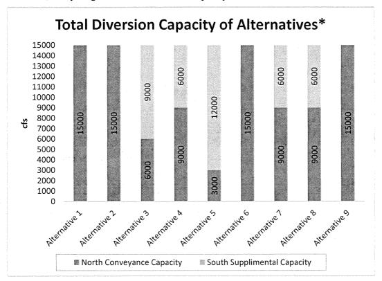
observed, every single out would have the capacity to divert 15,000 cfs from the delta.
