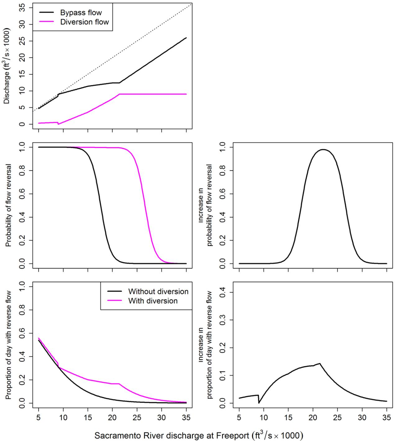
**Figure 9.** Effect of North Delta Diversion (NDD) on bypass discharge, probability of flow reversal, and proportion of the day with reverse flow for Level 3 post-pulse operations in May as defined in the NDD bypass rules. In the top panel, the dotted line shows bypass discharge when diversion discharge is zero.
