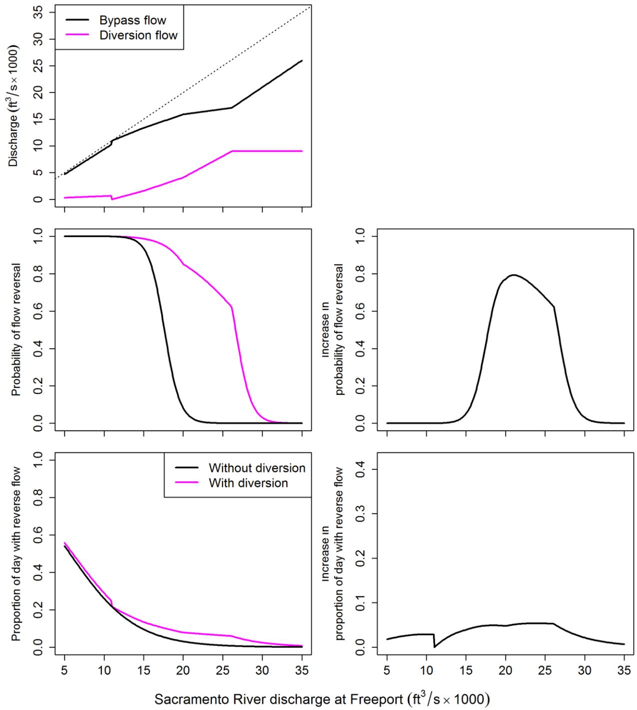
**Figure 5.** Effect of North Delta Diversion (NDD) on bypass discharge, probability of flow reversal, and proportion of the day with reverse flow for Level 2 post-pulse operations in December–April as defined in the NDD bypass rules. In the top panel, the dotted line shows bypass discharge when diversion discharge is zero.
