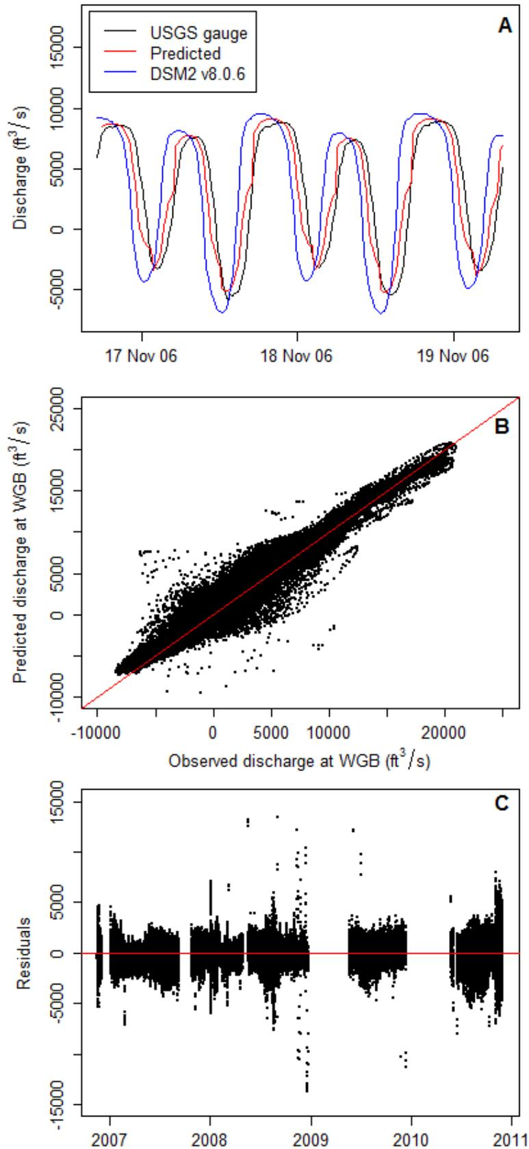
Figure 15. Comparison of observed, DSM2v8.0.6, and regression-corrected (predicted) discharge at the
