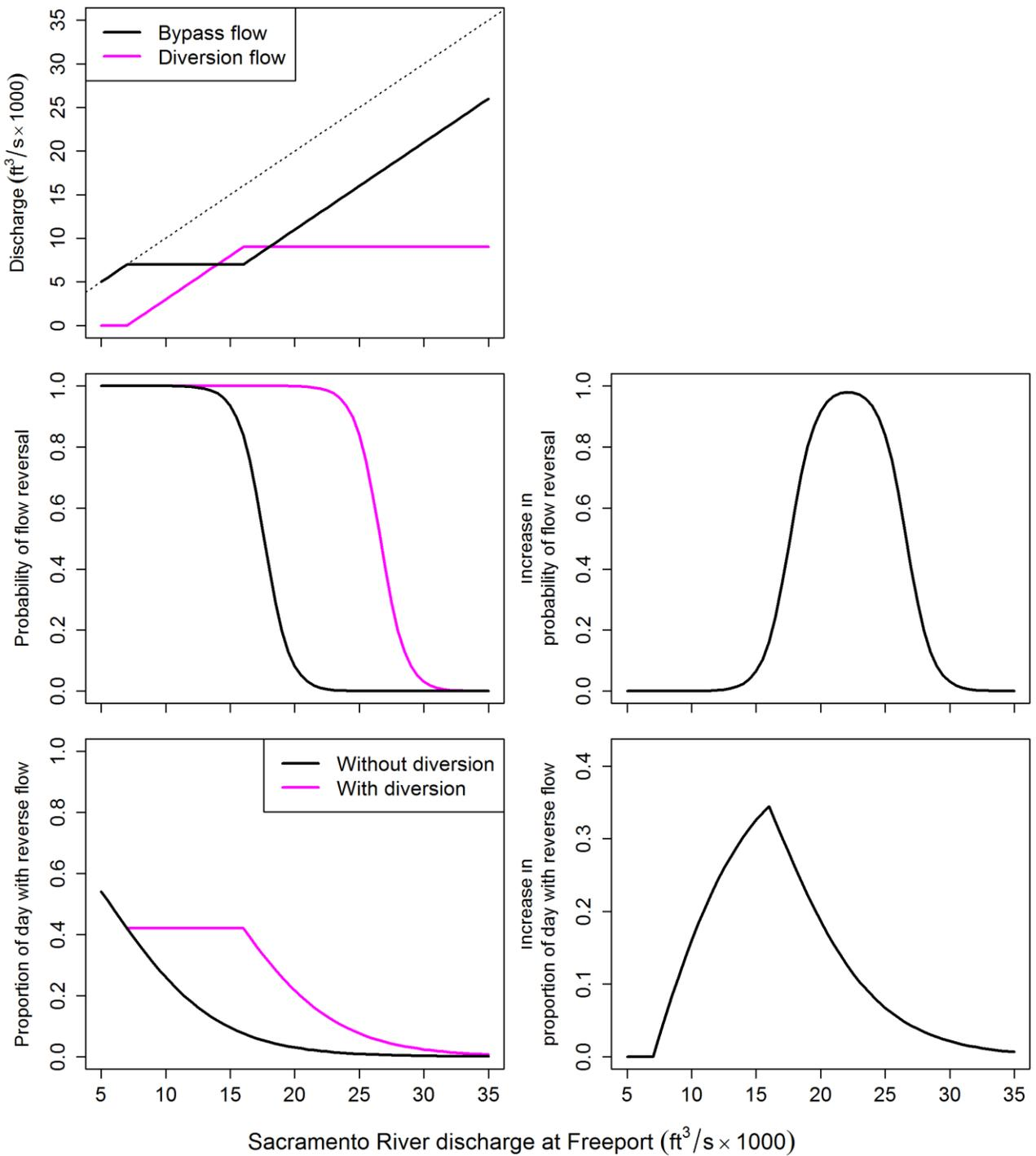
**Figure 3.** Effect of North Delta Diversion (NDD) on bypass discharge, probability of flow reversal, and proportion of the day with reverse flow for October–November as defined in the NDD bypass rules. In the top panel, the dotted line shows bypass discharge when diversion discharge is zero.
