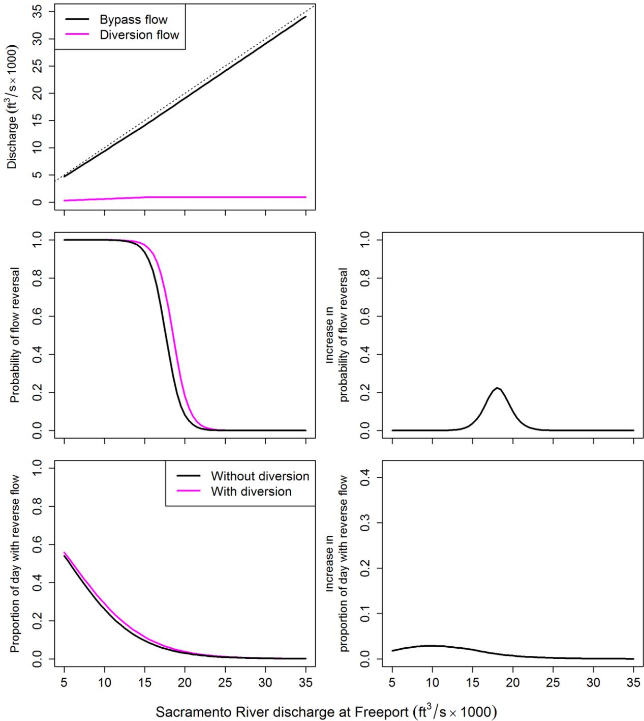
**Figure 2.** Effect of North Delta Diversion (NDD) on bypass discharge, probability of flow reversal, and proportion of the day with reverse flow for constant low-level pumping as defined in the NDD bypass rules. In the top panel, the dotted line shows bypass discharge when diversion discharge is zero.
