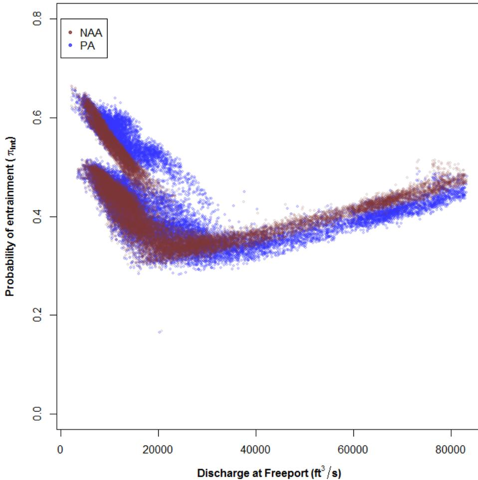
**Figure 16.** Daily probability of entering the interior Delta ( $\pi_{int} = \pi_{GEO} + \pi_{DCC}$ ) as a function of Sacramento River discharge at Freeport for the No Action Alternative (NAA) and Proposed Action (PA) simulations conducted with DSM2 (Delta Simulation Model 2).
