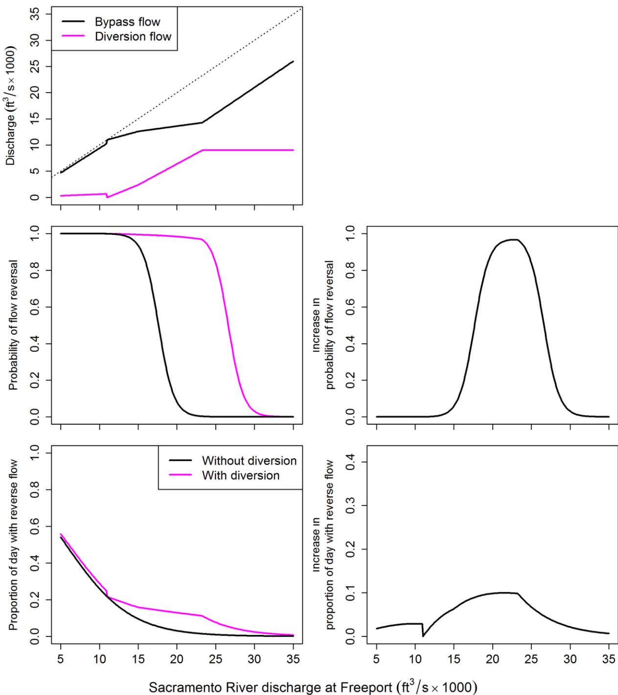
**Figure 11.** Effect of North Delta Diversion (NDD) on bypass discharge, probability of flow reversal, and proportion of the day with reverse flow for Level 2 post-pulse operations in June as defined in the NDD bypass rules. In the top panel, the dotted line shows bypass discharge when diversion discharge is zero.
