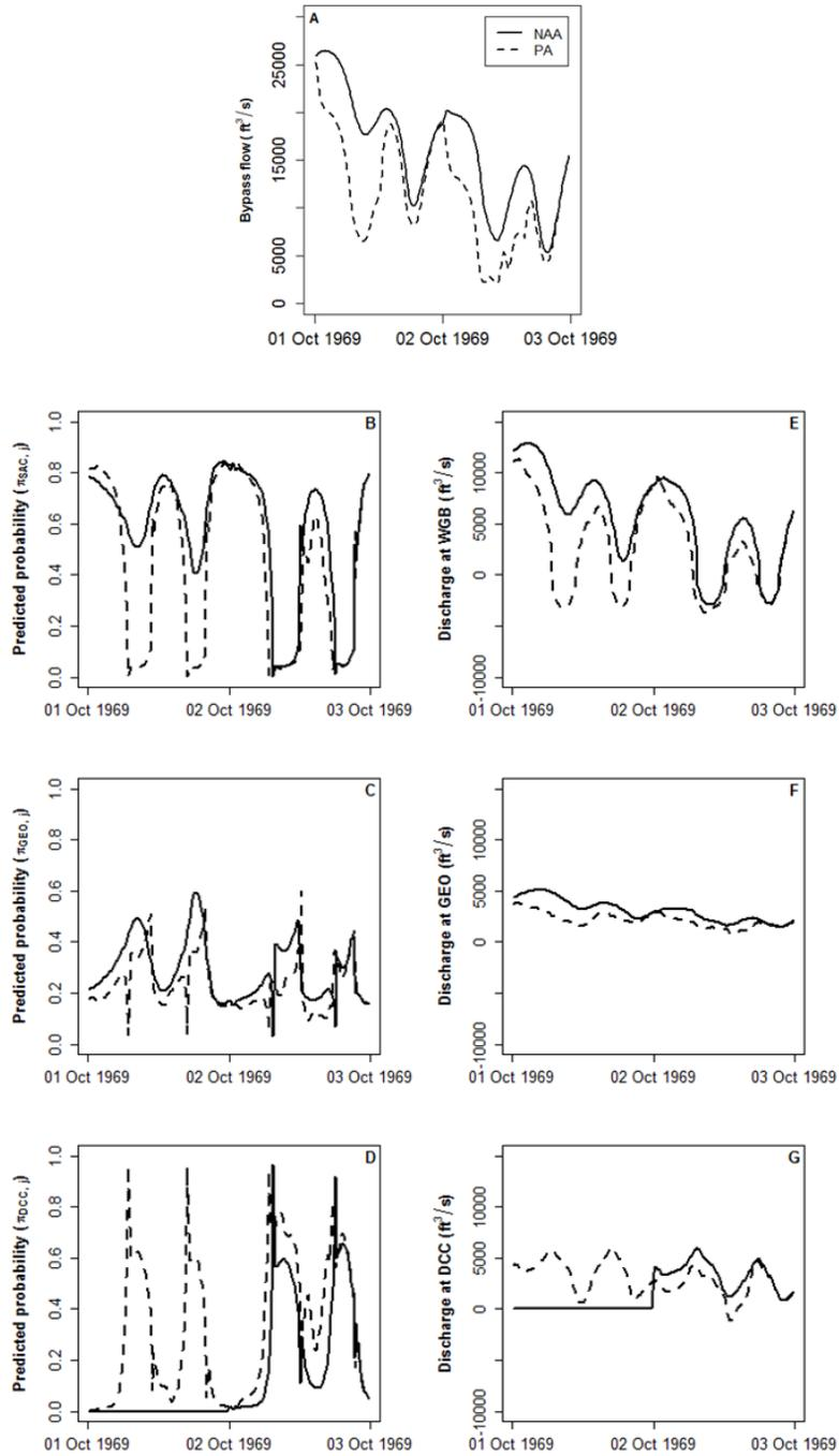
**Figure 22.** Comparison of bypass flows (A), predicted probability of entrainment into Sacramento River (B), Georgiana Slough (C), and the Delta Cross Channel (D) for the Proposed Action (PA) and No Action Alternative (NAA) during dates when the DCC was open under PA but closed under NAA. Discharge entering each route for NAA and PA are also shown (E, F, G).
