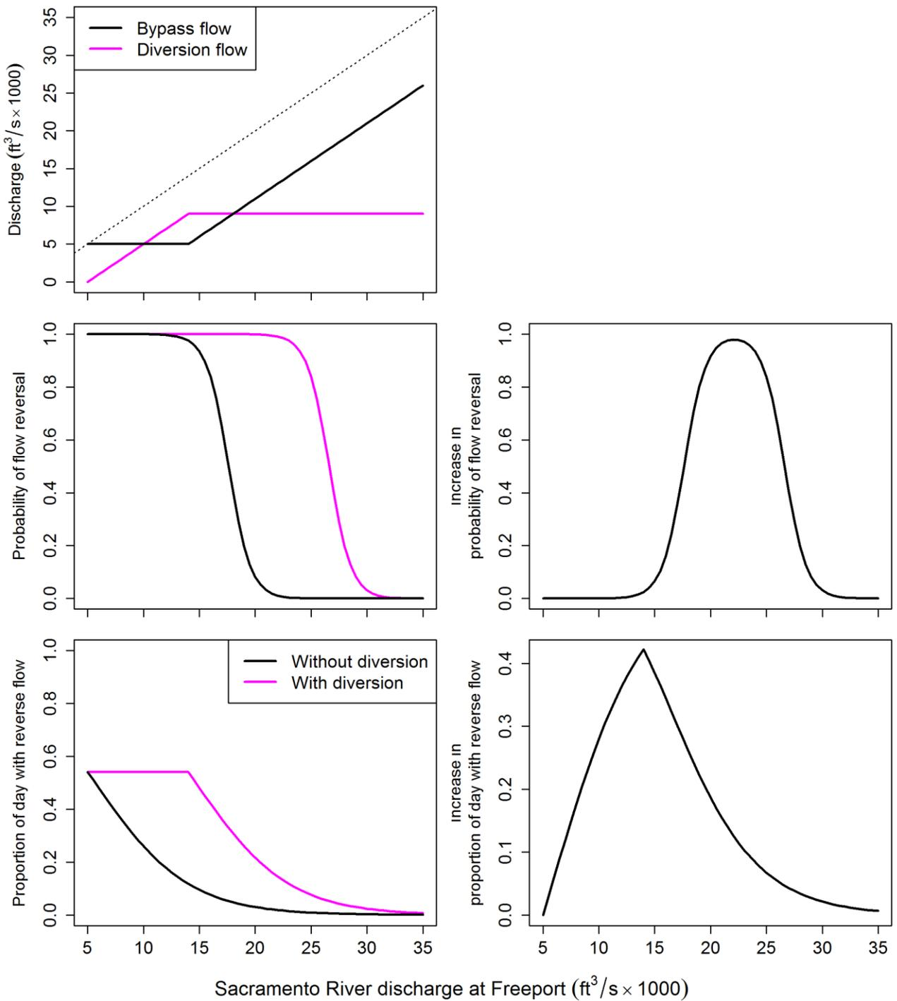
**Figure 13.** Effect of North Delta Diversion (NDD) on bypass discharge, probability of flow reversal, and proportion of the day with reverse flow for July–December as defined in the NDD bypass rules. In the top panel, the dotted line shows bypass discharge when diversion discharge is zero.
