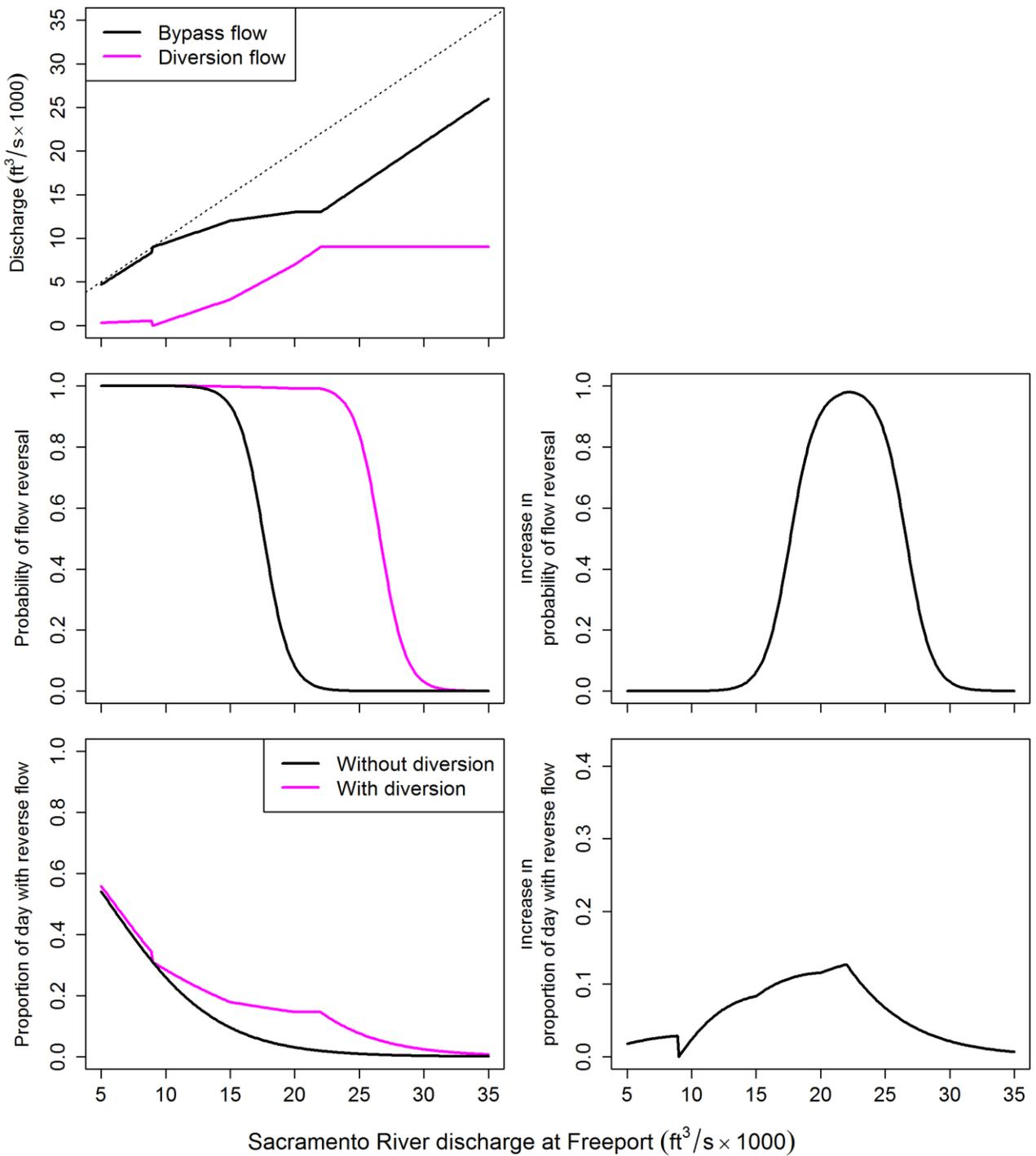
**Figure 6.** Effect of North Delta Diversion (NDD) on bypass discharge, probability of flow reversal, and proportion of the day with reverse flow for Level 3 post-pulse operations in December–April as defined in the NDD bypass rules. In the top panel, the dotted line shows bypass discharge when diversion discharge is zero.
