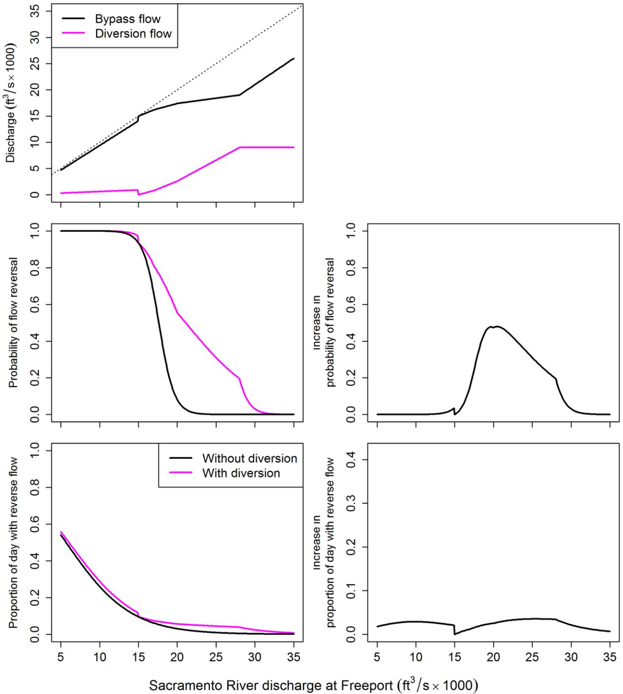
**Figure 10.** Effect of North Delta Diversion (NDD) on bypass discharge, probability of flow reversal, and proportion of the day with reverse flow for Level 1 post-pulse operations in June as defined in the NDD bypass rules. In the top panel, the dotted line shows bypass discharge when diversion discharge is zero.
