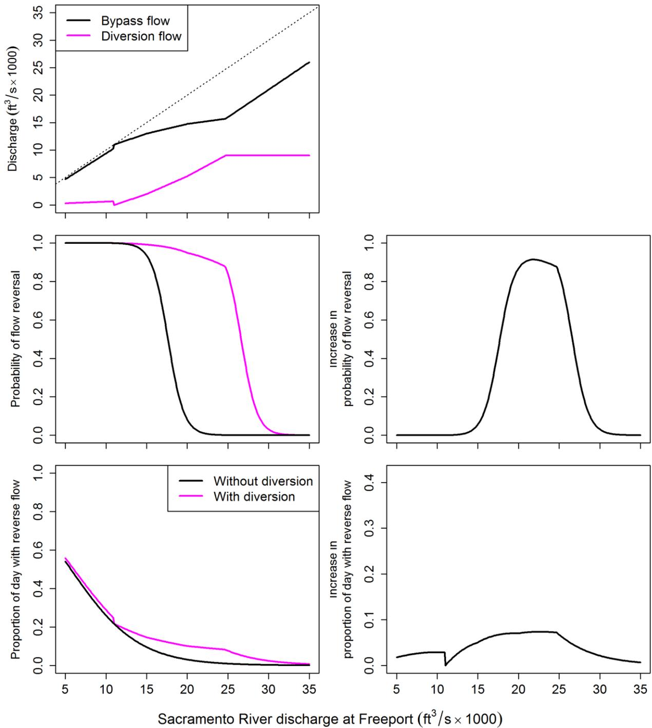
**Figure 8.** Effect of North Delta Diversion (NDD) on bypass discharge, probability of flow reversal, and proportion of the day with reverse flow for Level 2 post-pulse operations in May as defined in the NDD bypass rules. In the top panel, the dotted line shows bypass discharge when diversion discharge is zero.
