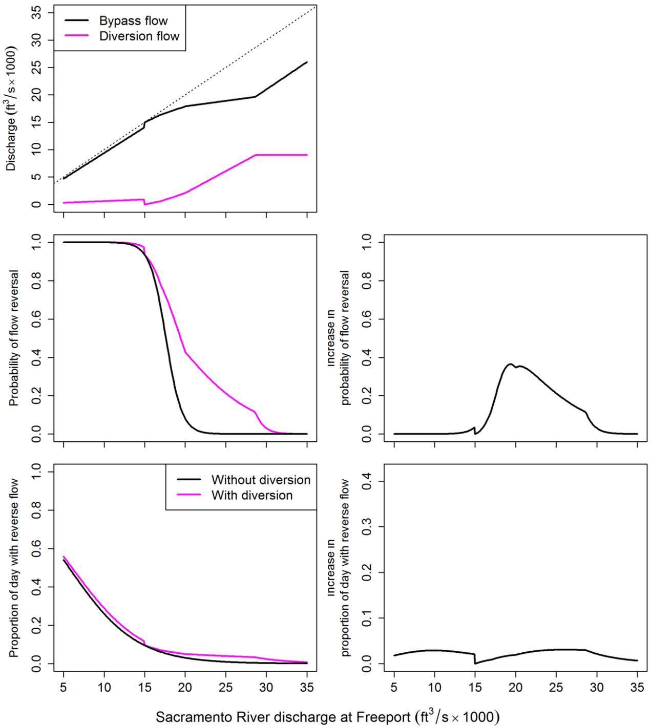
**Figure 7.** Effect of North Delta Diversion (NDD) on bypass discharge, probability of flow reversal, and proportion of the day with reverse flow for Level 1 post-pulse operations in May as defined in the NDD bypass rules. In the top panel, the dotted line shows bypass discharge when diversion discharge is zero.
