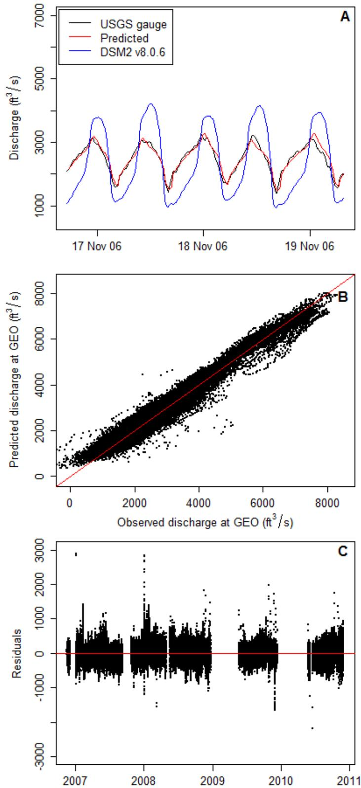
**Figure 14.** Comparison of observed, DSM2v8.0.6, and regression-corrected (predicted) discharge at the Georgiana Slough (GEO) USGS flow gage (A). Panel B compares observed and predicted discharge. The
