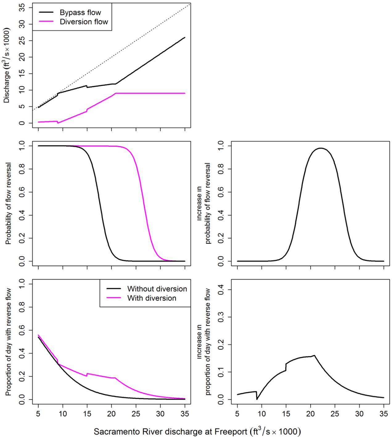
**Figure 12.** Effect of North Delta Diversion (NDD) on bypass discharge, probability of flow reversal, and proportion of the day with reverse flow for Level 3 post-pulse operations in June as defined in the NDD bypass rules. In the top panel, the dotted line shows bypass discharge when diversion discharge is zero.
