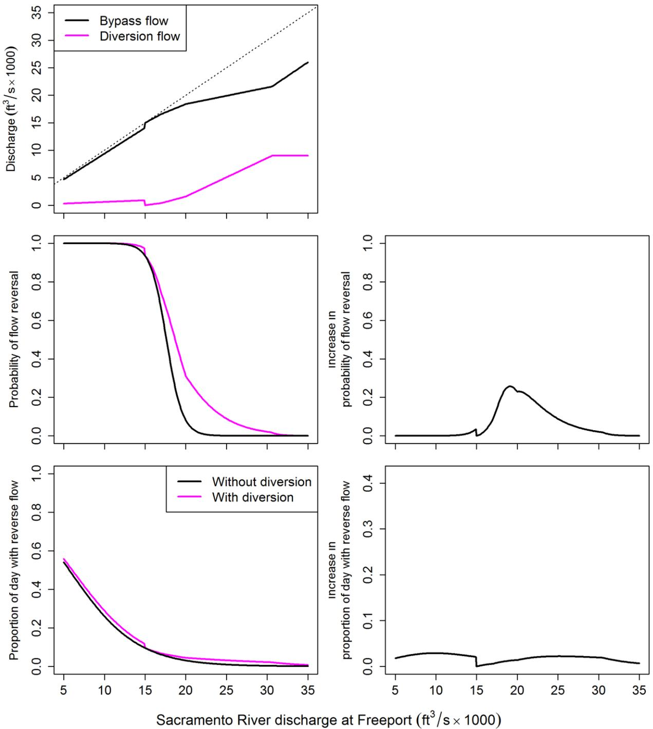
**Figure 4.** Effect of North Delta Diversion (NDD) on bypass discharge, probability of flow reversal, and proportion of the day with reverse flow for Level 1 post-pulse operations in December–April as defined in the NDD bypass rules. In the top panel, the dotted line shows bypass discharge when diversion discharge is zero.
