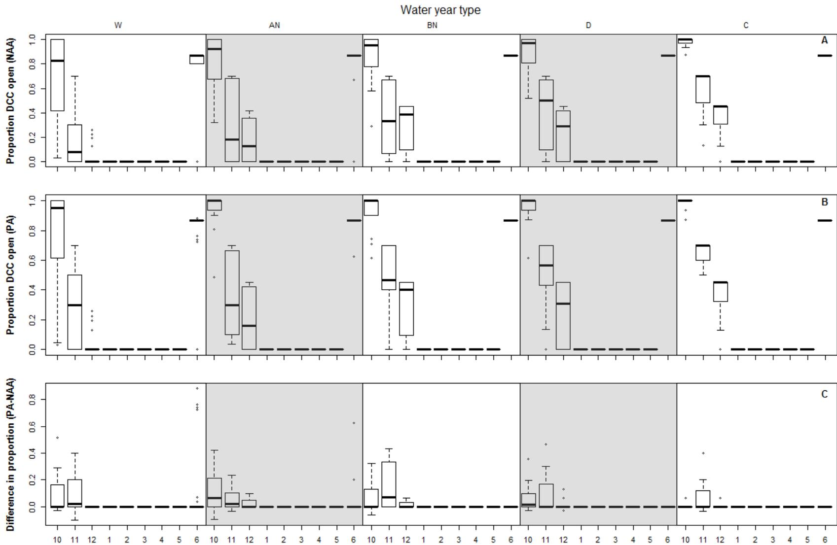
**Figure 21.** Boxplot of the proportion of each month that the DCC was open for the No Action Alternative (NAA, panel A), Proposed Action (PA, panel B), and the difference between PA and NAA (panel C) by water year type (W=Wet, AN=Above Normal, BN=Below Normal, D=Dry, C=Critical). Boxes range from the 25th to the 75th percentiles with a line indicating the median, whiskers extend 1.5 times past the length of the box, and dots represent data points that fall beyond the whiskers.
