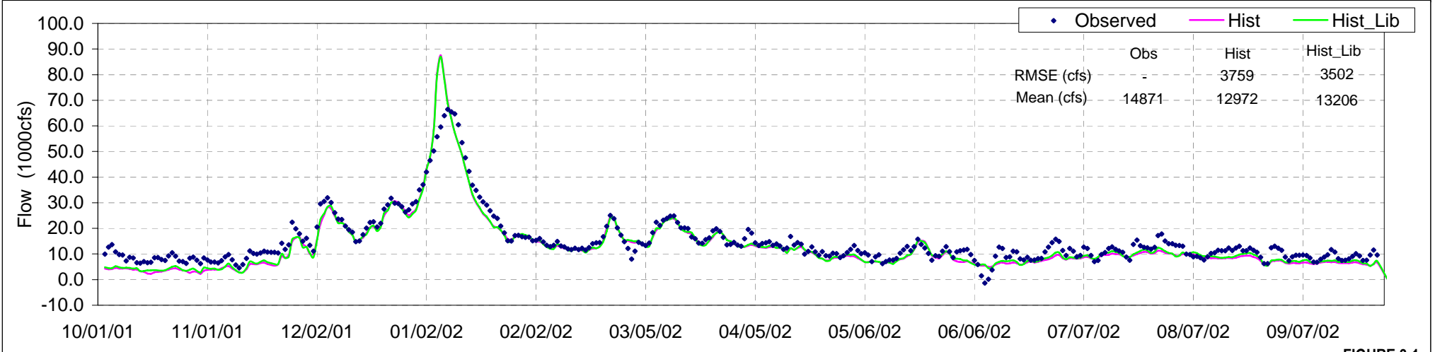
FIGURE 3-1 Sample Plot Showing the Metrics for Evaluating HYDRO Calibration
