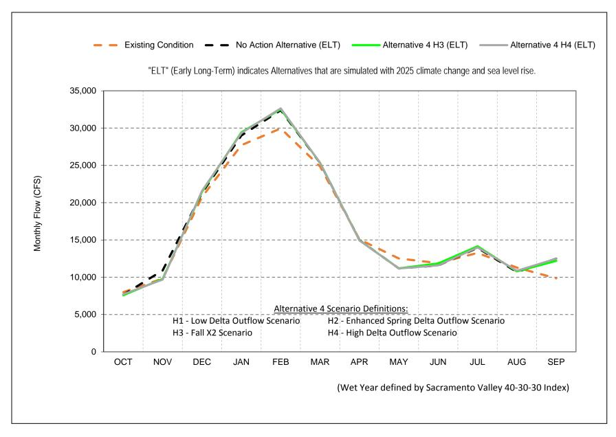
Figure 4.3.2-1 Sacramento River at Bend Bridge for Alternative 4A, Average Wet Years
