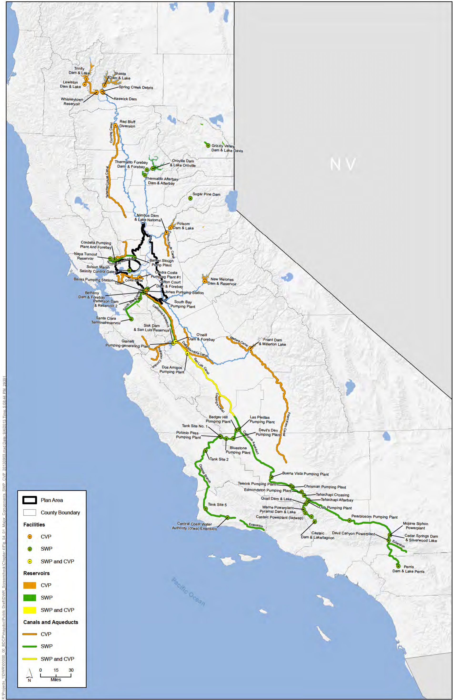
GIS Data Source: Dams/Pumps, DWR 1994; SWPCVP Lakes, HDR 2011; SWPCVP Canals/Aqueducts, HDR 2011. Figure 4-1 Major Components of the State Water Project (SWP) and Central Valley Project (CVP)
