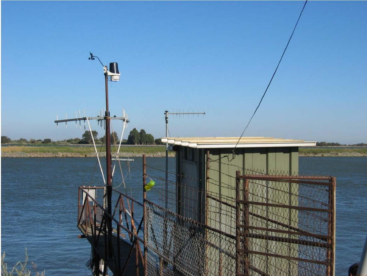
Figure 5.5 - Radar antenna installed at Three-mile slough gage.
