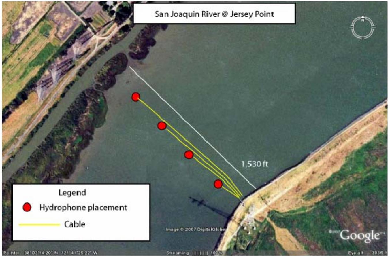
Figure 6.3 - Proposed 4-port system: hydrophone and communication cable locations in the San Joaquin River, at Jersey Point (JER). Exact hydrophone and cable locations will be determined through detailed field reconnaissance and testing conducted in the summer/fall of 2007.
