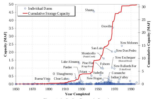
Figure A-6 – Surface Reservoir Capacity
