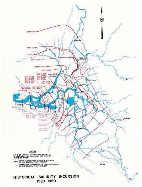
Figure D-12 – Salinity intrusion during 1920-1960 (DWR, 1960)
