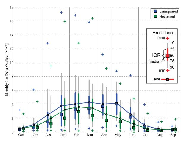
**Figure 3-6 – Monthly distribution of Net Delta Outflow**Distribution of monthly NDO for water years 1930 through 2008. Monthly averages are indicated by the lines with black circles. Monthly median is given by the squares, while the interquartile range is indicated by the vertical line for each month and the vertical grey line extends to the 10th and 90th percentiles. Maximum and minimum values are indicated by '+' marks.
