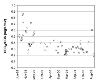
**Figure 3.** Ratio of point concentration to optical backscatter for Three Mile Slough, illustrating the drift in sensor voltage output with time.
