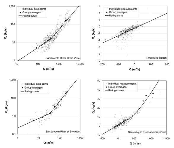
Figure 7. Daily suspended-sediment rating curves for four of the optical sensors sites.
