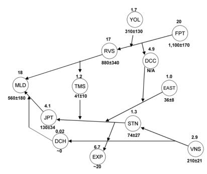
**Figure 9.** Average annual delta water and sediment budgets based on water years 1999-2002, except for TMS, which is based on water years 2001 and 2002 only. For each location the top number is annual water flux in billion m<sup>3</sup>, and the bottom number is annual suspended-sediment flux and the estimated error in thousand metric tons.
