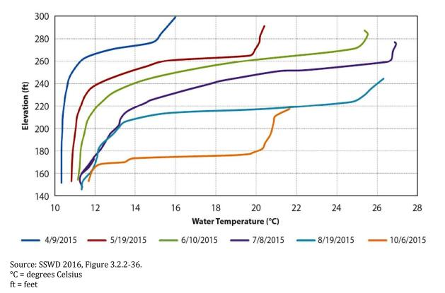
Figure A1c-25. Water Temperature (°C) Profiles Measured Downstream of Camp Far West Reservoir in the Bear River by South Sutter Water District (2015)
