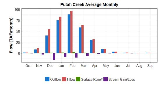
Figure A7-21. Monthly Average Unimpaired Flow Components for Putah Creek
