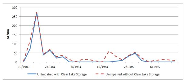
Figure A7-29. Monthly Unimpaired Flow on Cache Creek below Clear Lake for Water Years 1984– 1985
