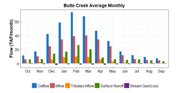
Figure A7-7. Monthly Average Unimpaired Flow Components for Butte Creek
