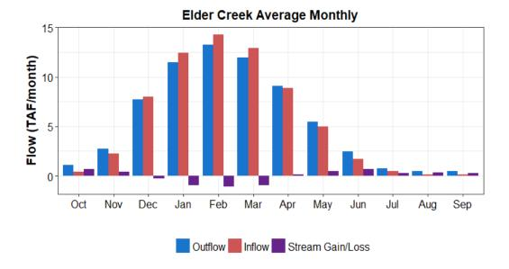
Figure A7-15. Monthly Average Unimpaired Flow Components for Elder Creek
