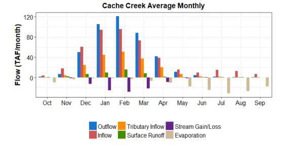
Figure A7-8. Monthly Average Unimpaired Flow Components for Cache Creek
