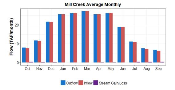
Figure A7-17. Monthly Average Unimpaired Flow Components for Mill Creek
