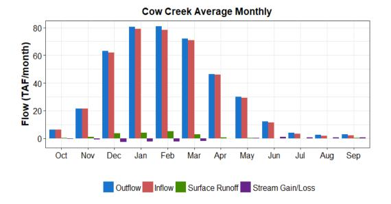
Figure A7-13. Monthly Average Unimpaired Flow Components for Cow Creek
