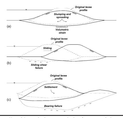
Figure 5.4. Potential levee failure modes due to seismic loading. (Source: Brandenberg and Stewart 2006)
