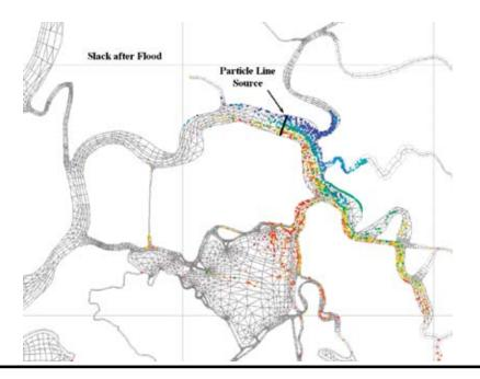
Figure 6.4. Particle Tracking: San Joaquin River near Mokelumne River. Details of the finite element grid used within RMA2. The image shows the locations of particles at some time after their simulated release. Results are shown for illustration purposes only. (Source: Resource Management Associates 2007)
