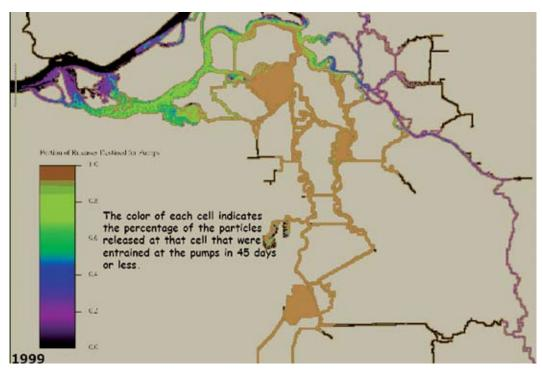
Figure 6.6. Percent of Particles Entrained at Pumps for Aug 15 Particle Release. Display of results from particle fate mapping using August 15, 1999 as the simulated condition for the Delta. (Source: P. Smith, USGS, unpublished material)
