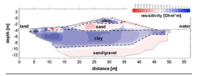
Figure 5.3. An example of the subsurface structure of a levee as determined by resistivity measurements. (Source: Niederleithinger et al. 2005)
