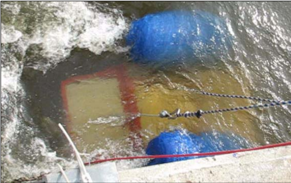
Figure 17. Release of tagged steelhead immediately upstream of the radial gates using the live-car. Two blue floats were attached to the live-car and used to float the live-car into position directly upstream of the radial gates.
