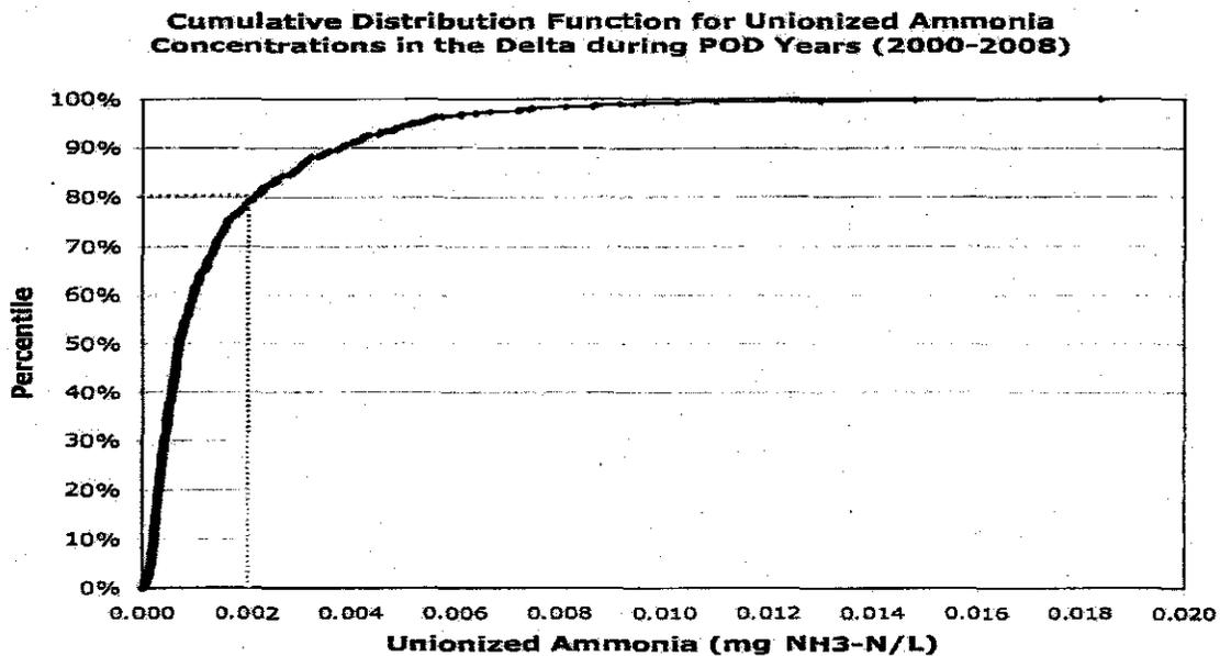
**Figure 2. Cumulative distribution of un-ionized ammonia concentrations (N = 639) from freshwater Delta monitoring stations at which total ammonia, pH, water temperature and EC were measured during POD years (2000-2008). Station names and monitoring entities are identified in Table 1. Data for Freeport were omitted from the cumulative distribution.**
