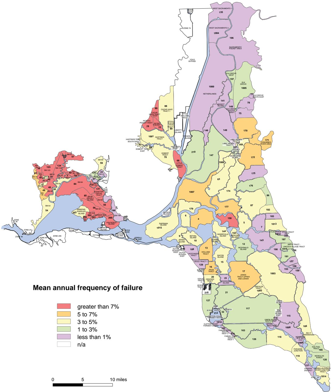
**FIGURE 14. Annual Frequency Of Failures Of Individual Islands Under Flooding Events**
