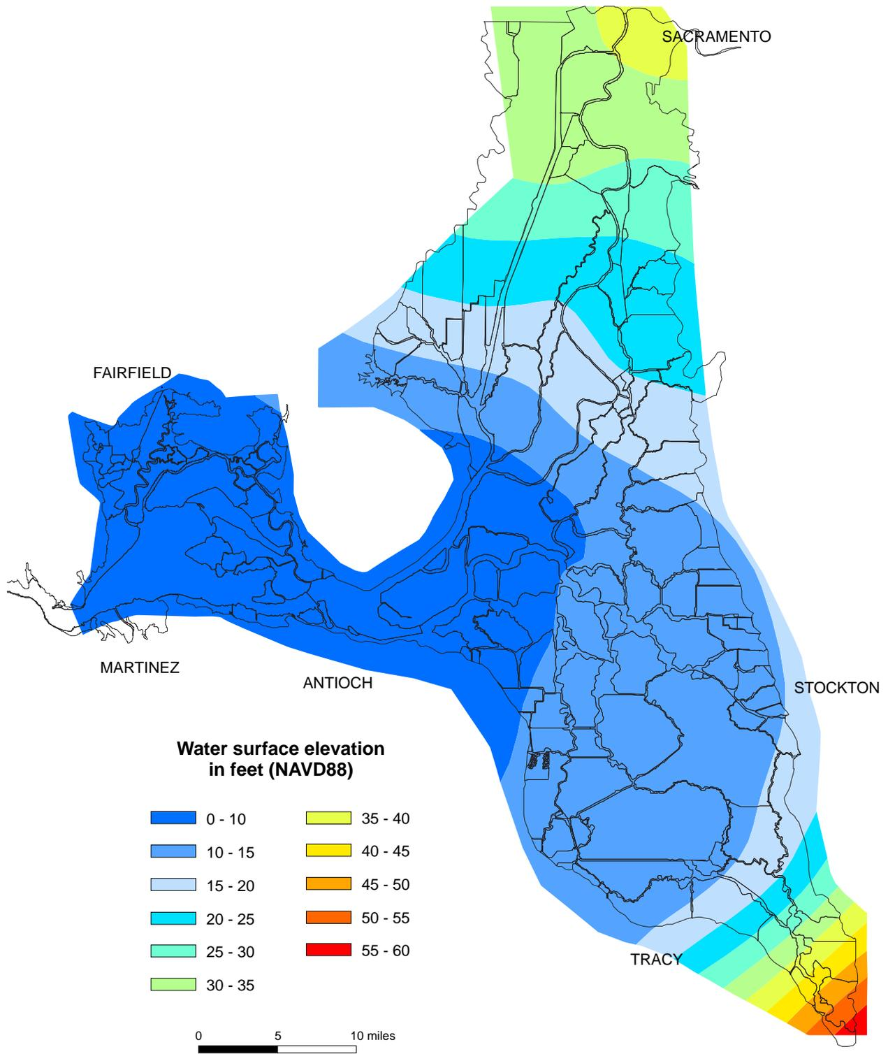
**FIGURE 5. Example Water Surface Elevations During Extreme Flood Events In The Delta.**
