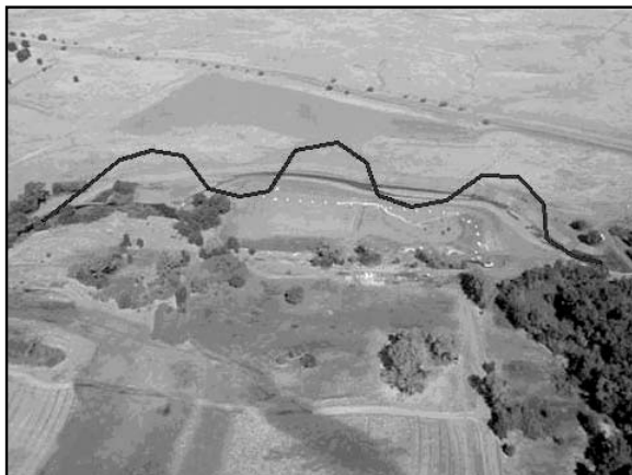
FIGURE 4. Oblique aerial view of Best Slough pre-project, showing initial restoration proposal (for a meandering channel) superimposed on photo. Flow is right to left. Photo by Beale Air Force Base Summer 2000.
