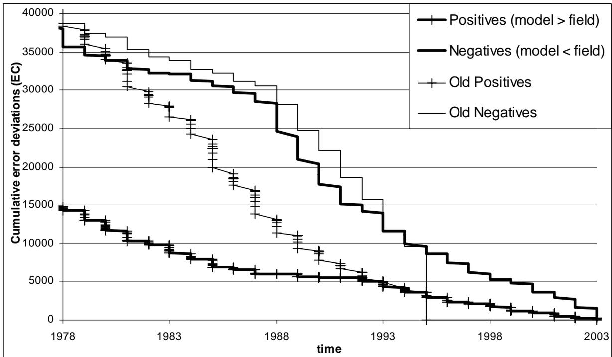
**Figure B2. Cumulative positive and negative deviations of new and old CalSim II models from historical data, going backwards from 2003. Old model results (which end in 1994) are begun at the same values as the new model in 1994.**
