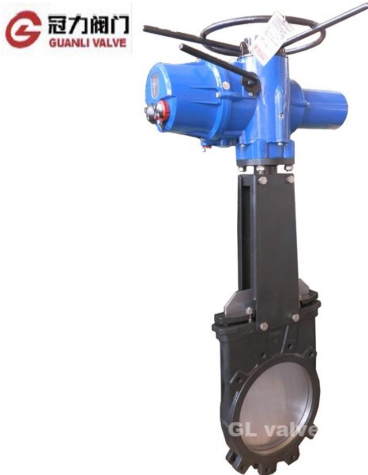
*ELECTRIC VALVE - Example of small, computer controlled, 3" electric Knife valve installed at each customer box (POU) and secured to standard NID plywood orifice as a drop in replacement. Cost @20x : \$200 ~ \$300 ea. (Less in volume.)*
