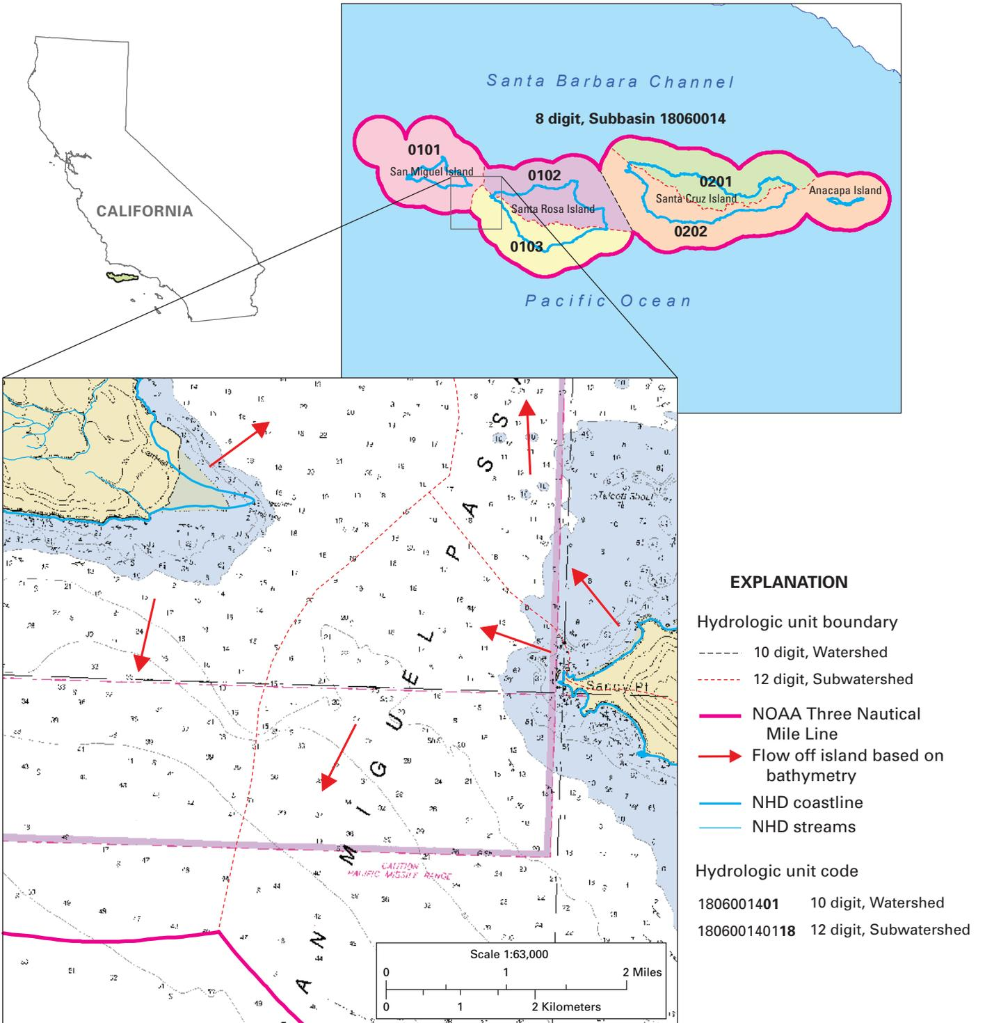
**Figure 14.** For an island that is beyond the mainland NOAA Three Nautical Mile Line, such as the Channel Islands off the California coast, the outer extent of the island hydrologic unit is the NOAA Three Nautical Mile Line. The nearshore delineation is optional.
