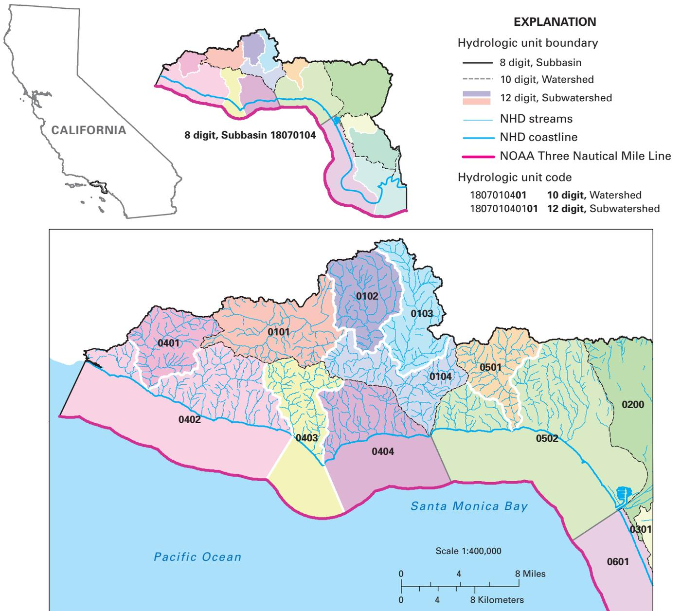
**Figure 12.** The outer extent of these standard and frontal hydrologic units in the Santa Monica Bay area, California, is delineated to the first offshore boundary, the NOAA Three Nautical Mile Line. (NHD, National Hydrography Dataset; NOAA, National Oceanic and Atmospheric Administration)
