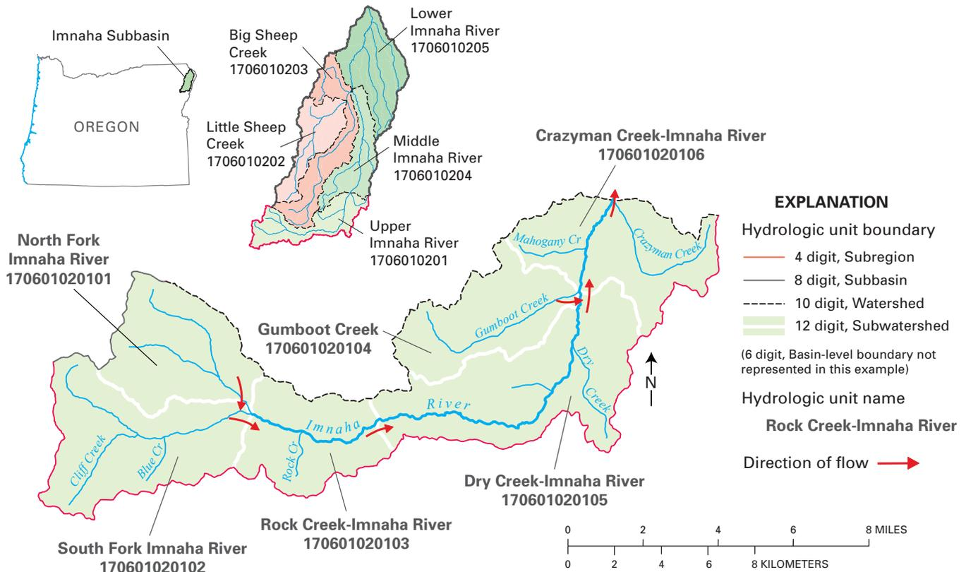
**Figure 17.** Each hydrologic unit should be coded sequentially based on the location of the outlet, starting with the uppermost stream outlet. The downstream code should always be a higher number than the upstream code for 10- and 12-digit hydrologic units. The main-stem hydrologic unit should carry the higher code when outlets are adjacent or break at the same place. Codes are shown for the Upper Imnaha River 10-digit hydrologic unit.
