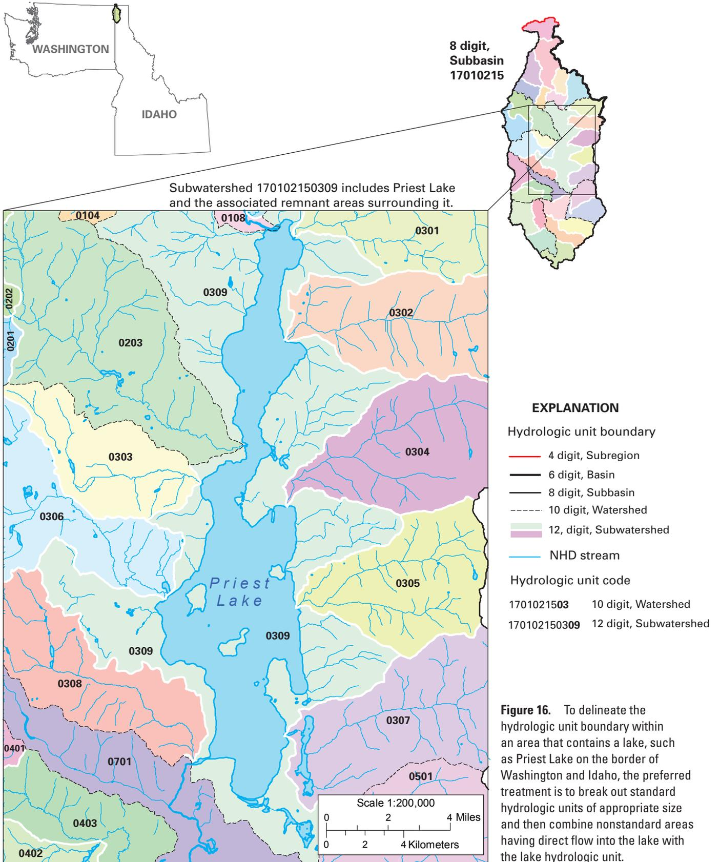
**Figure 16.** To delineate the hydrologic unit boundary within an area that contains a lake, such as Priest Lake on the border of Washington and Idaho, the preferred treatment is to break out standard hydrologic units of appropriate size and then combine nonstandard areas having direct flow into the lake with the lake hydrologic unit.
