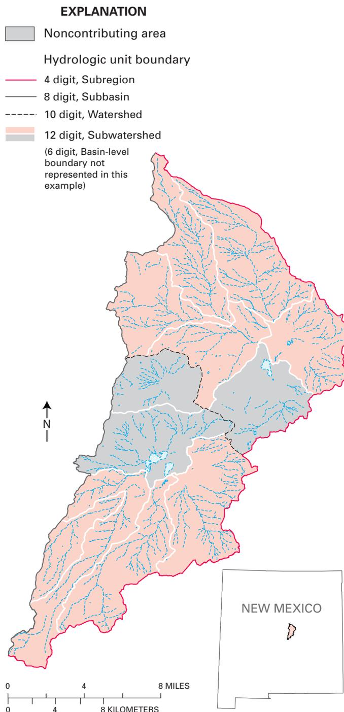
**Figure 7.** Noncontributing areas, caused by unique and unusual landforms, do not flow to the outlet of the hydrologic unit. Isolated noncontributing areas such as these in Eastern Estancia Subbasin, Torrance County, New Mexico, should be delineated.
