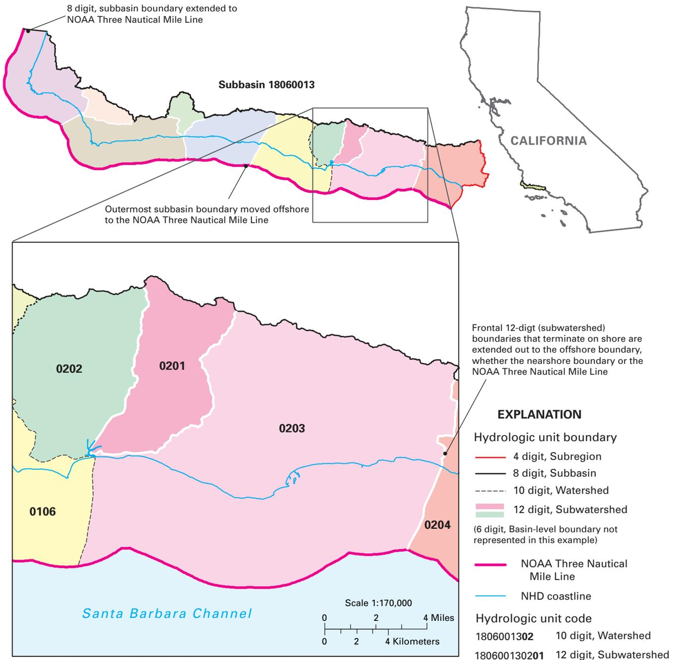
**Figure 8.** To delineate the hydrologic unit boundary for frontal hydrologic units in open ocean areas, extend the boundaries of the frontal unit to intersect offshore boundaries. (NHD, National Hydrography Dataset; NOAA, National Oceanic and Atmospheric Administration)
