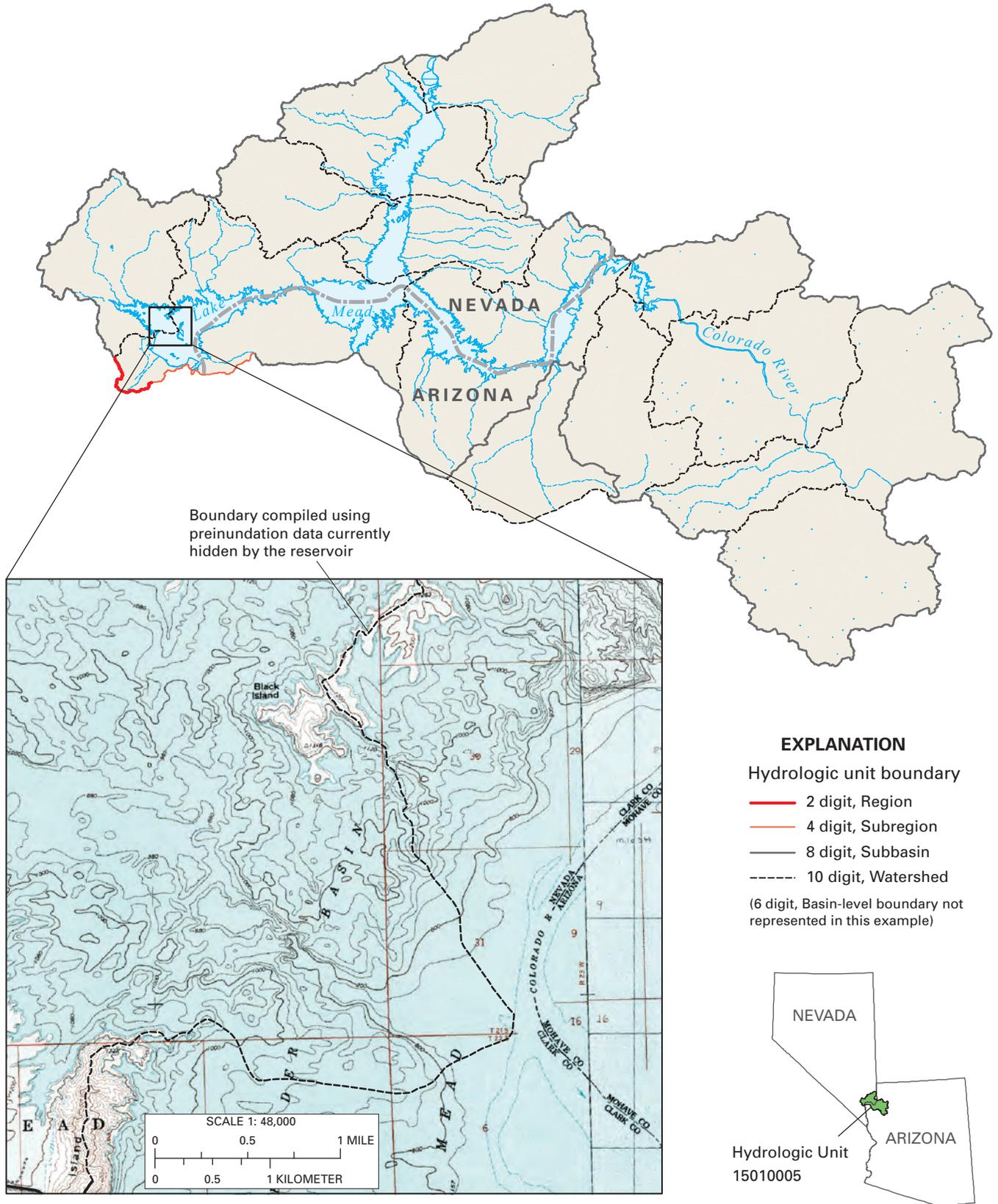
**Figure 15.** To delineate the hydrologic unit boundary within a hydrologic unit that contains a major reservoir, such as the Lake Mead area of Arizona and Nevada, the preferred treatment is to use a topographic map showing preinundation contours of underwater features if such a map is available.
