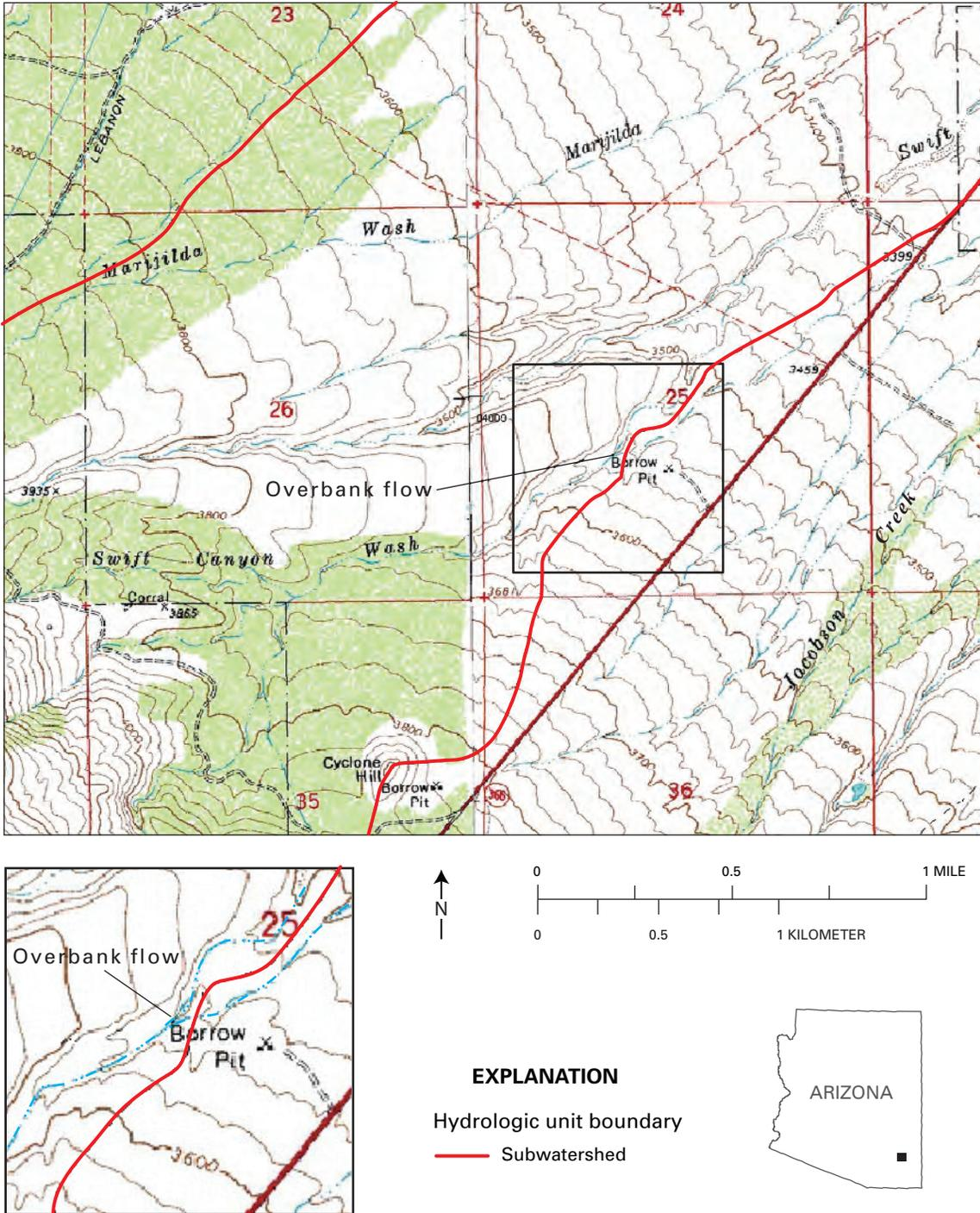
**Figure 18.** When high flows cause a natural diversion and the excess runs into an adjacent channel draining to a different hydrologic unit, the special condition is named overbank flow. Overbank flow is usually found in areas of alluvial material, such as in this area of Graham County, Arizona.
