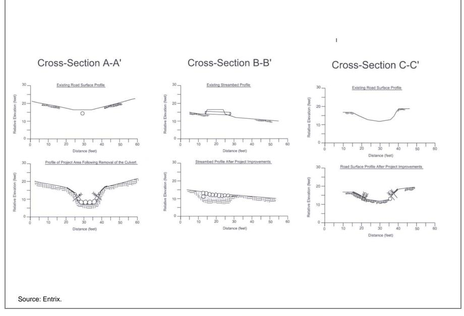
Figure 2-23. Cross Sections of Culvert Removal Project
