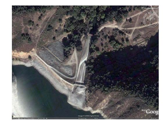
Figure 2. Google Earth image of the Los Padres Dam spillway, probably in 2007. Juvenile steelhead and kelts have to pass down the long concrete ramp in shallow water.
