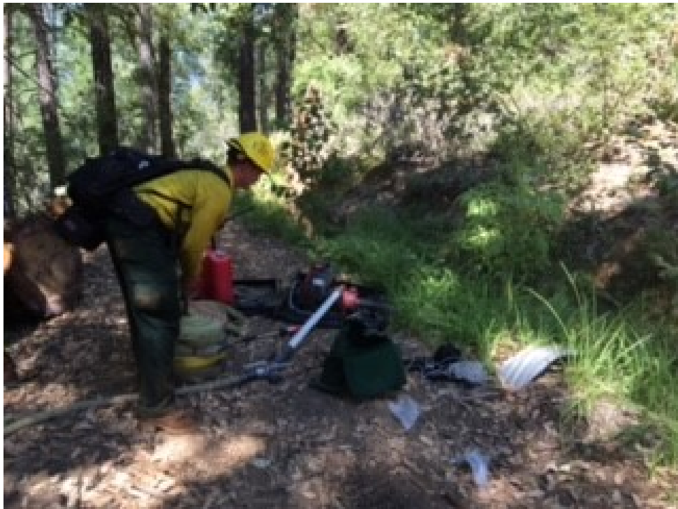
Exhibit MMR-10 Photograph #3 Forest Service Firefighter monitoring a pump that is pumping water from the diversion to fill fire engines.
