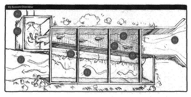
The Farmers Screen™ fish screen has several components that work together to create the hydraulic conditions necessary for both fish protection and debris management without the need for a mechanical cleaning mechanism. These system components work in harmony to create consistent hydraulic conditions to effectively manage debris and protect fish.
