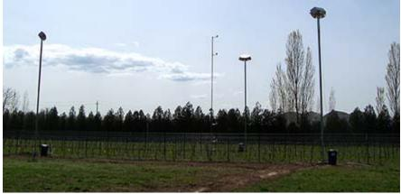
Vineland, Ontario -- A prototype system using low-level microwave radiant heat to prevent freezing and frost damage to vineyards and orchards is now being tested in Ontario. The new system trademarked as Tempwave was developed by the Raytheon Co., and installed in early April at the Vineland Research and Innovation Centre in Vineland.
