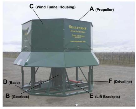
iron housing, aluminum caps, carburized and case hardened gears.
