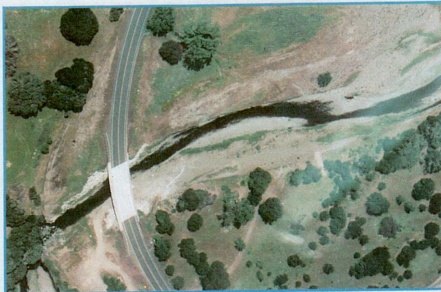
May 8, 1992. Note lone bush upper right center. River removed bush by 1995. Channel is wide and shallow.
