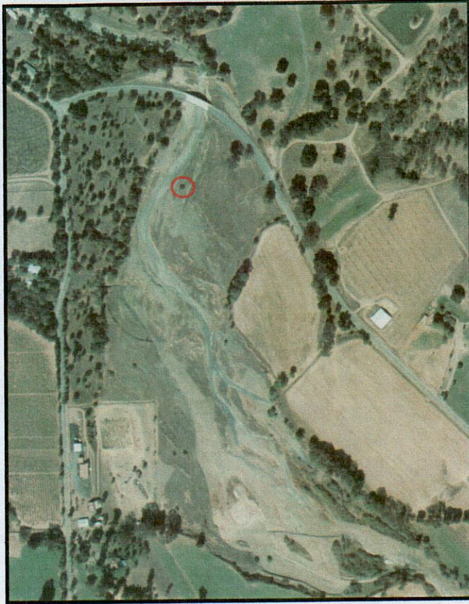
October 7, 1992, after new bridge. Bush is still present, and river course is more or less the same as before bridge construction but is beginning to shift to the east just below the bridge. It has not yet begun to move to the southwest downstream from the bush.
