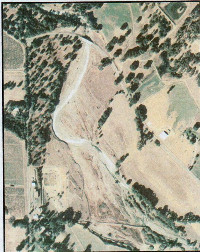
October 18, 1995. The river channel has changed markedly, the bush was lost to erosion, and the river has swung far to the southwest forcing it to make a sharp left turn. Serious erosion is taking place there and the channel is now fixed in place.
