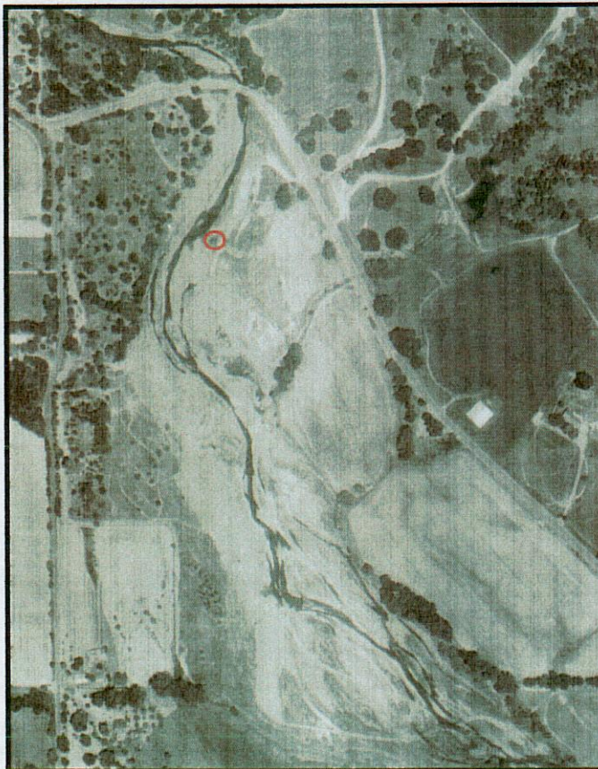
April 1988, before new bridge. Course of the river is gently curved and the stream is braided. The channel is not well defined but shows no tendency to move to the southwest.
