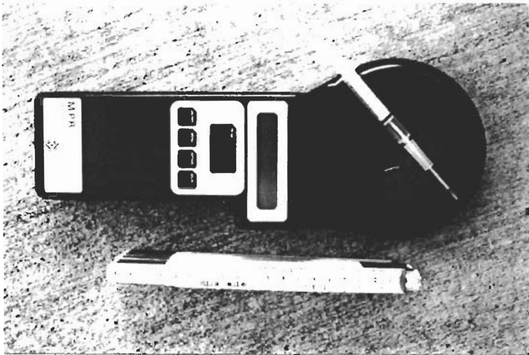
Photo 10. The PIT tagging equipment, including the reader, injector with needle and a PIT tag. A folding meter stick is provided for scale.
