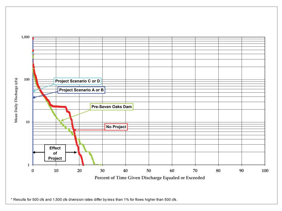
Figure 6.2-9. Probability of Daily Discharge (Non-Storm Days) for SAR Segment C, below Cuttle Weir\* WY 1966-67 through YW 1999-2000
