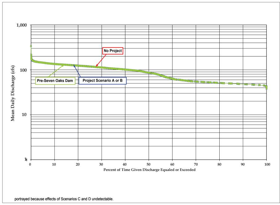
Figure 6.2-13. Probability of Daily Discharge (Non-Storm Days) for SAR Segment G, below Riverside Narrows, WY 1966-67 through YW 1999-2000
