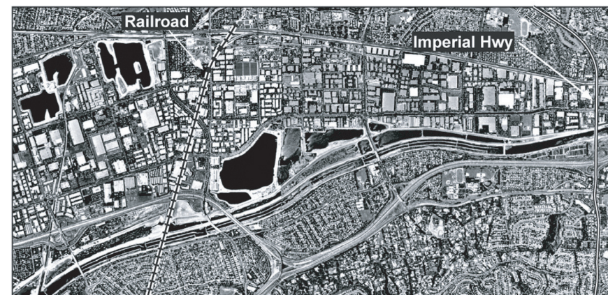
2002 Similar to existing condition with in-river and off-river recharge facilities. Well defined side levees. Well defined in-river "T and L" levees.
