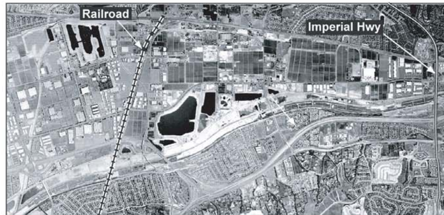
1977 Off-river recharge system paralleling main river channel is apparent. River channel is groomed with "T and L" levees. Miller Basin, Anaheim Lake, Warner Basin, Conrock Basin, Huckberry Pond are clearly visible.
