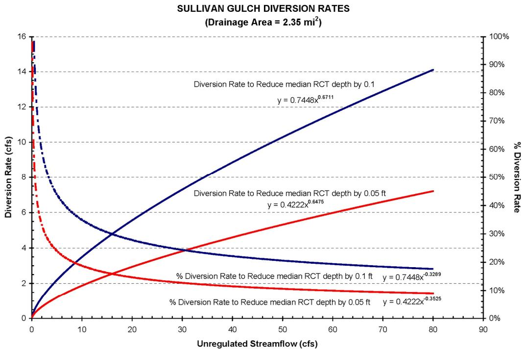
Figure 11. Fixed diversion rates as a function of unregulated streamflows for Sullivan Gulch at 0.10 ft and 0.05 ft diversion rates.
