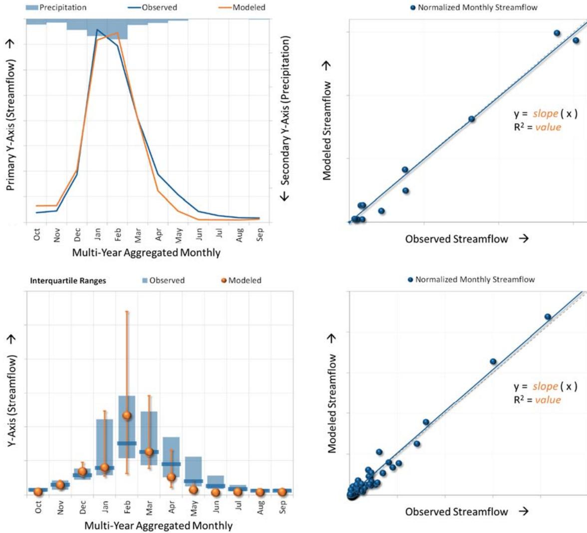
Figure 3-22. Example seasonal average and interquartile modeled versus observed streamflow (not based on the Shasta Basin).
