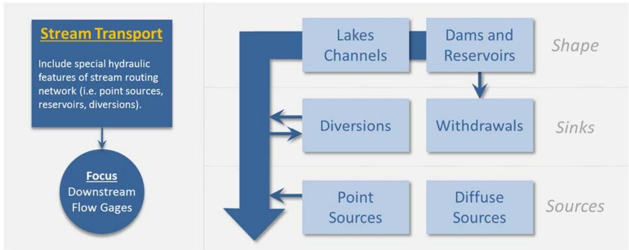
Figure 3-18. Model parameterization and calibration sequence for waterbodies and stream transport.
