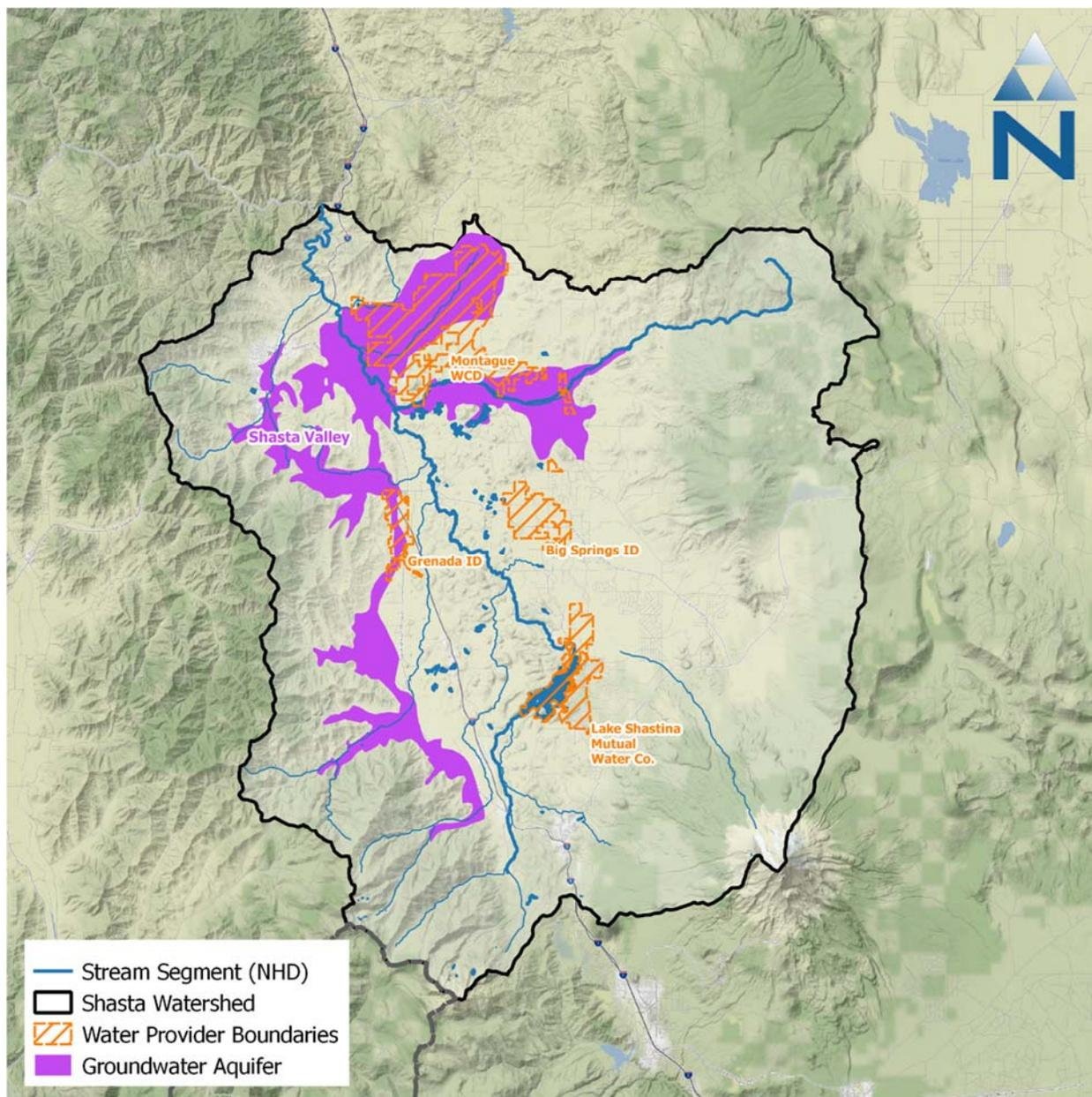
Figure 2-6. Alluvial aquifers recognized within the Shasta River watershed and water provider boundaries.
