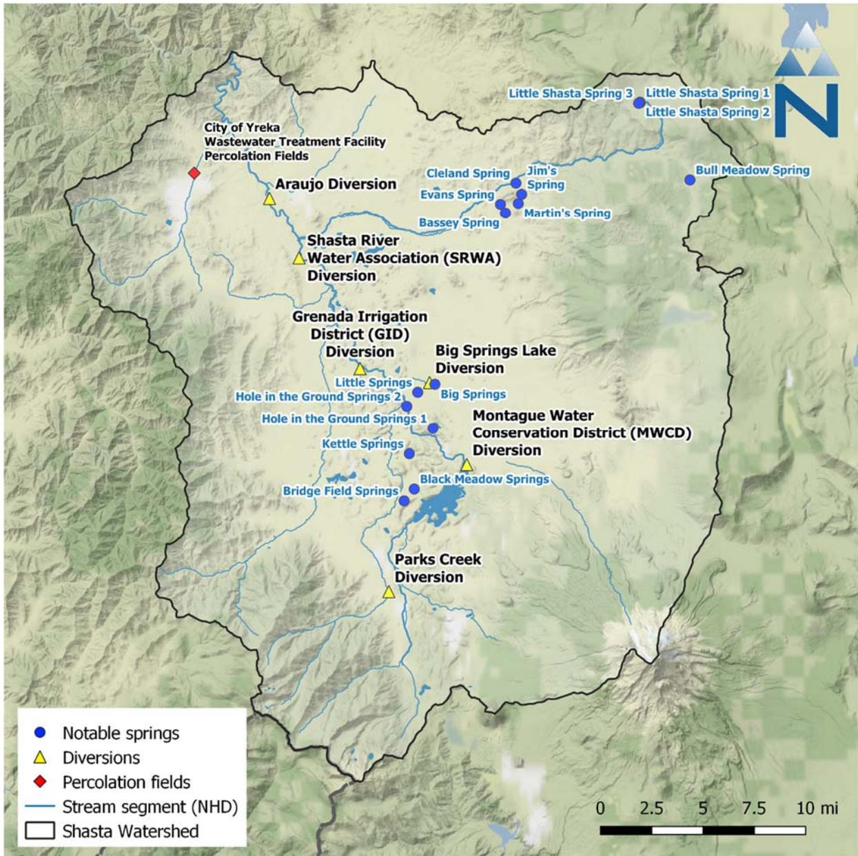
Figure 2-7. Notable groundwater springs, surface water diversions, and percolation fields in the Shasta Valley.
