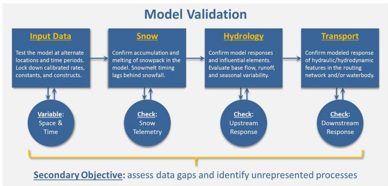
Figure 3-23. Process for model validation and identification of data gaps.
