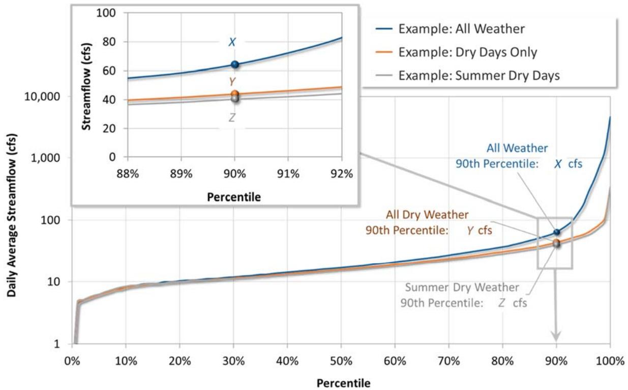
Figure 3-24. Example flow-duration curve analysis to define summer low-flow critical conditions (not based on the Shasta Basin).
