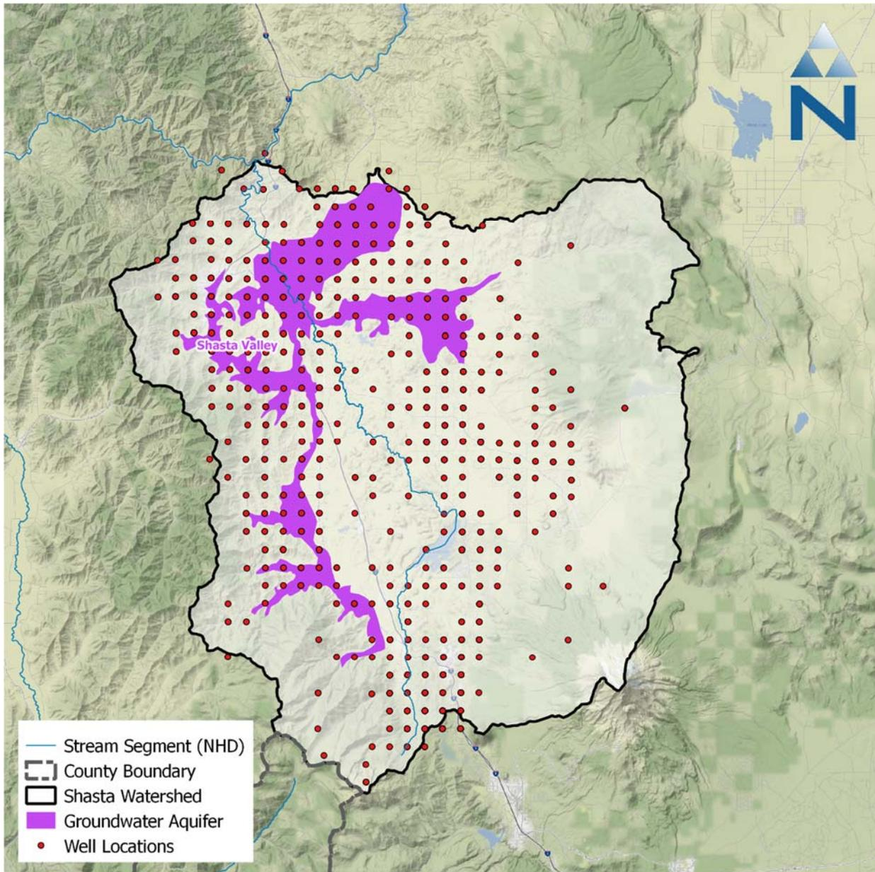
Figure 3-14. Estimated groundwater well locations in the Shasta River Watershed (1/8-mile location accuracy). Some red dots represent multiple wells within that area.
