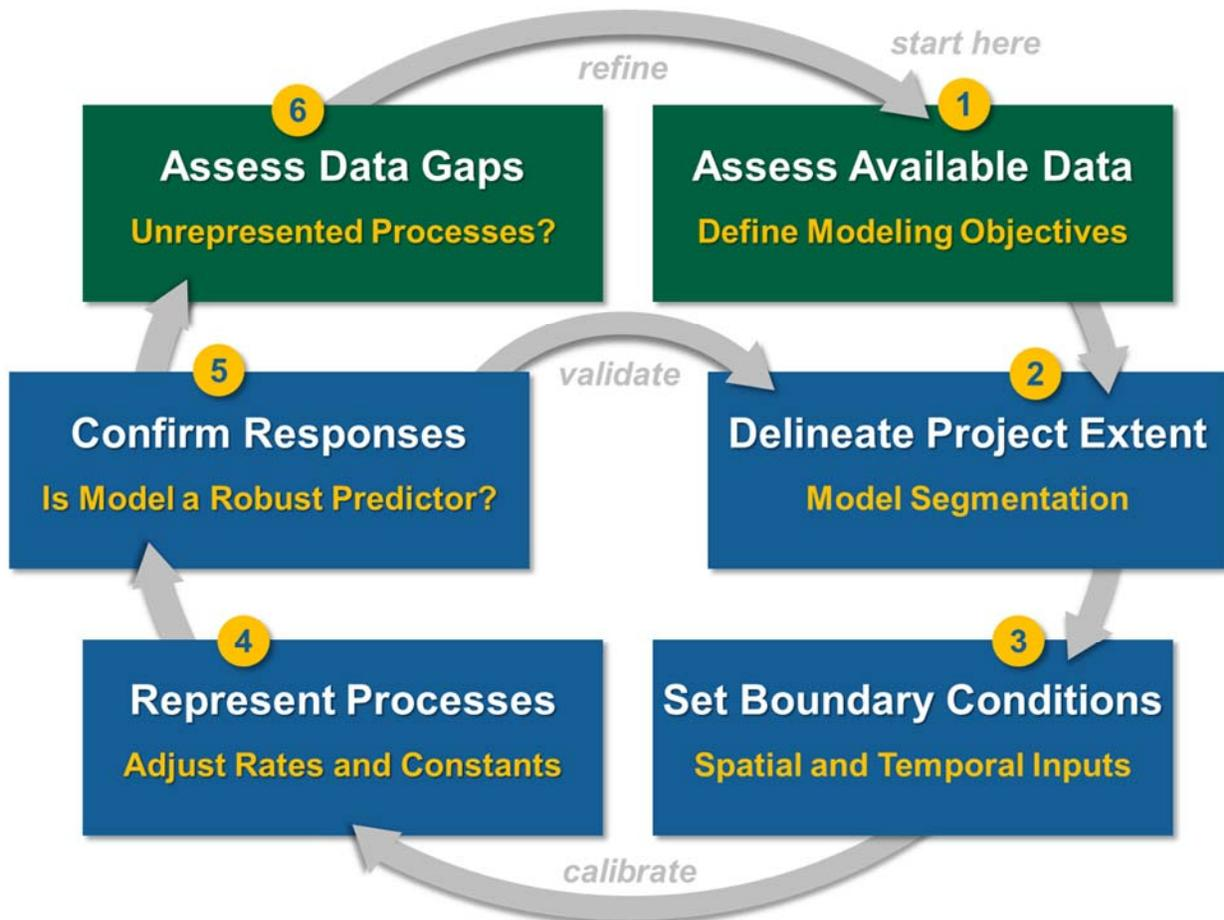
Figure 3-1. Conceptual schematic of a model development cycle.
