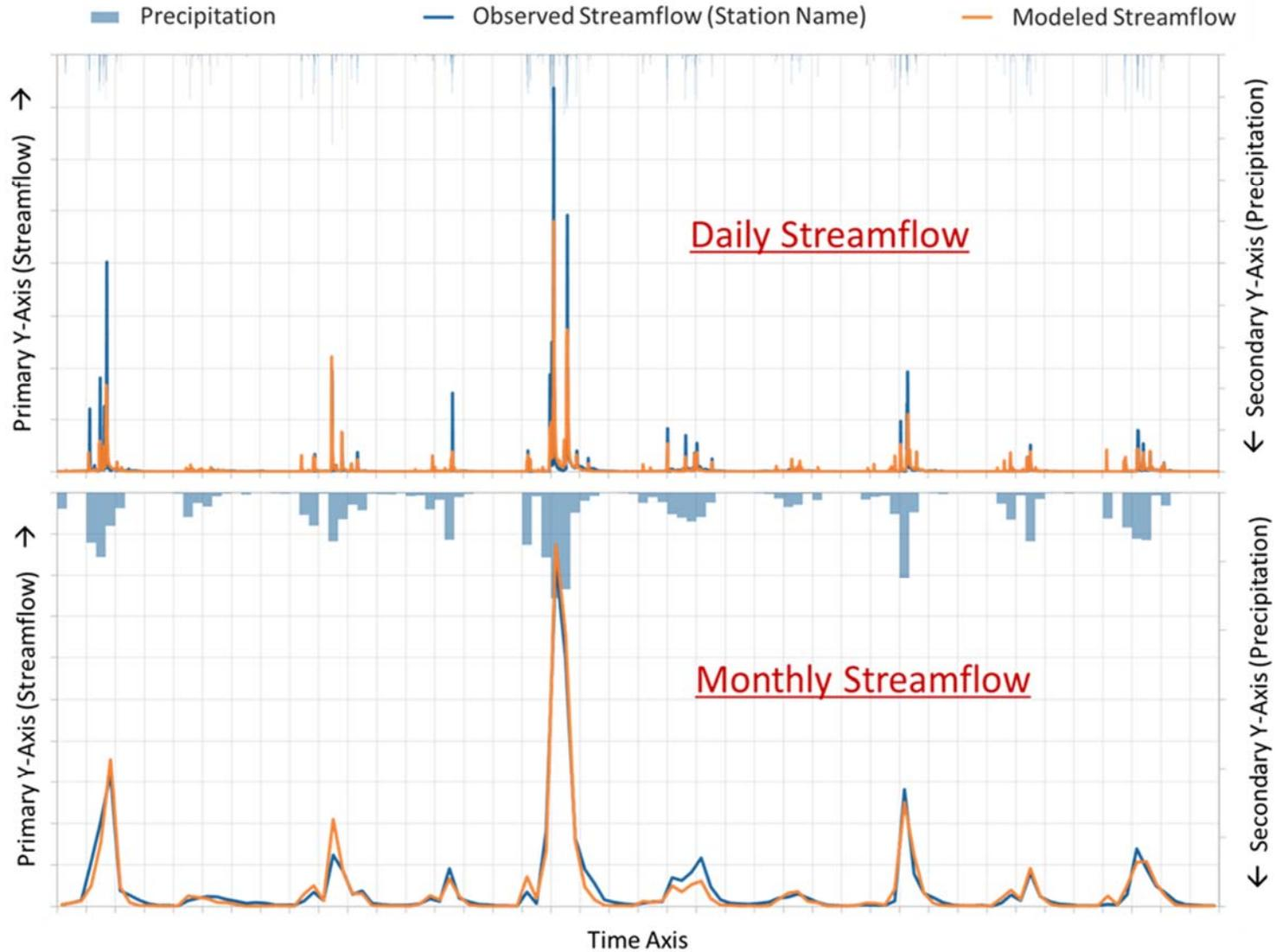
Figure 3-21. Examples of daily and monthly modeled versus observed streamflow (not based on the Shasta basin).
