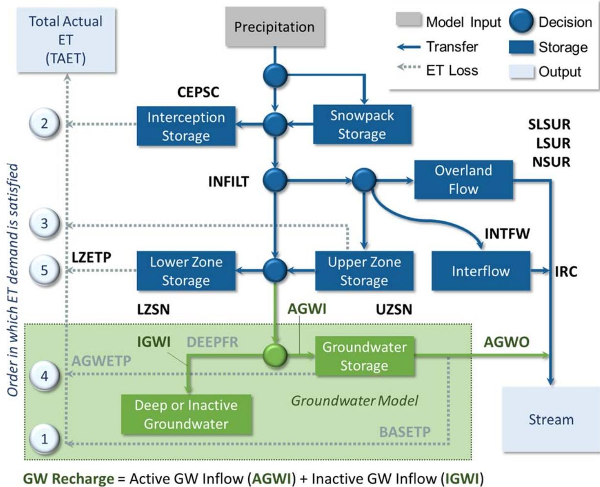
Figure 3-13. Conceptual linkage of a coupled groundwater model with HSPF.
