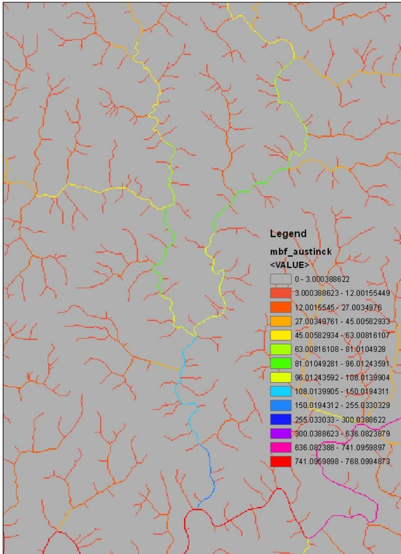
Figure 1: Estimated MBF (CFS) the Austin Creek network. Tributary channels in the box have MBF ~90 cfs each, while the confluent stream MBF ~140 cfs. Computations were carried out using information from the NHDplus and sampled information from the 13 gauged sites reported in the NCISFP documents.
