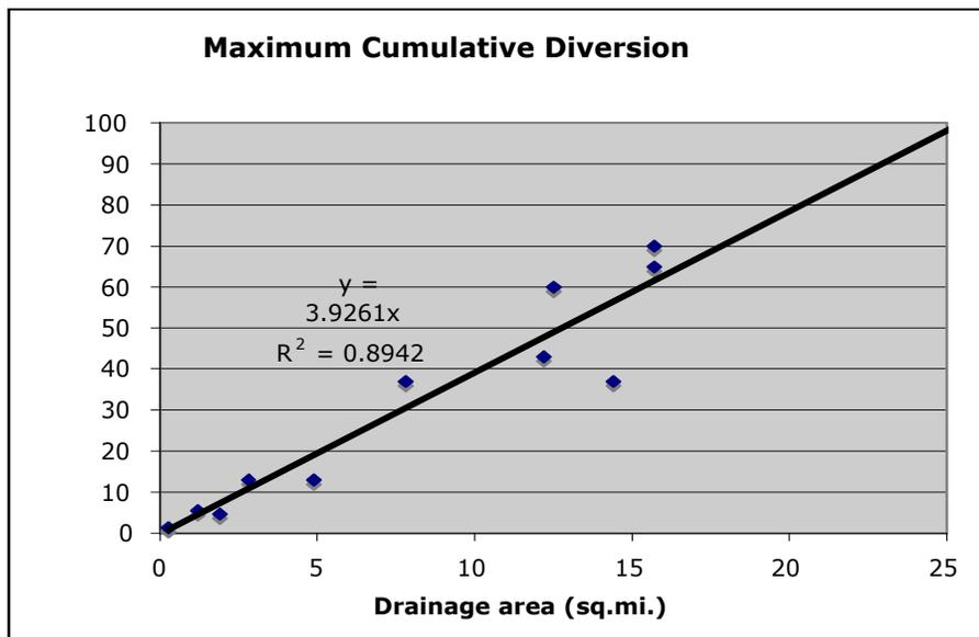
Figure 2: The maximum cumulative diversion rate based on the 5% of the 1.5 year flood extrapolated by drainage area from the sampled stream sites.
