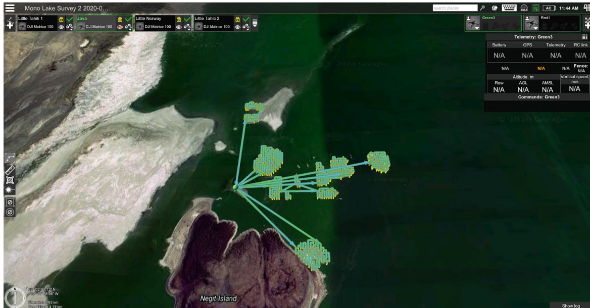
Figure 4. Flight planning routes and coverage of the Negit nesting islets from the base on Java used to acquire aerial imagery of gull nests and chicks.
