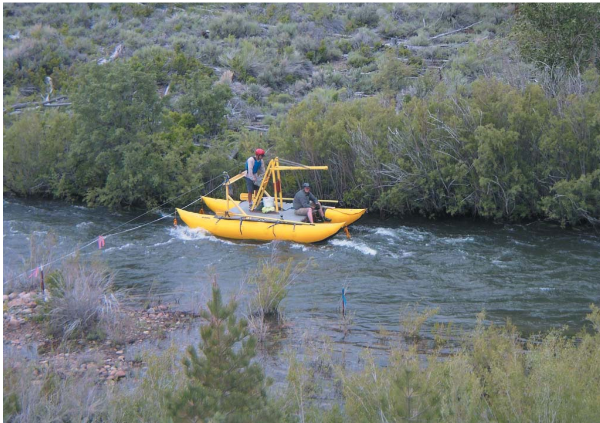
Figure 24a. Sediment sampling from the cataraft at the Upper Rush Creek site on June 25, 2005. The cataraft is attached to a cable that spans the channel, and is maneuvered between banks to collect sediment samples at discrete locations along the streambed and in the water column. One crew member operates a reel which raises and lowers the sampler; while the other crew member controls the sampler as it is lowered and raised through the water column. View is from the right bank, flow is from left to right and is approximately 400 cfs.
