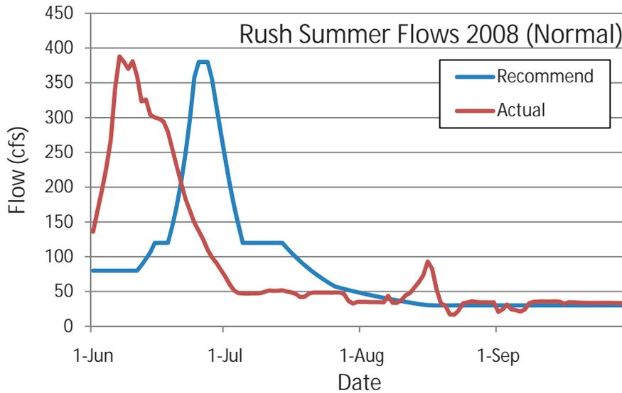
Figure D-4.16. Comparison of recommended flows (Recommended) and actual flows released down upper Rush Creek (Actual) during 2008. The short-duration increase and decline in “Actual” flows during mid-August represents test-flow releases for the instream flow study and usually D-1631 baseflows are held near 44 cfs throughout this period.
