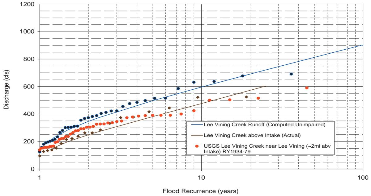
Appendix A-4. Figure 3. Lee Vining Creek above Intake (actual) and Lee Vining Creek Runoff (computed unimpaired) flood frequency analysis for Runoff Years 1973-2008.
