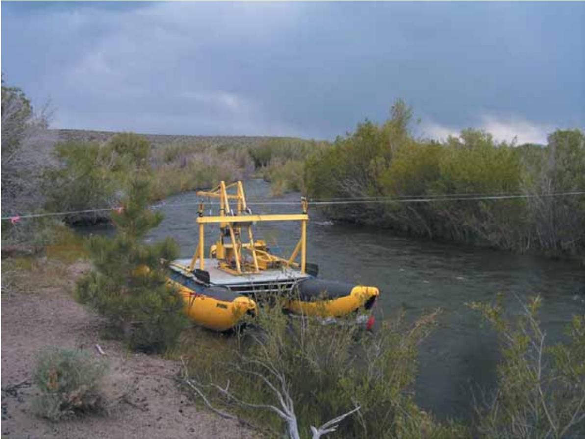
*Figure 24b. Cataraft set-up at the Lower Rush Creek site, June 25, 2005. Bank configuration on the left channel margin and vegetation along the right channel margin prevented the reel-operated samplers (TR-2 and D-74) to be used along the edges, so sampling along both channel edges was performed with hand-held samplers (3-inch Helley-Smith and DH-48). View is from the left bank, flow is from lower right and is approximately 465 cfs.*
