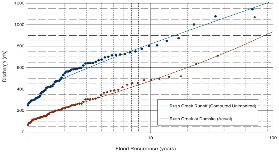
Appendix A-4. Figure 1. Rush Creek at Damsite (actual) and Rush Creek Runoff (computed unimpaired) flood frequency analysis for Runoff Years 1941-2008.
