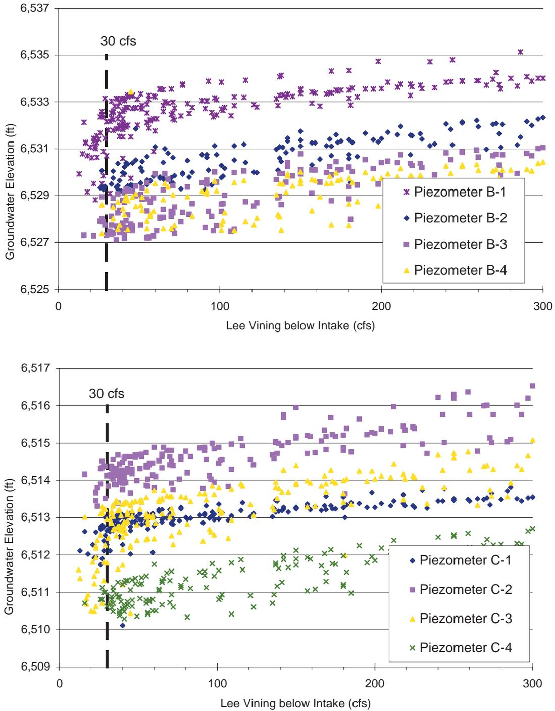
Figure C-22. Figure 4-8. Groundwater elevations at Lee Vining Creek piezometers B 1-4 and C 1-4 collected by the Mono Lake Committee for RYs 1995 to 2009.
