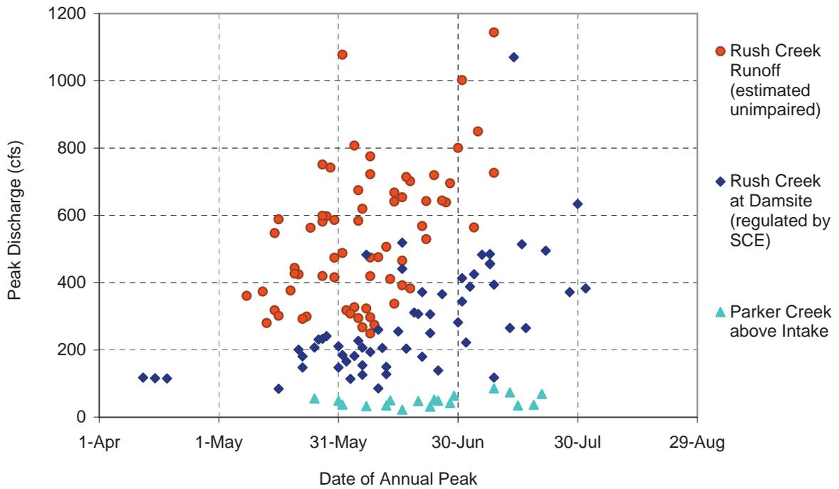
Appendix A-3. Figure 1. Timing and magnitude of peak flows for Rush Creek Runoff (estimated unimpaired), Rush Creek at Damsite (regulated by SCE), and Parker Creek above Intake (unimpaired).
