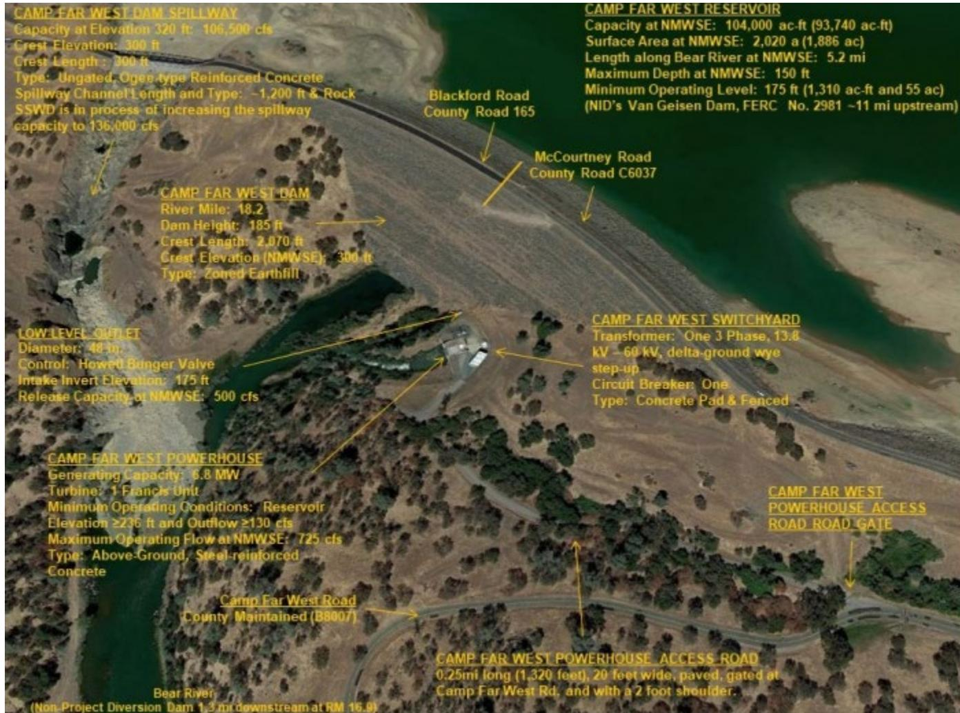
Figure A4. Camp Far West Hydroelectric Project Main Features (SSWD 2019a)
