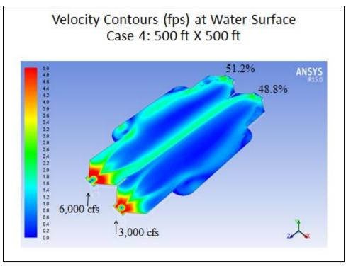
Figure 5-5: Intermediate Forebay CFD Case 4
