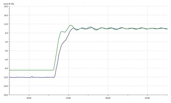
Figure 15 – HGL (ft) at STA 3150+70 Vent Shaft (located Upstream of the IF)
