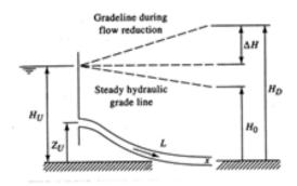
While the above represents a theoretical condition, in actuality - for the DHCCP system, the compression (i.e., pressure) wave traveling upstream does not bring the fluid to rest because there is an overflow relief at the surge shaft weirs and - as a result, the magnitude of the potential surge is lessened.
