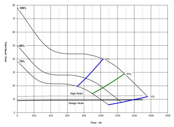
Figure 7-8: Pump and System Curves for 1 Large Variable Speed Pump Operating
