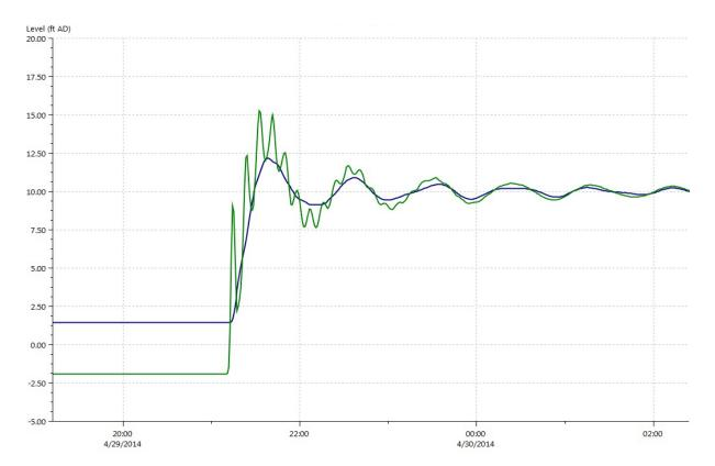
Figure 5 – HGL (ft) Upstream and Downstream of the IF; CELRAT = 76 Case Only
