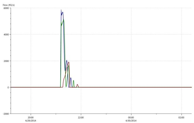
Figure 4 – Flow (cfs) in the Surge Bypass Channel
