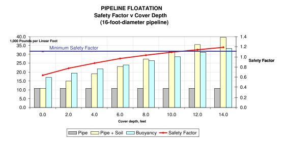
Figure 2: Concrete Pipe – Depth of Cover (16-foot-diameter)
