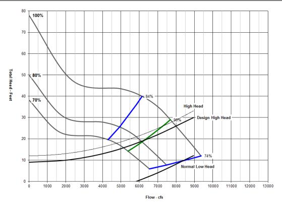
Figure 7-6: Pump and System Curves for 6 Large Variable Speed Pumps Operating
