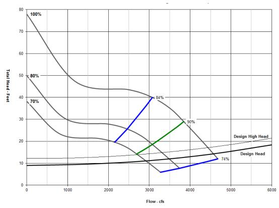
Figure 7-7: Pump and System Curves for 3 Large Variable Speed Pumps Operating
