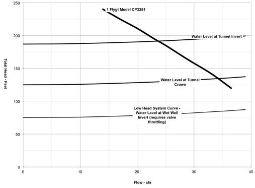
Figure 7-2: Dewatering Pump and System Curves – 1 Pump Operation (Flygt – Xylem Model CP 3351)
