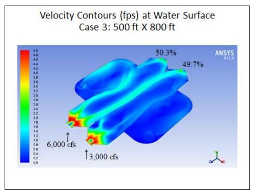
Figure 5-4: Intermediate Forebay CFD Case 3
