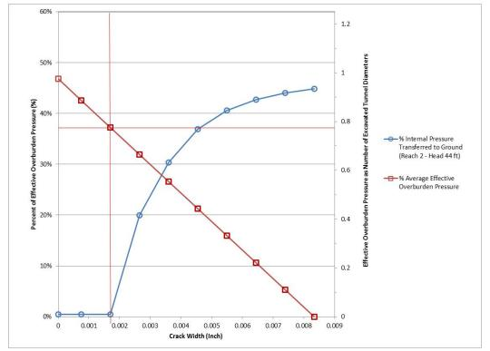
Figure 2: Reach 2 – Effective Overburden Pressure vs. Concrete Lining Crack Width
