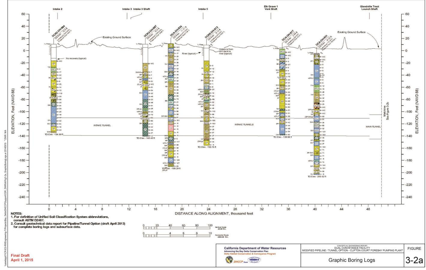
Figure 3-2: Graphic Boring Log, 1 of 5
