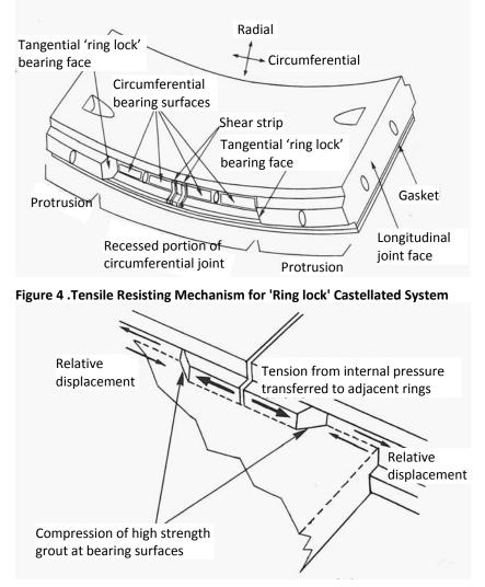
The ring acts to transfer the tension load into the adjacent rings via the bearing surfaces of the profiled joint. In principle, the mechanism is similar to the dowels, except that the compression of the concrete provides a much stiffer resistance.
