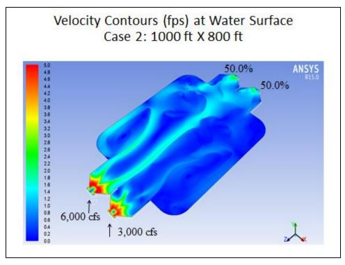
Figure 5-3: Intermediate Forebay CFD Case 2
