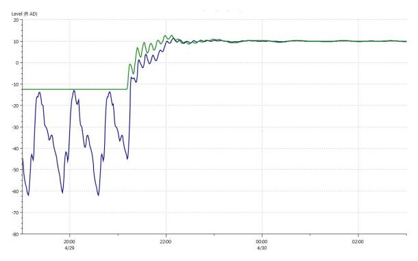
Figure 16 – HGL (ft) at Staten Island Vent Shaft (located Downstream of the IF)
