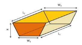
Known: Elevation, height, slope, Length L1, Width W1 Unknown: Length L2, Width W2
