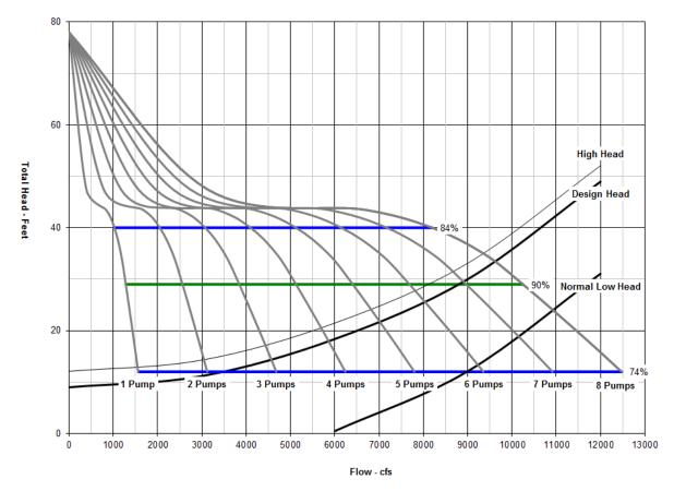
Figure 7-4: Pump and System Curves for 1 to 8 Large Constant Speed Pumps
