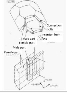
Machined steel pieces that fit together on insertion to provide a tight fit. They were originally conceived as part of hybrid segments comprising all-round steel structure with concrete infill. However, they could be employed in conventional reinforced concrete segments. Careful detailing could ensure that the required tensile capacity is provided with minimal impact on joint bearing surface, so the ability of the lining to take compression loads would not be compromised.
