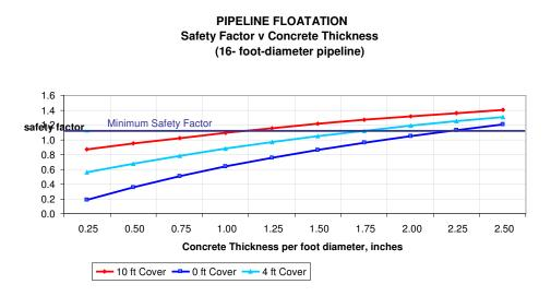
Figure 3: Concrete Pipe – Pipeline Wall Thickness
