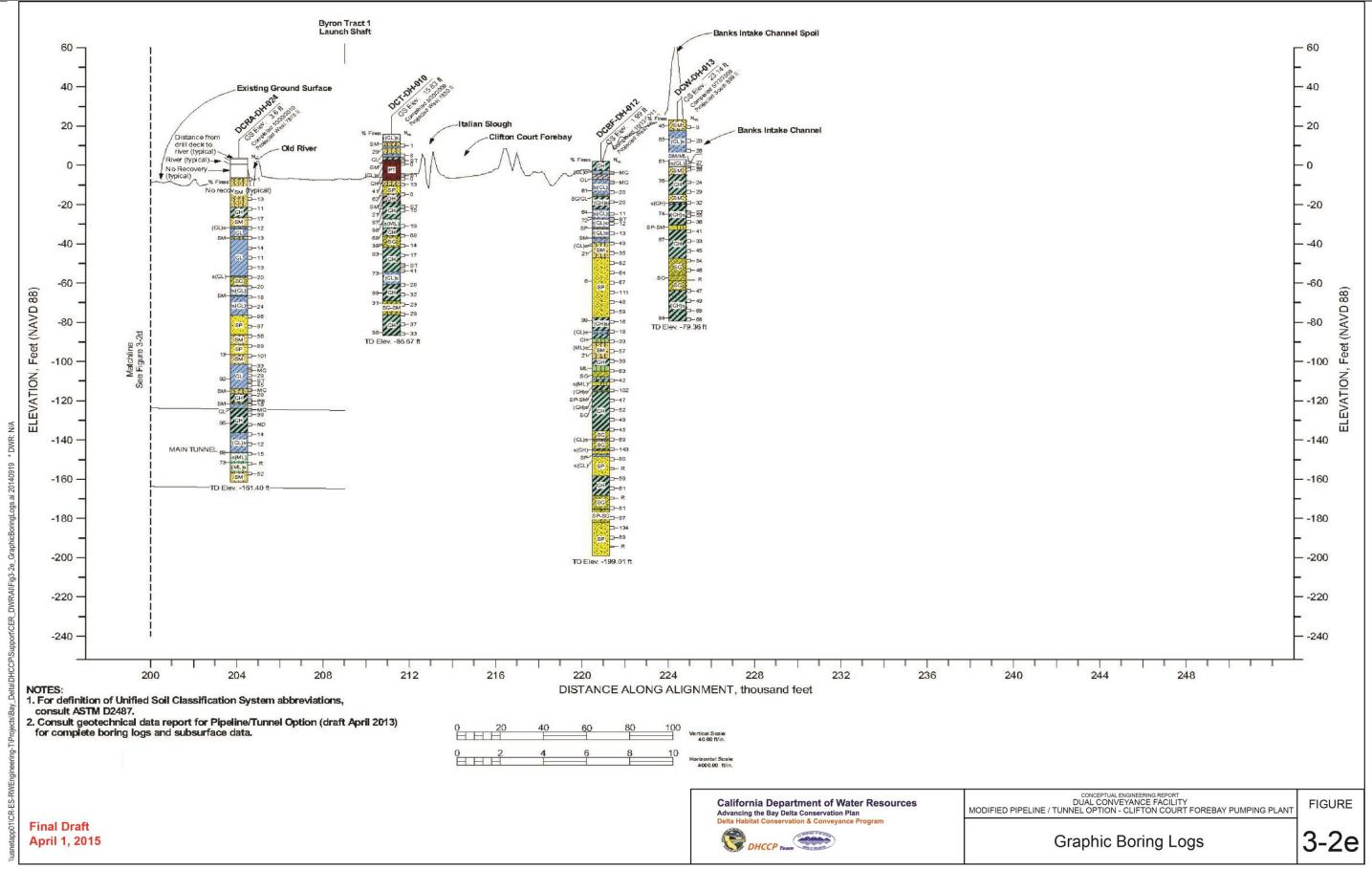
Figure 3-6: Graphic Boring Logs, 5 of 5
