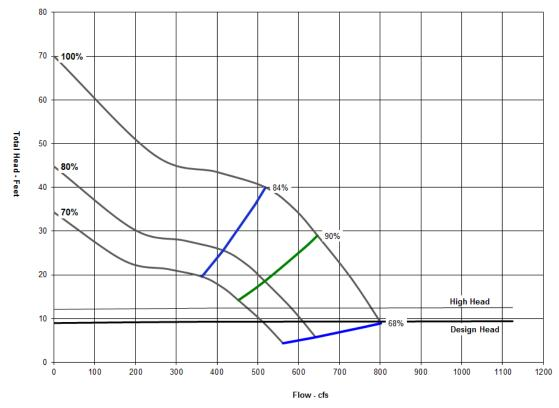
Figure 7-9: Pump and System Curves for 1 Small Variable Speed Pump Operating
