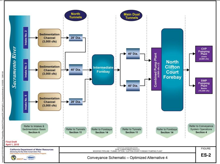
*Figure ES- 2: Conveyance Schematic*
