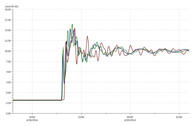
Figure 1 – HGL (ft) at the Staten Island Vent Shaft (located downstream of the IF)
