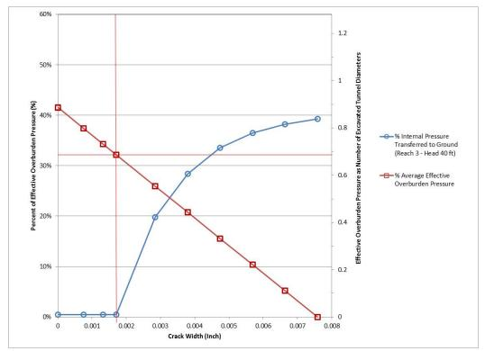
Figure 3: Reach 3 – Effective Overburden Pressure vs. Concrete Lining Crack Width
