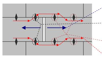
Figure 1. Dowels resisting tension: conventional 3 dowel arrangement
