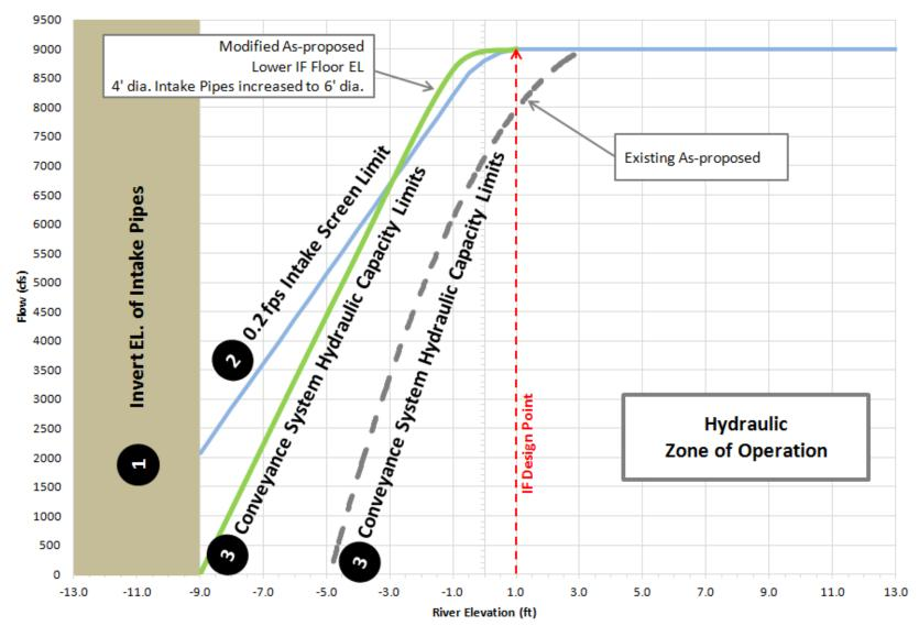
Figure 3 – As-Proposed Hydraulic Conveyance System Capacity Curve
