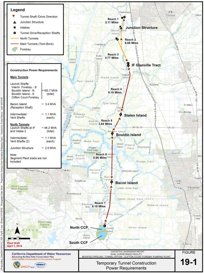
Figure 19-1: **Tunnel Construction Power Requirements**
