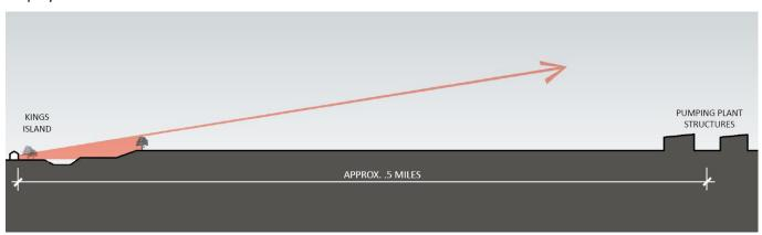
Figure 27-8: Site Section. Increase in berm height and plantings buffer view of King's Island residents from tall pump plants.
