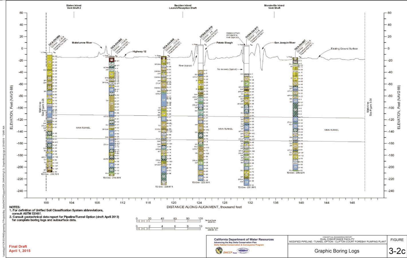
Figure 3-4: Graphic Boring Logs, 3 of 5
