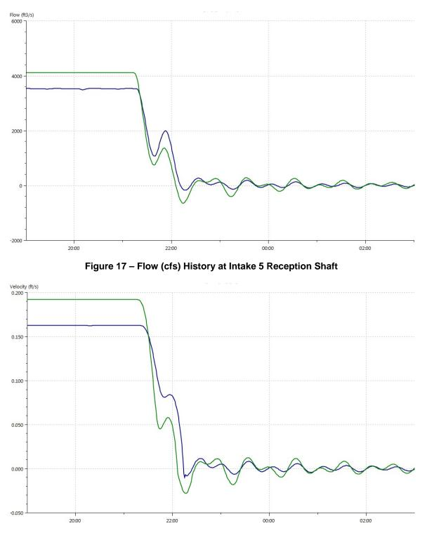
Figure 18 – Velocity (fps) History in an Intake 5 Sediment Basin
