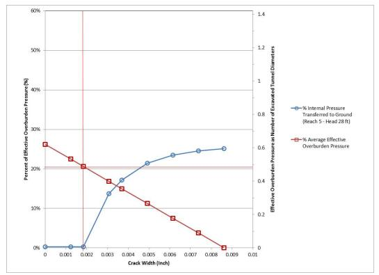
Figure 5: Reach 5 - Effective Overburden Pressure vs. Concrete Lining Crack Width
