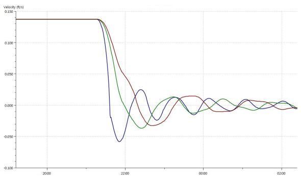
Figure 12 – Velocity (fps) History in an Intake 5 Sediment Basin
