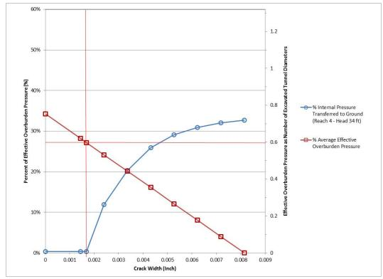
Figure 4: Reach 4 – Effective Overburden Pressure vs. Concrete Lining Crack Width
