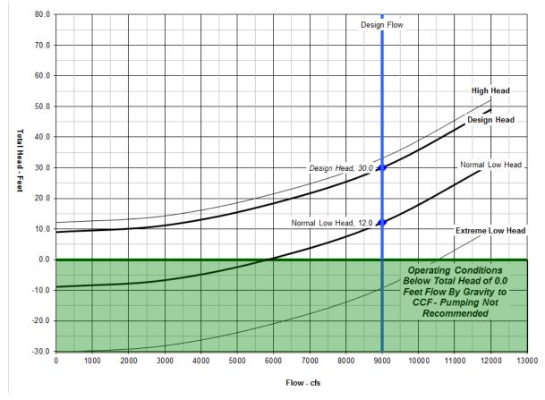
Figure 7-3: System Curves for the Range of Operating Conditions
