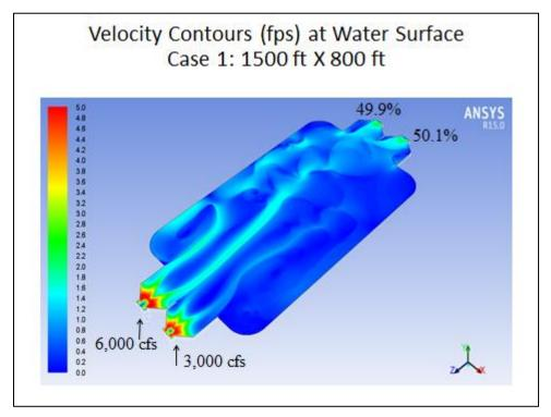
Figure 5-2: Intermediate Forebay CFD Case 1
