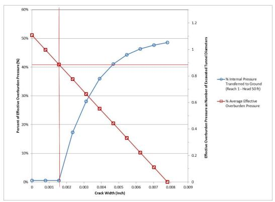
Figure 1: Reach 1 – Effective Overburden Pressure vs. Concrete Lining Crack Width
