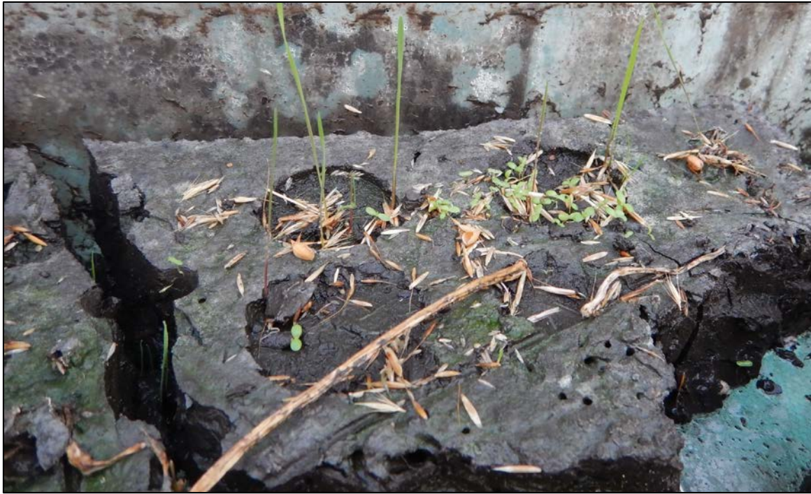
Plant growth is visible in cracks and the round Torvane scars.
